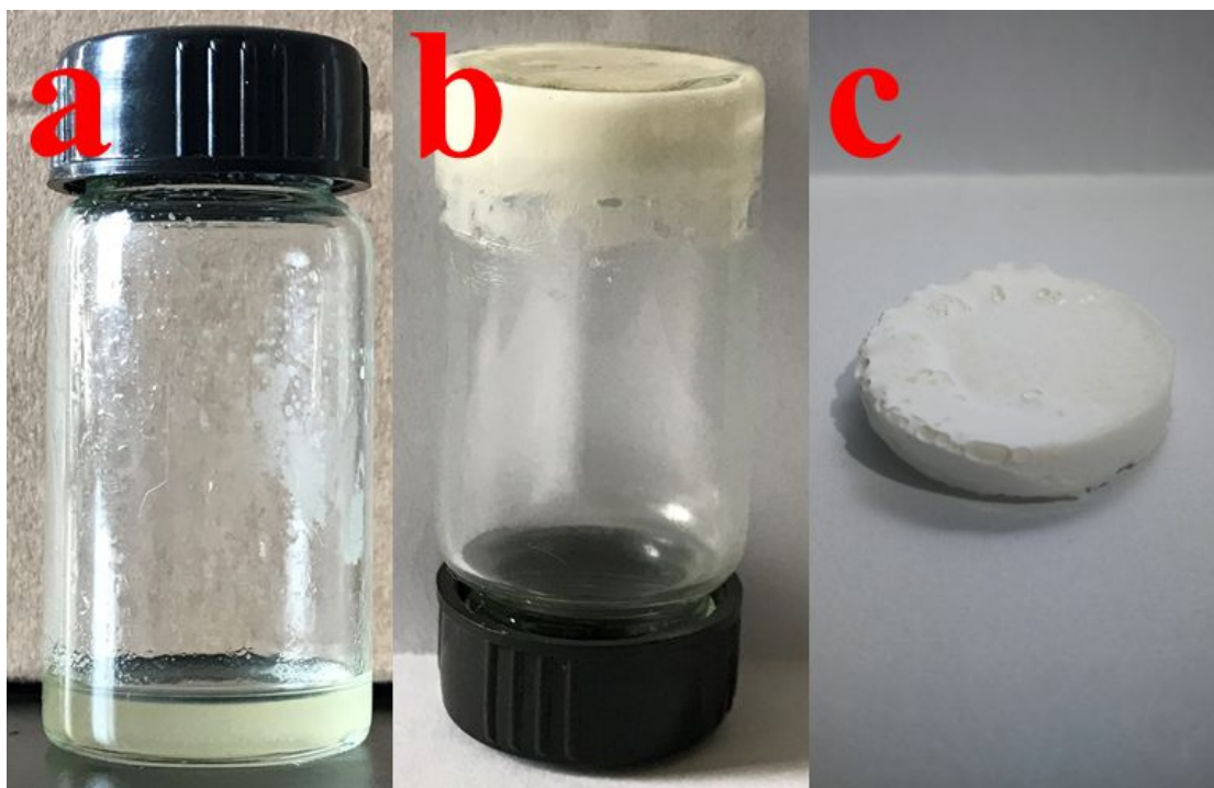
Figure S3. typical photographs of forming PLLA-based polyHIPE, continuous phase solution (a), HIPE (b) and PLLA-based polyHIPE (c).
