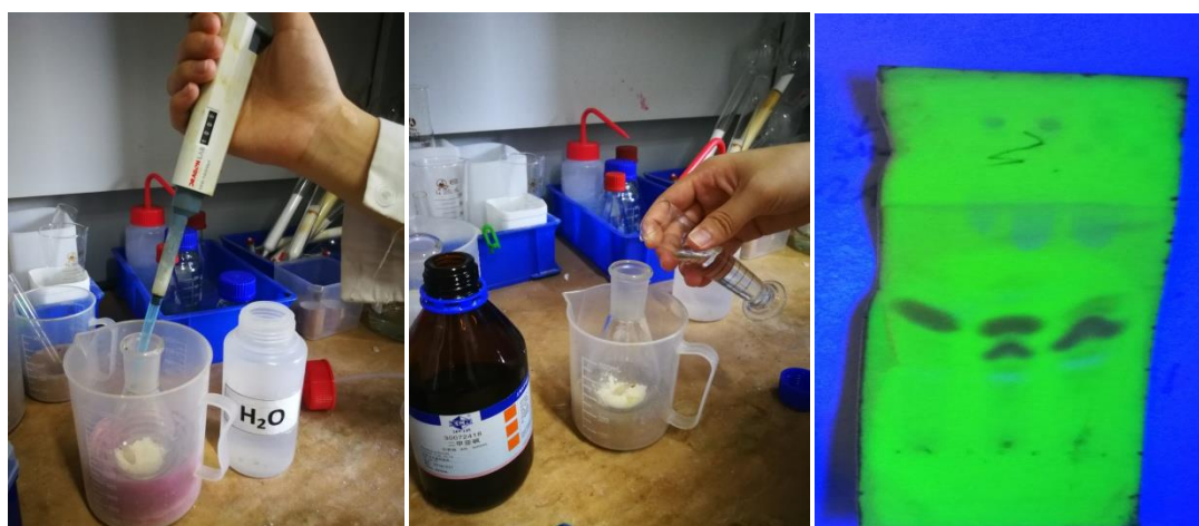
(Left) Addition of \text{H}_2\text{O} (1.4 mL, 80 mmol); (Center) Dissolved in DMSO (25 mL); (Right) TLC under UV (PE/EtOAc = 2:1).
