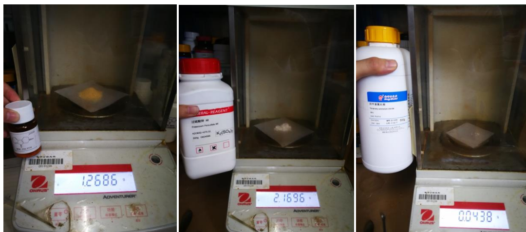
(Left) 1 (1.26 g, 4 mmol); (Center) \text{Na}_2\text{S}_2\text{O}_8 (2.16 g, 8 mmol); (Right) \text{Me}_4\text{NCl} (43 mg, 0.4 mmol).
