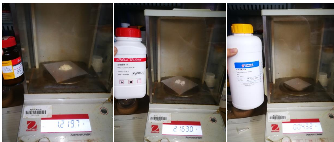
(Left) Evodiamine (1.21 g, 4 mmol); (Center) \text{Na}_2\text{S}_2\text{O}_8 (2.16 g, 8 mmol); (Right) \text{Me}_4\text{NCl} (43 mg, 0.4 mmol).
