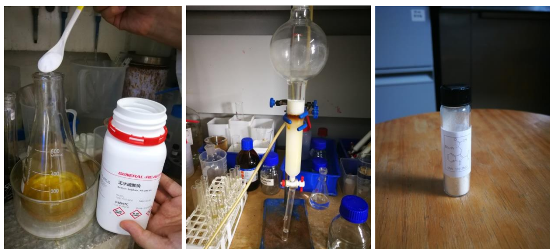
(Left) dried with \text{Na}_2\text{SO}_4 ; (Center) Purified by chromatography on silica gel (PE/EtOAc = 2:1); (Right) Product after column chromatography.
