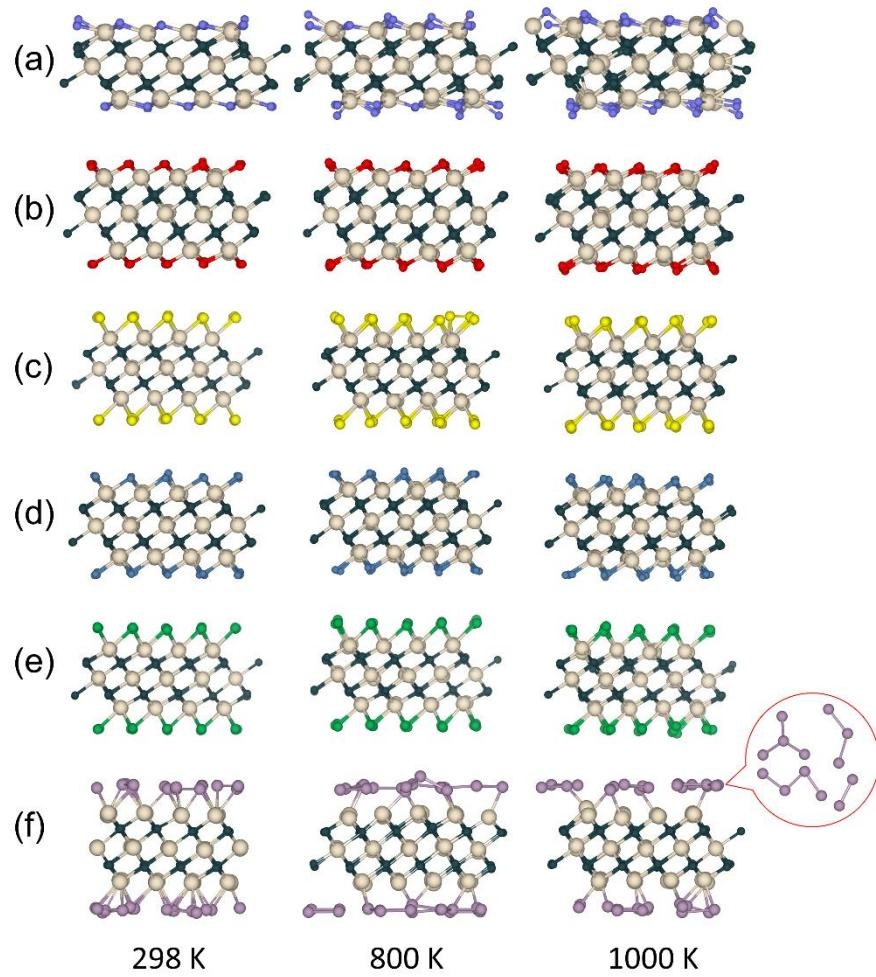
**Fig. S2** Snapshots of the equilibrium structure of (a)  $\text{Ti}_3\text{C}_2\text{N}_2$ , (b)  $\text{Ti}_3\text{C}_2\text{O}_2$ , (c)  $\text{Ti}_3\text{C}_2\text{S}_2$ , (d)  $\text{Ti}_3\text{C}_2\text{F}_2$ , (e)  $\text{Ti}_3\text{C}_2\text{Cl}_2$  and (f)  $\text{Ti}_3\text{C}_2\text{P}_2$  after 5 ps AIMD simulation.
