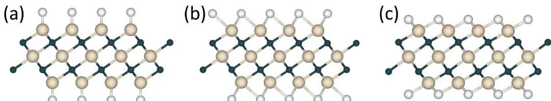
**Fig. S1** Three possible configurations for  $\text{Ti}_3\text{C}_2\text{T}_2$  (a) Mode I, (b) Mode II, (c) Mode III with different functional group positions. White balls are functional groups T.
