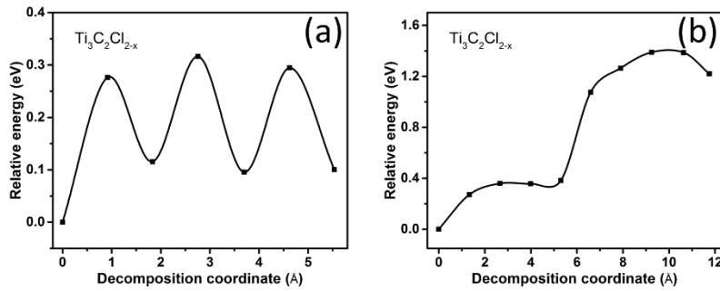
**Fig. S9** Energy profiles for the decomposition of (a)  $\text{Li}_2\text{S}$  and (b)  $\text{Li}_2\text{S}_6$  on  $\text{Ti}_3\text{C}_2\text{Cl}_{2-x}$ , respectively.
