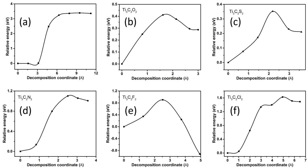
**Fig. S6** Energy profiles for the decomposition of  $\text{Li}_2\text{S}$  in (a) vacuum and on (b-f)  $\text{Ti}_3\text{C}_2\text{T}_2$  ( $\text{T} = \text{O}, \text{S}, \text{N}, \text{F}, \text{Cl}$ ),
