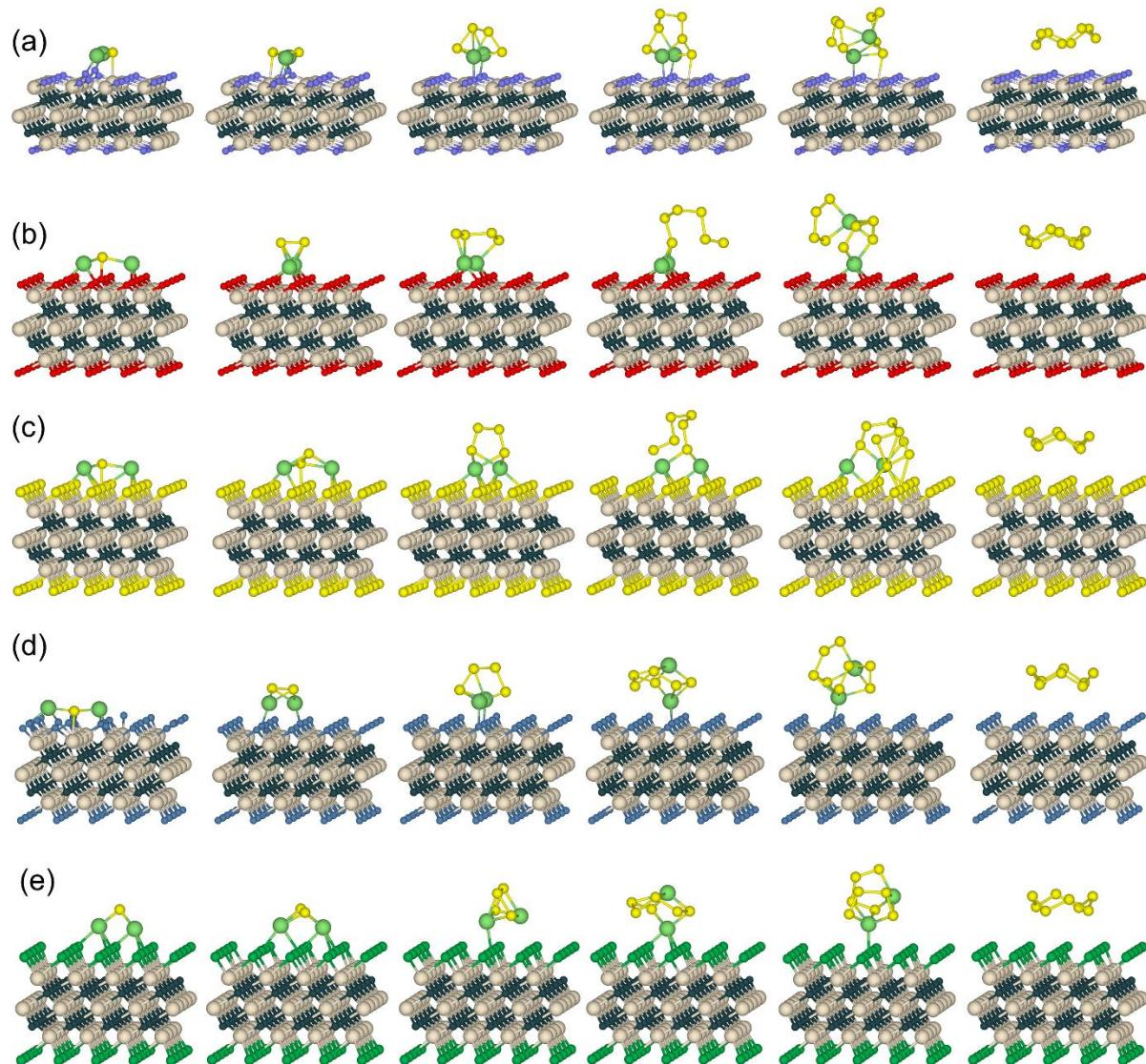
**Fig. S4** Adsorption configurations of  $\text{Li}_2\text{S}_n$  and  $\text{S}_8$  on the surface of (a)  $\text{Ti}_3\text{C}_2\text{N}_2$ , (b)  $\text{Ti}_3\text{C}_2\text{O}_2$ , (c)  $\text{Ti}_3\text{C}_2\text{S}_2$ , (d)  $\text{Ti}_3\text{C}_2\text{F}_2$  and (e)  $\text{Ti}_3\text{C}_2\text{Cl}_2$ .
