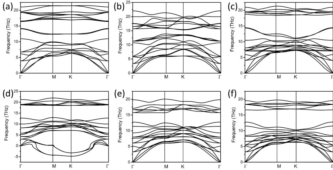
**Fig. S3** Calculated phonon dispersions along the high symmetrical directions of the Brillouin zone for (a)  $\text{Ti}_3\text{C}_2\text{N}_2$ , (b)  $\text{Ti}_3\text{C}_2\text{O}_2$ , (c)  $\text{Ti}_3\text{C}_2\text{F}_2$ , (d)  $\text{Ti}_3\text{C}_2\text{P}_2$ , (e)  $\text{Ti}_3\text{C}_2\text{S}_2$ , and (f)  $\text{Ti}_3\text{C}_2\text{Cl}_2$ .
