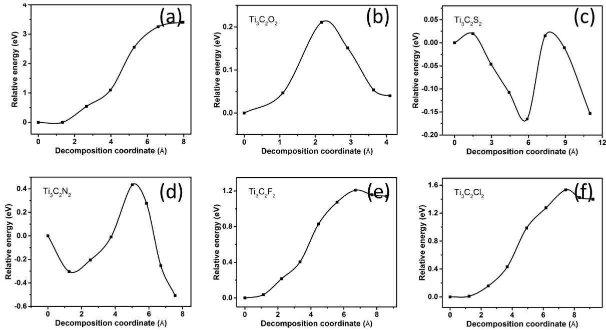
**Fig. S7** Energy profiles for the decomposition of  $\text{Li}_2\text{S}_6$  in (a) vacuum and on (b-f)  $\text{Ti}_3\text{C}_2\text{T}_2$  ( $\text{T} = \text{O}, \text{S}, \text{N}, \text{F}, \text{Cl}$ ), respectively.
