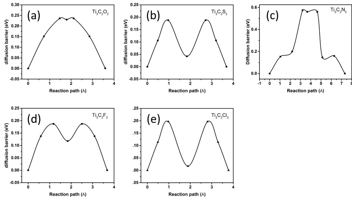
**Fig. S8** Energy profiles for  $\text{Li}^+$  diffusion on  $\text{Ti}_3\text{C}_2\text{T}_2$  ( $\text{T} = \text{O}, \text{S}, \text{N}, \text{F}, \text{Cl}$ ), respectively.
