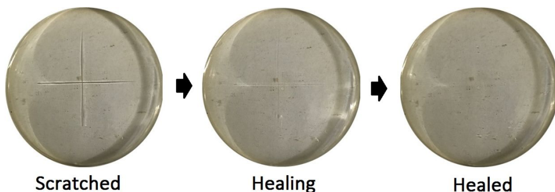
Figure S16. Photographs recording the self-healing process of PDMS-MPI-TM film at room temperature. As shown, a visible scratch could be autonomously restored after 4 h at room temperature without any assistance.
