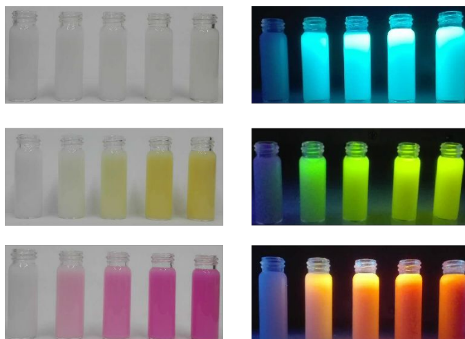
Figure S7. The photographs of methanol solution of C-151@ZIF-8 2 (top), F@ZIF-8 2 (middle) and RB@ZIF-8 2 (below) with different dye concentration under daylight (left) and UV light (right).
