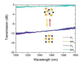
Figure S2. Measured transmission spectra of the device with 1-µm-diameter GST over two phase-change cycles.
