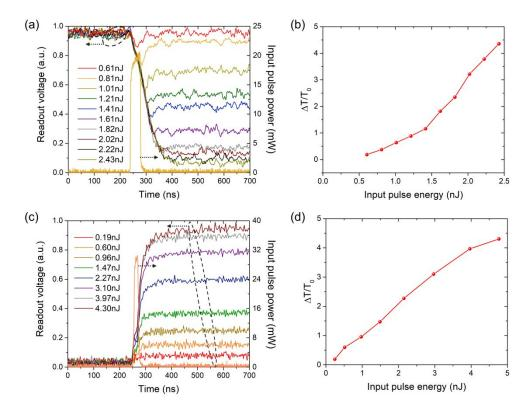
Figure S5 (a, b) Dynamic response of optical transmission during the crystallization process. (a) The input optical pulse has a fixed power and a varying duration. (b) The maximum transmission change varies with the pulse energy. (c, d) Dynamic response of optical transmission during the amorphization process. (c) The input optical pulse has a fixed duration and a varying power. (d) The maximum transmission change varies with the pulse energy.
