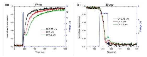
Figure S3. Transmission dynamics during (a) the amorphization and (b) the crystallization processes. The excitation electrical pulse energy is high enough to initiate the phase transition for different sizes of GST.
