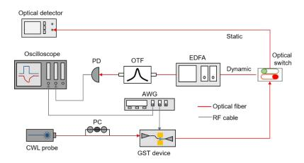
Figure S1. Experimental setup for device characterization. CWL: continuous-wave laser; PC: polarization controller; AWG: arbitrary waveform generator; EDFA: erbium-doped fiber amplifier; OTF: optical tunable filter; PD: photodiode.
