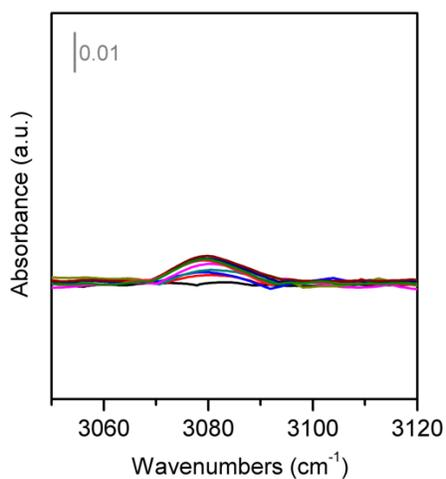
**Figure S10.** Peak between 3070 and 3100 cm<sup>-1</sup>. ATR-IR spectra were collected with 1-hexyne and 120 psi H<sub>2</sub> applied on Pd<sub>0.004</sub>Au-SAA catalysts in the batch mode at room temperature.
