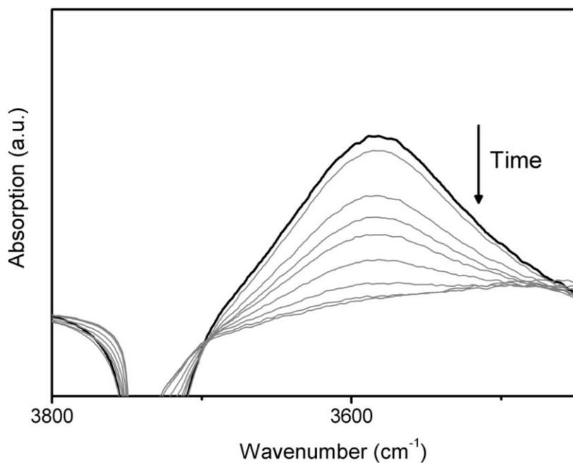
**Figure S8.** DRIFT spectra between 3800 and 3450 cm<sup>-1</sup> recorded when 1-hexyne and H<sub>2</sub> are carried over Pd<sub>0.004</sub>Au-SAA/SiO<sub>2</sub> at room temperature.
