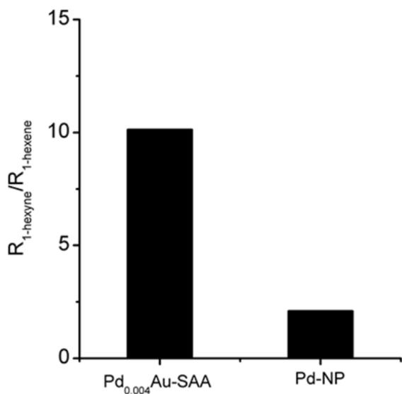
**Figure S13.** Ratio between the conversion rate of 1-hexyne and 1-hexene in hydrogenation reaction conditions. Reaction conditions: 1% hexyne-ethanol or hexene-ethanol solution, 5 bar H<sub>2</sub>, 25 °C.
