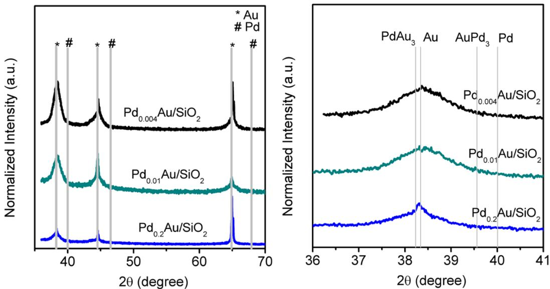
**Figure S1.** Powder XRD of PdAu samples with different Pd/Au ratios. The Pd<sub>0.004</sub>Au/SiO<sub>2</sub> is the single-atom alloy (SAA) sample investigated in this paper.
