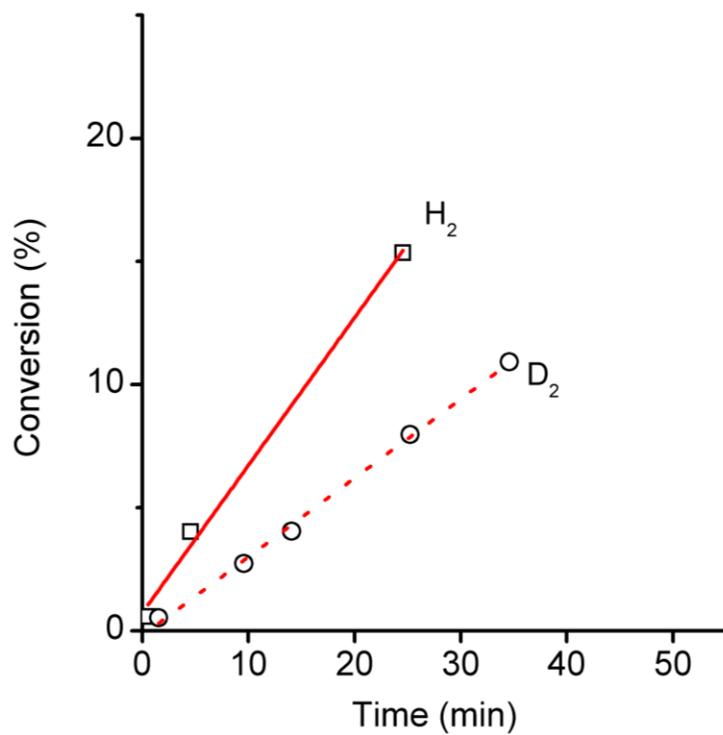
**Figure S4.** Kinetic Isotope Effect (KIE) measurements. Conversion vs. reaction time for 1-hexyne hydrogenation on Pd<sub>0.004</sub>Au/SiO<sub>2</sub> catalysts. The initial rate is calculated from the slope of the conversion-time curve. Reaction conditions: 1% hexyne-ethanol solution, 5 bar H<sub>2</sub> or D<sub>2</sub>, 600 rpm, 25 °C.
