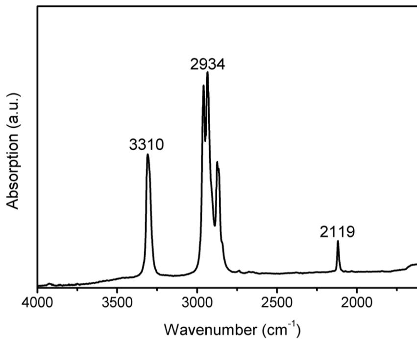
**Figure S7.** ATR-IR spectra of liquid 1-hexyne in ATR cell without catalyst.
