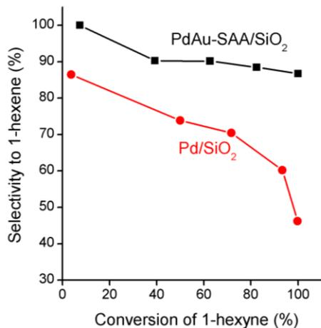
**Figure S12.** Time-resolved batch reactor data for the hydrogenation of 1-hexyne over Pd<sub>0.004</sub>Au - SAA catalysts vs Pd.
