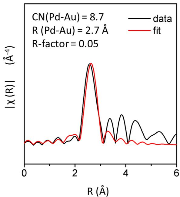
**Figure S3.** Fourier transform of EXAFS spectra of Pd K edge for the Pd<sub>0.004</sub>Au-SAA/SiO<sub>2</sub> and the EXAFS modeling fitting results.
