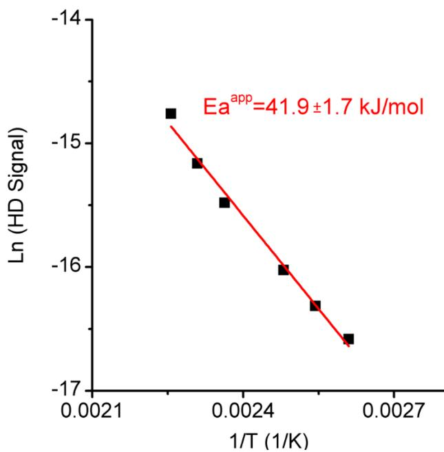
**Figure S5.** Arrhenius-type plot for H<sub>2</sub>-D<sub>2</sub> exchange over Pd<sub>0.004</sub>Au-SAA/SiO<sub>2</sub> catalyst.
