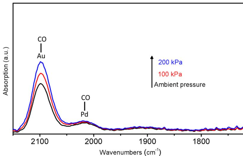
**Figure S2.** ATR-IR spectra of the CO stretch on unsupported Pd<sub>0.004</sub>Au-SAA samples. Spectra were collected at 30 °C with different CO partial pressure in the gas phase. The bridge adsorbed CO typically appears at 1920 cm<sup>-1</sup>, which is not observed on the PdAu-SAA sample.
