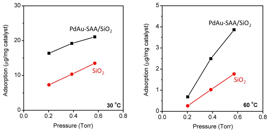
**Figure S6.** 1-hexyne adsorption isotherm at 30° and 60 °C with Pd<sub>0.004</sub>Au-SAA/SiO<sub>2</sub>.
