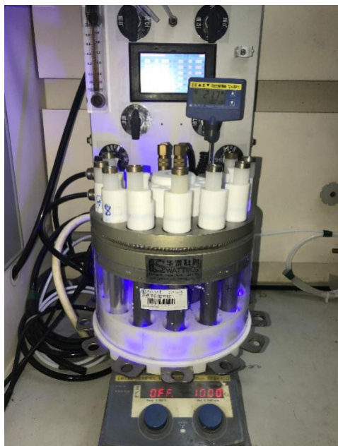
Wattecs Parallel Light Reactor (Blue LED Light source, 10 W every position)
