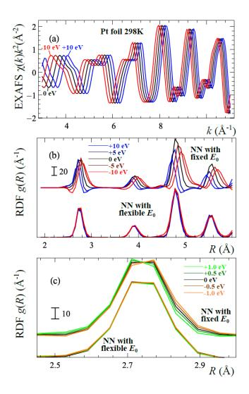
**Figure S3.** Experimental Pt L<sub>3</sub>-edge EXAFS spectra for a Pt foil (room temperature) shifted by  $\Delta E_0$  between -10 and +10 eV (a). Corresponding RDFs extracted by a NNs trained on data with fixed and flexible  $E_0$  values (b, c). For clarity, RDFs are shifted vertically in (b,c).
