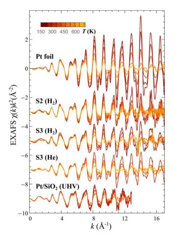
**Figure S2**. Experimental temperature-dependent Pt L<sub>3</sub>-edge EXAFS spectra for a Pt foil, Pt NPs supported on  $Al_2O_3$  (samples S2 and S3) and measured in H<sub>2</sub> and He atmospheres, and for Pt NPs deposited on  $SiO_2/Si(111)$  and measured in UHV. Spectra are shifted vertically for clarity.
