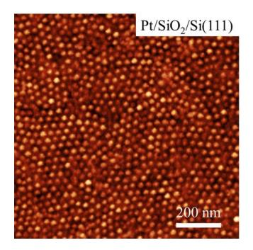
Figure S1.  $1 \times 1 \mu m$  AFM image of the as-prepared Pt nanoparticles (NPs) supported on SiO<sub>2</sub>/Si(111). Additional AFM images are available in Ref.[64].
