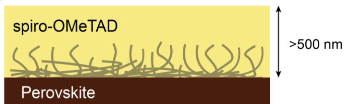
Figure S11: We can identify three thickness regimes for spiro-OMeTAD: a) thin spiro-OMeTAD, where spiro-OMeTAD is thinner than the penetration length of the SWCNTs ( < 200 nm); b) optimized spiro-OMeTAD thickness, where spiro-OMeTAD completely covers the SWCNTs but the travel distance for the charges is relatively short; c) thick spiro-OMeTAD, where the capping layer of spiro-OMeTAD is fairly thick and charges have to traverse a relatively large distance through the low-mobility material to reach the electrode.
