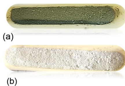
Figure S2 Aspect of a typical TiO 2 /graphene nanopowder obtained by laser pyrolysis before (a) and after (b) thermal annealing at 430°C for 6h in air.
