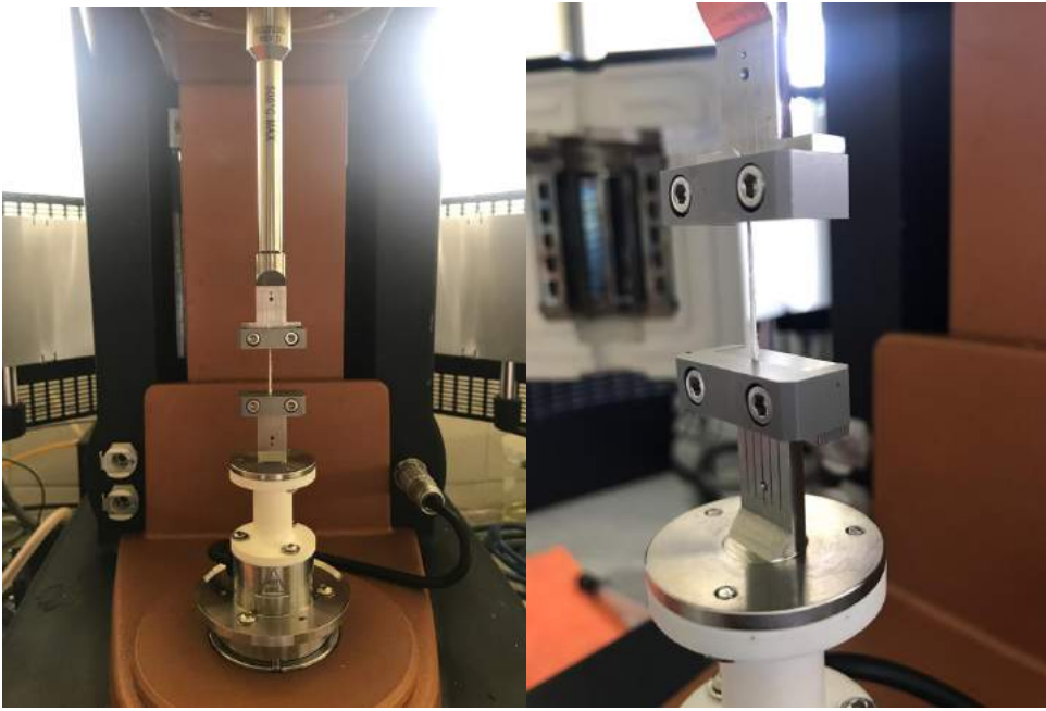
Figure S5. Show a photograph of this experimental set up for mechanical measurements. The specimens were tested as yarns of approximate diameter df = 900 \mu\text{m} and length L = 3 \text{ cm} by rolling flat fiber mats.
