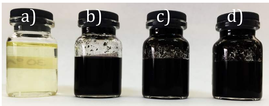
Figure S7. Macroscopic pictures of 7 ml vials: a) PVP/Ethanol 30 wt.%. (b-c) pristine Single Walled Carbon Nanotubes (Elicarb) suspension in PVP/Ethanol at different content of nanotubes, b) 0.02 wt.%, c) 0.1 wt.% and d) 0.2 wt.%. PVP content was maintained constant at 30 wt.% in all samples. Single walled Carbon nanotubes (SWNT) from Elicarb “Thomas Swan” (UK) with purity > 95%, average diameter = 2 nm, average BET specific surface area > 800 m 2 /g, metal oxide content: maximum of 5 wt.% and moisture content: maximum of 1 wt.% are presently used.
