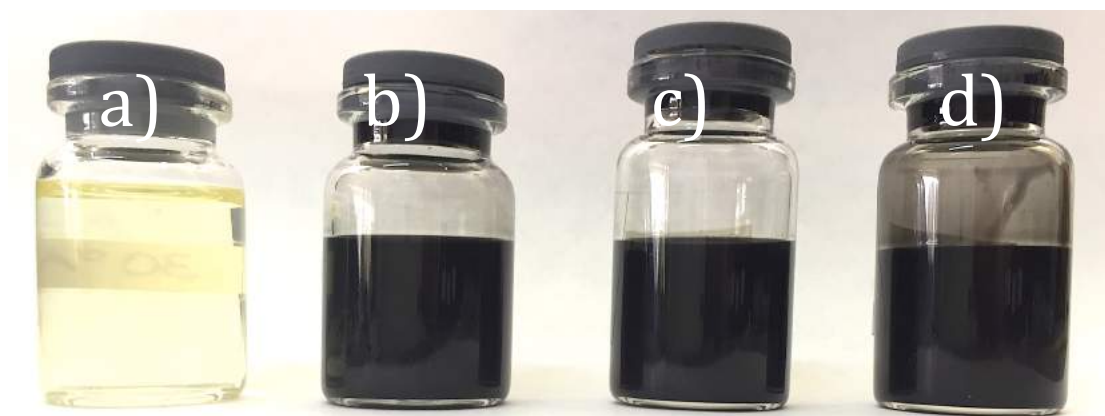
Figure S4. Macroscopic pictures of 7 ml vials: a) PVP/Ethanol 30 wt.%. (b-c) Functionalized Multi Walled Carbon Nanotubes (NanoAmor) suspensions in PVP/Ethanol at different content of nanotubes, b) 0.02 wt.%, c) 0.2 wt.% and d) 0.4 wt.%. PVP content was maintained constant at 30 wt.% in all samples.
