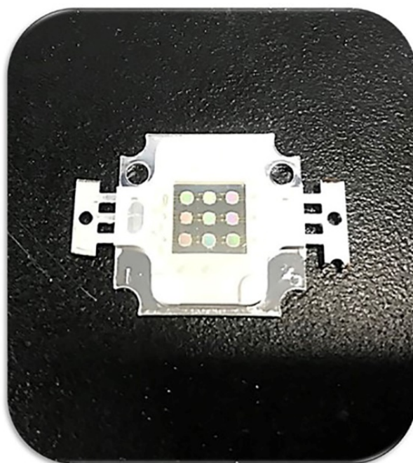
Figure S21 The photograph images of the white plane light source in off state.
