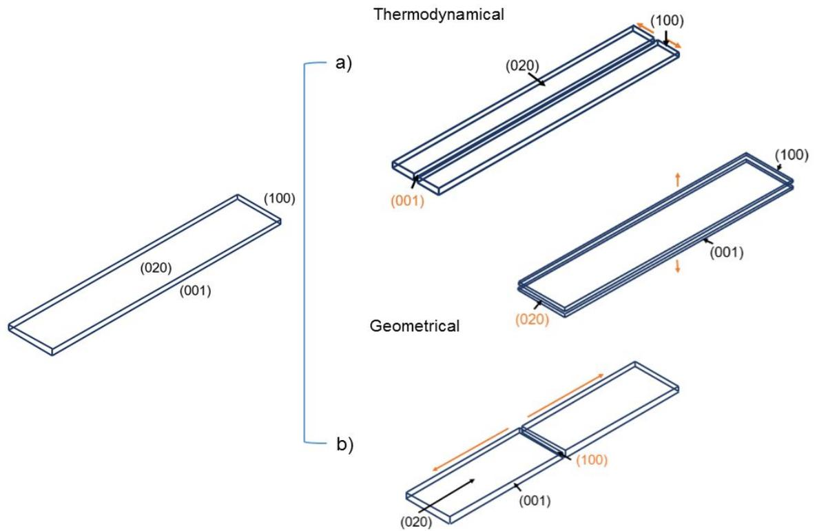
Figure S 2. Proposed fracture mechanism of a) AZD5423 and b) AZD4721 (data based on Figure S 3)
