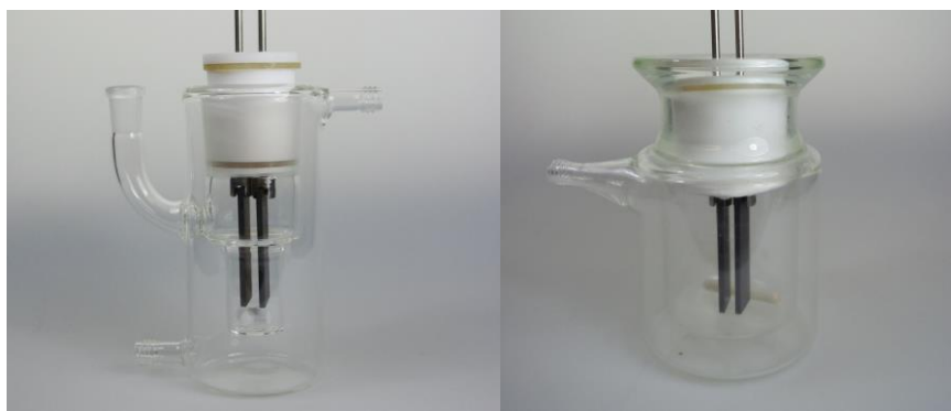
Figure S1: Double-jacketed beaker-type cell; left: 25 mL; right: 200 mL.
