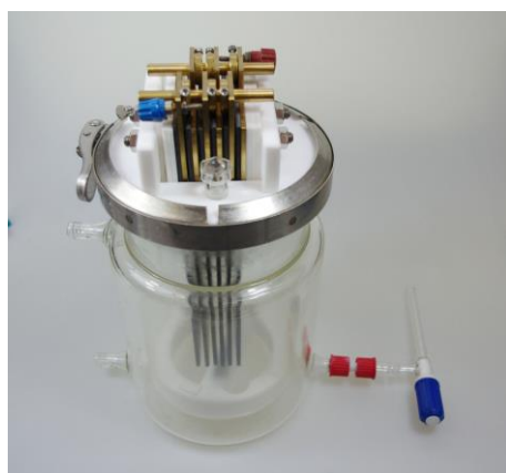
Figure S2: Double-jacketed 1500 mL beaker-type cell; left: assembled; right: technical illustration of the electrode arrangement.
