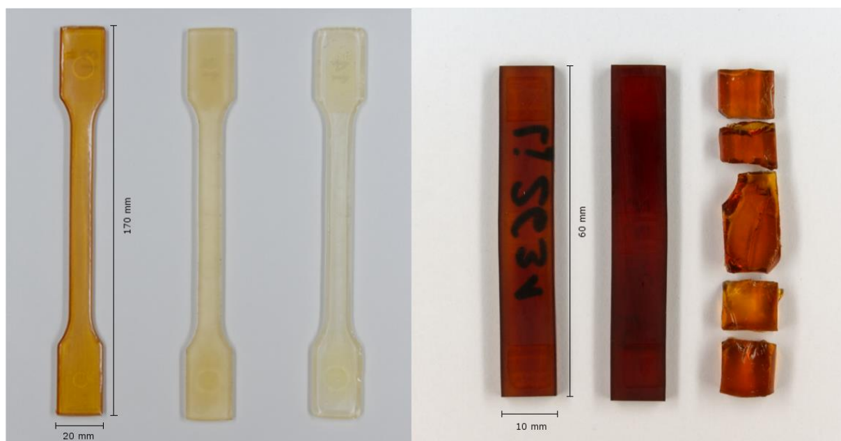
Figure S9: Test specimen, left: dog-bone shaped for tensile testing (ELPOXY-TOFA, PTP cured with MTHPA), right: bar-shaped DMA specimen of ELPOXY-TOFA cured with MTHPA, MNA and DDSA, respectively (deformed after recovery from DMA measurement sample holder).
