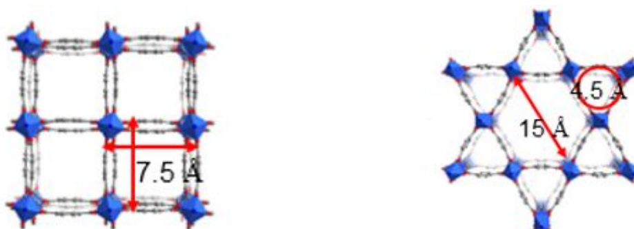
Figure S2: Crystal structure of DMOF-1 (left) and ZnBD (right). “Reproduced from 5. Copyright 2017, Elsevier.”
