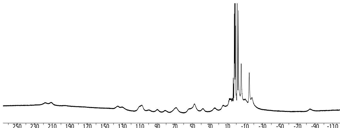
**Figure S3.**  $^1\text{H}$ -NMR spectra (400 MHz) of  $\mathbf{1}^{\text{Amide}}$  in  $\text{CD}_3\text{CN}$  at 298 K.
