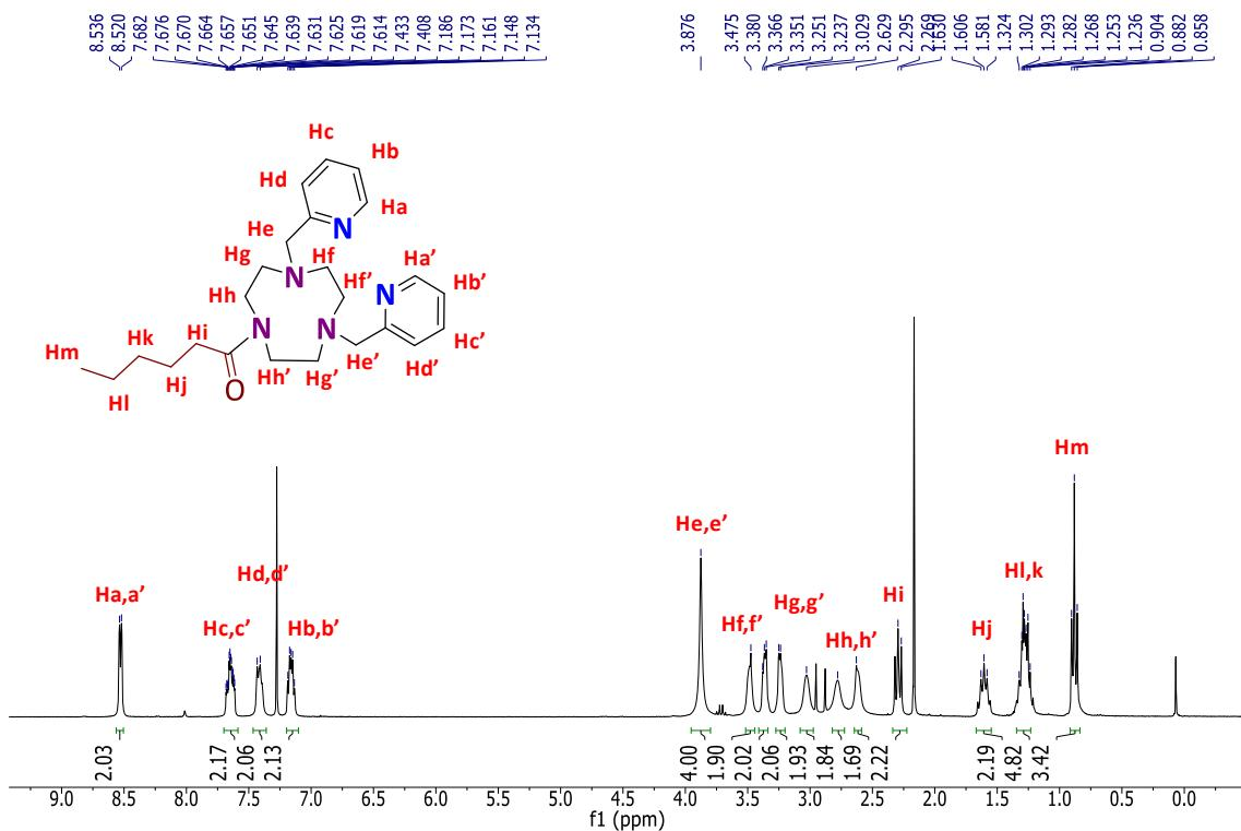
**Figure S97.**  $^1\text{H}$  NMR ( $\text{CDCl}_3$ , 500 MHz, 300 K) spectrum of  $^{\text{Amide}}\text{Py}_2\text{tacn}$ .
