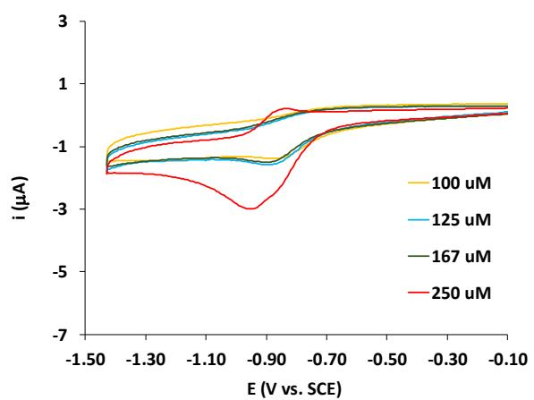
**Figure S15.** CVs of **biotin** (from 250 – 100  $\mu\text{M}$ ) in dry MeCN. Experimental conditions:  $\text{Bu}_4\text{NPF}_6$  (0.1 M) as supporting electrolyte in acetonitrile, using a  $0.28 \text{ cm}^2$  glassy carbon as working and SCE as reference electrodes. Scan rate of  $100 \text{ mV}\cdot\text{s}^{-1}$ .
