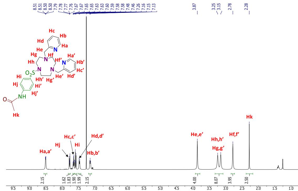
**Figure S102.**  $^1\text{H}$  NMR ( $\text{CDCl}_3$ , 400 MHz, 300 K) spectrum of  $^{\text{Amide-SP}}\text{Py}_2\text{tacn}$ .
