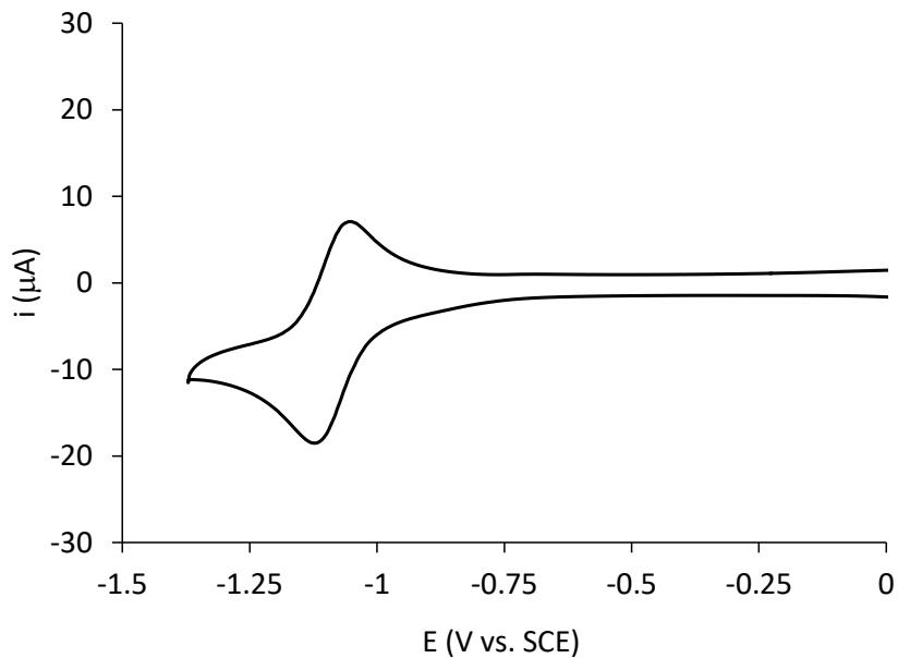
**Figure S10.** CVs of **1<sup>Bio</sup>** (1 mM) in dry MeCN. Experimental conditions: Bu<sub>4</sub>NPF<sub>6</sub> (0.1 M) as supporting electrolyte in acetonitrile, using a 0.28 cm<sup>2</sup> glassy carbon as working and SCE as reference electrodes. Scan rate of 100 mV·s<sup>-1</sup>.
