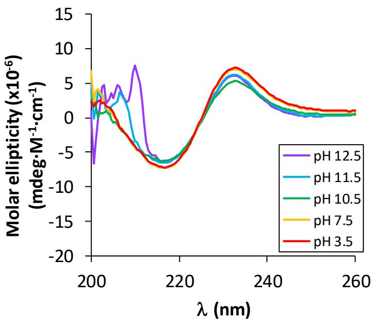
**Figure S60.** CD spectra of **SA** at different pHs analogous to photocatalytic (pH 7.5 to 12.5) and electrocatalytic (pH 3.5) conditions: 5  $\mu$ M **SA**, 100 mM phosphite buffer:MeCN mixtures (3:7, v/v) at 20 °C. The CD at pH 7.5 has been measured in 100 mM Tris · HCl buffer pH 7.5.
