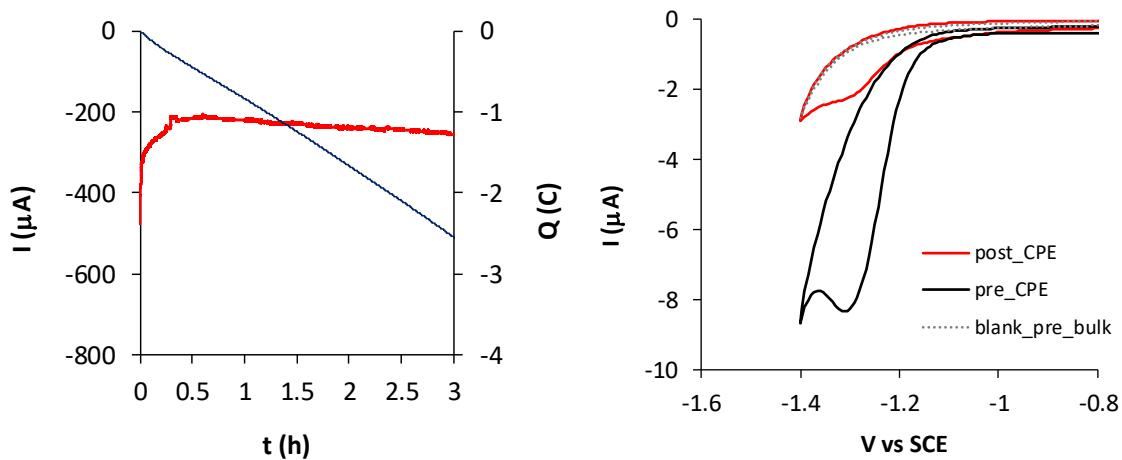
**Figure S50.** *Left)* Bulk electrolysis of **2<sup>Bio</sup> C SA** (73  $\mu\text{M}$ ) in 100 mM citrate buffer 100 mM NaCl pH 3.5 under N<sub>2</sub> atmosphere at  $E_{\text{appl}} = -1.4$  V vs SCE using a carbon mesh as working electrode, Pt wire as counter electrode and SCE as reference electrode. Represented are the current (red) and charge (blue) passed over 3 h. *Right)* CV before (blank) and after (red) the CPE.
