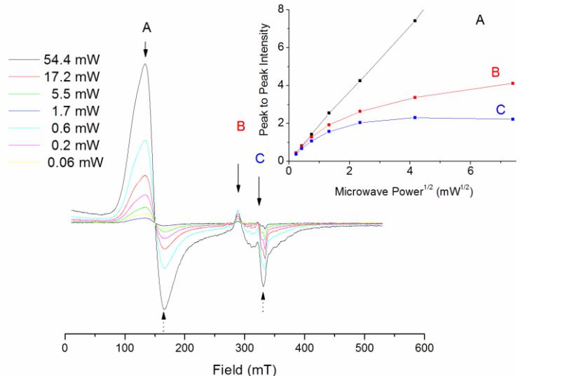
**Figure S30.** EPR power saturation of **2<sup>Bio</sup>** at 15K.
