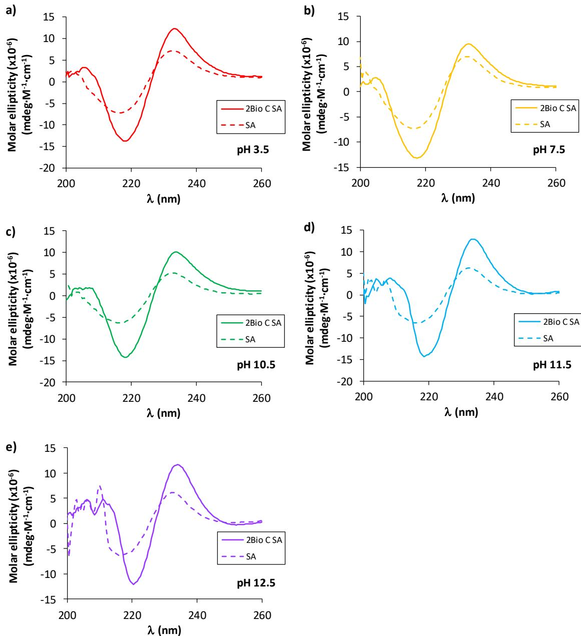
**Figure S61.** Comparison of the CD spectra of **2<sup>Bio</sup> C SA** and **SA** at different pHs analogous to photocatalytic (pH 7.5 to 12.5) and electrocatalytic (pH 3.5) conditions: 5  $\mu$ M **2<sup>Bio</sup> C SA** or **SA**, 100 mM phosphite buffer:MeCN mixtures (3:7, v/v) at 20 °C. The CD at pH 7.5 has been measured in 100 mM Tris · HCl buffer pH 7.5.
