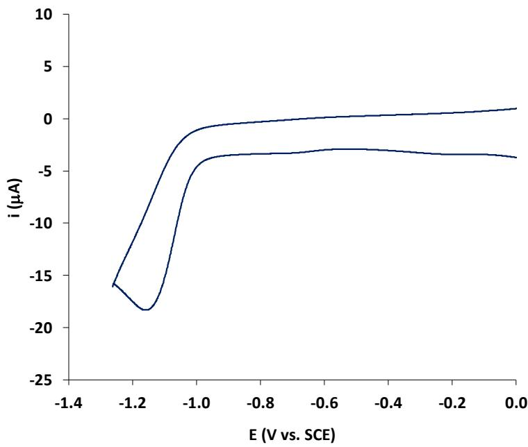
**Figure S13.** CV of **2<sup>Amide</sup>** (1 mM) in dry MeCN. Experimental conditions: Bu<sub>4</sub>NPF<sub>6</sub> (0.1 M) as supporting electrolyte in acetonitrile, using a 0.28 cm<sup>2</sup> glassy carbon as working and Ag pseudoreference and the Fc/Fc<sup>+</sup> couple as reference electrodes. Scan rate of 100 mV·s<sup>-1</sup>.
