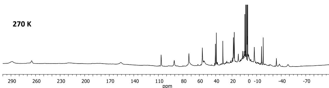
**Figure S1.**  $^1\text{H-NMR}$  spectra (500 MHz) of  $\mathbf{1}^{\text{Bio}}$  in  $\text{CD}_3\text{CN}$  at 270K.
