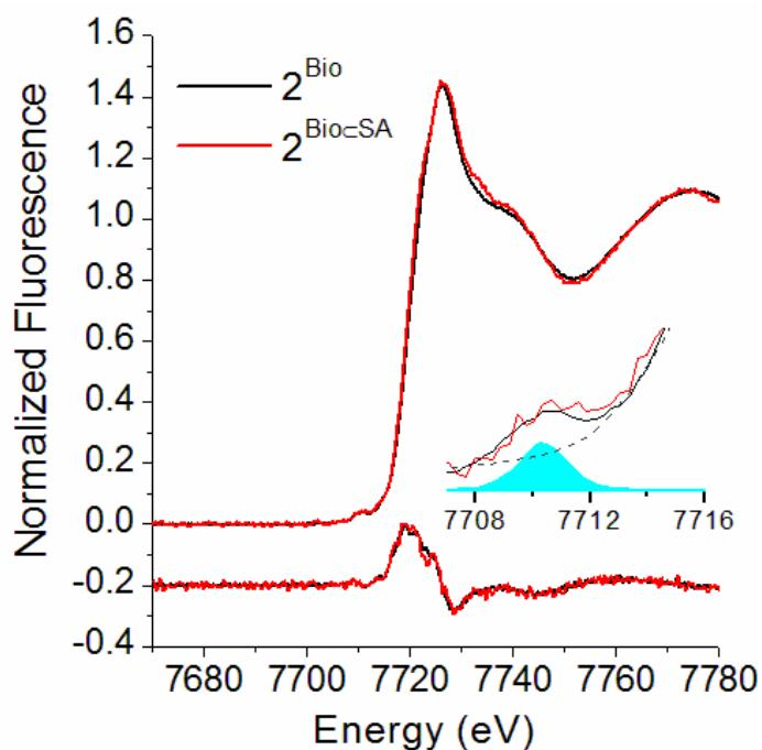
**Figure S26.** Co K-edge XANES spectra of **2<sup>Bio</sup>** and **2<sup>Bio</sup>C SA** and the corresponding derivative. Inset: Pre-edge area and fit centered at 7710.4 eV with an intensity of 0.06 (cyan).
