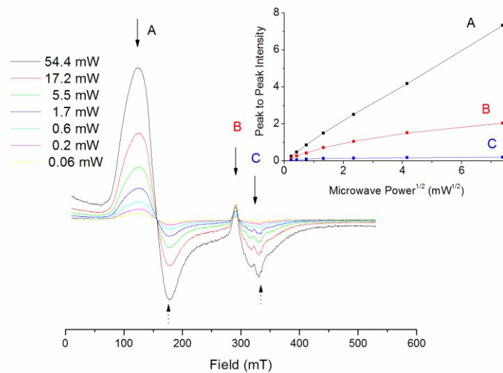
**Figure S28.** EPR power saturation of **1<sup>Bio</sup>** at 15K.
