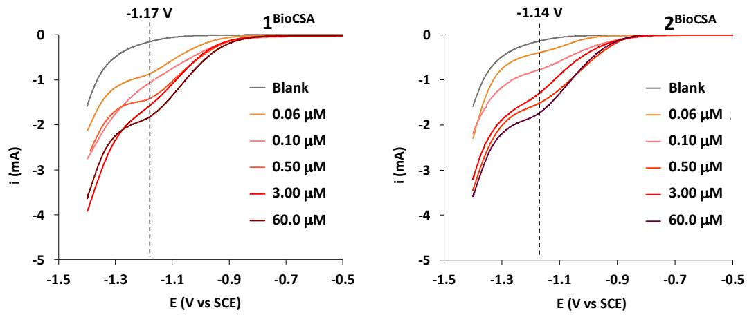
**Figure S40.** Cyclic voltammograms of the thin film electrochemistry of *Left*) **1**<sup>BioCSA</sup> and *Right*) **2**<sup>BioCSA</sup> in buffer (citrate 100 mM, NaCl 100 mM) at pH 3.5 at increasing concentrations (from 0.06 to 60  $\mu$ M) of the metalloprotein onto the surface of the carbon fabric working electrode ( $1 \text{ cm}^2$  surface). Scan rate of  $10 \text{ mV}\cdot\text{s}^{-1}$ . Potentials are quoted versus SCE.
