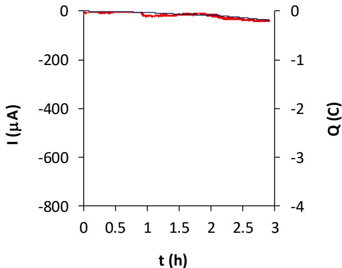
**Figure S49.** Bulk electrolysis of 100 mM citrate buffer 100 mM NaCl pH 3.5 under N<sub>2</sub> atmosphere at  $E_{\text{appl}} = -1.4$  V vs SCE using a carbon mesh as working electrode, Pt wire as counter electrode and SCE as reference electrode. Represented are the current (red) and charge (blue) passed over 3 h.
