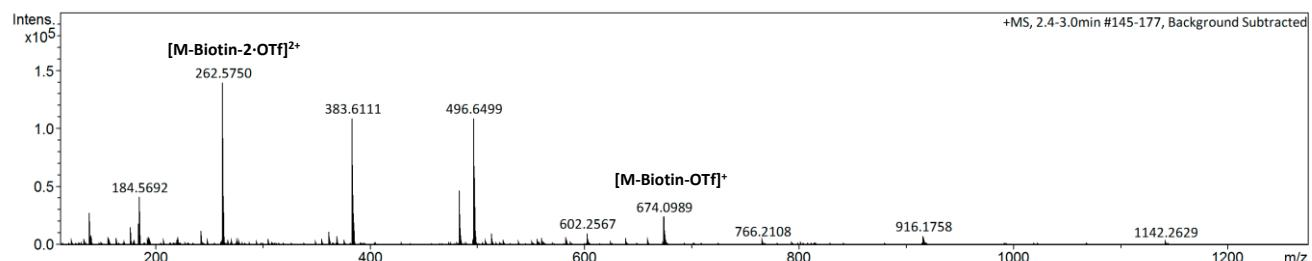
**Figure S7.** HR-MS-ESI spectrum of  $2^{\text{Bio}}$ .  $[\text{M-biotin-2-OTf}]^{2+}$  and  $[\text{M-biotin-OTf}]^+$  stand for  $[\text{Co}(\text{^{SP}Py}_2\text{tacn})]^{2+}$  and  $[\text{Co}(\text{^{SP}Py}_2\text{tacn})(\text{OTf})]^+$ , respectively.
