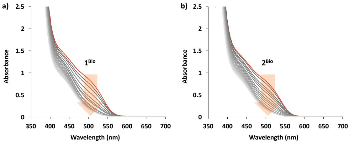
**Figure S18.** UV/Vis absorption decay in of the HABA C SA complex upon the addition of different amounts of **1<sup>Bio</sup>** (*Top*) and **2<sup>Bio</sup>** (*Bottom*) in 300 mM phosphate, pH 7 and saturated with 533.35  $\mu\text{M}$  HABA.
