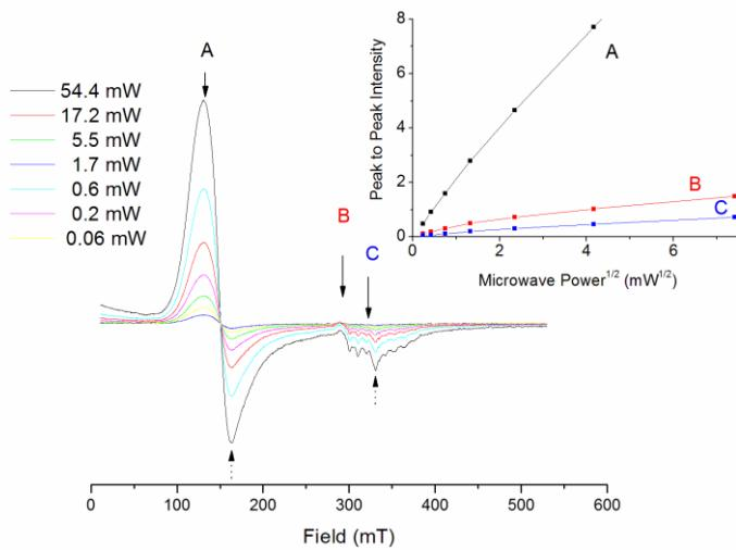
**Figure S31.** EPR power saturation of **2<sup>Bio</sup> C SA** at 15K.
