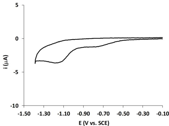
**Figure S11.** CVs of **2<sup>Bio</sup>** (0.25 mM) in dry MeCN. Experimental conditions: Bu<sub>4</sub>NPF<sub>6</sub> (0.1 M) as supporting electrolyte in acetonitrile, using a 0.28 cm<sup>2</sup> glassy carbon as working and SCE as reference electrodes. Scan rate of 100 mV·s<sup>-1</sup>.
