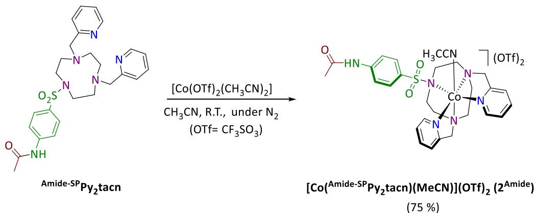
**Scheme S12.** Synthesis of  $[\text{Co}(\text{Amide-SPPy}_2\text{tacn})(\text{MeCN})](\text{OTf})_2$  ( $\mathbf{2}^{\text{Amide}}$ ).
