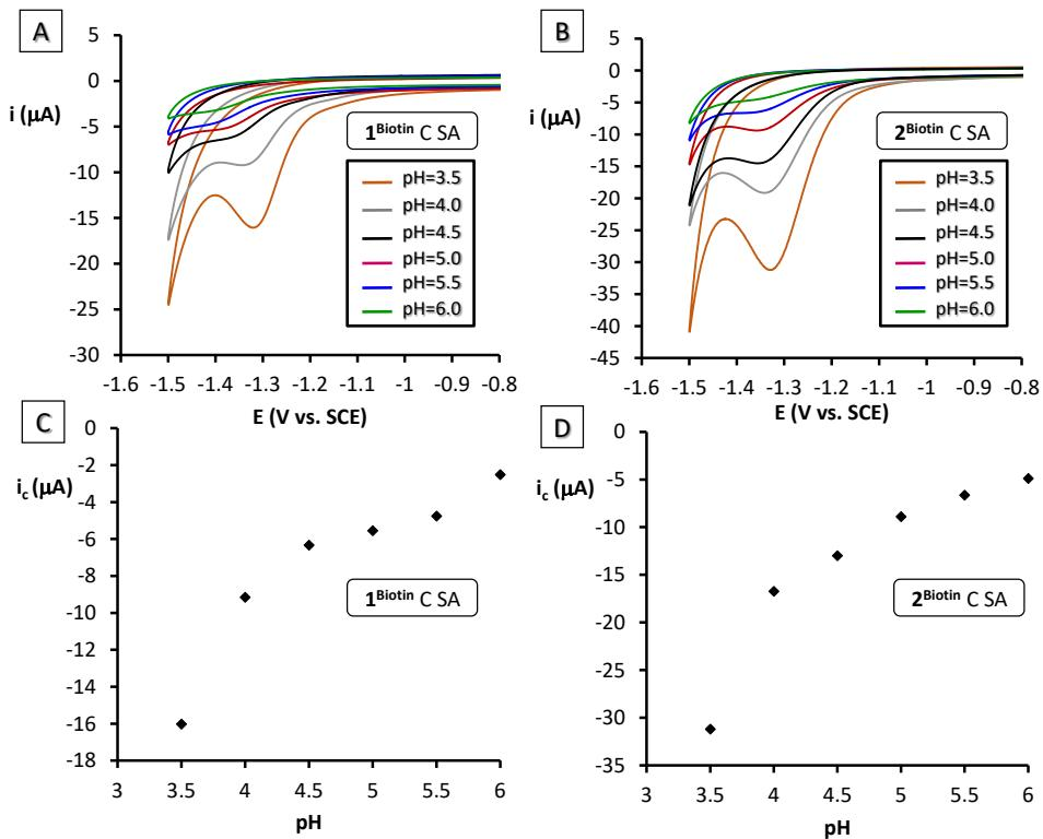
**Figure S42.** CV of thin films of A) **1<sup>Bio</sup> C SA** (A and B) **2<sup>Bio</sup> C SA** adducts in buffer (citrate 100 mM, NaCl 100 mM) in the pH 3.5 - 6.0 range. Scan rate of 100 mV·s<sup>-1</sup> using a 0.28 cm<sup>2</sup> glassy carbon working electrode. Potentials are quoted versus SCE. Maximum peak intensity values versus pH for C) **1<sup>Bio</sup> C SA** and D) **2<sup>Bio</sup> C SA**.
