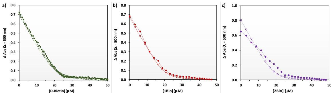
**Figure S20.** Fitting (empty dots) for the HABA displacement assay of SA by **D-biotin** (green dots, a) **1<sup>Bio</sup>** (red dots, b) and **2<sup>Bio</sup>** (purple dots, c). The fitting has been performed by taking into account a  $K_{exch}$  of 3, obtaining an association constant of about  $1 \cdot 10^7 \text{ M}^{-1}$  for the biotinylated catalysts.
