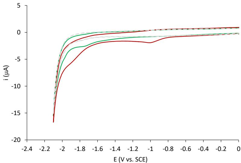
**Figure S14.** Cyclic voltammograms in CH<sub>2</sub>Cl<sub>2</sub> containing 100 mM Bu<sub>4</sub>NPF<sub>6</sub> in the absence (dashed grey trace), and presence of 0.5 mM of **BioPy<sub>2</sub>tacn** (green trace) and **Bio-SPy<sub>2</sub>tacn** (red trace) ligands. Scan rate of 100 mV·s<sup>-1</sup> using a 0.28 cm<sup>2</sup> glassy carbon working electrode. Potentials are quoted versus SCE.
