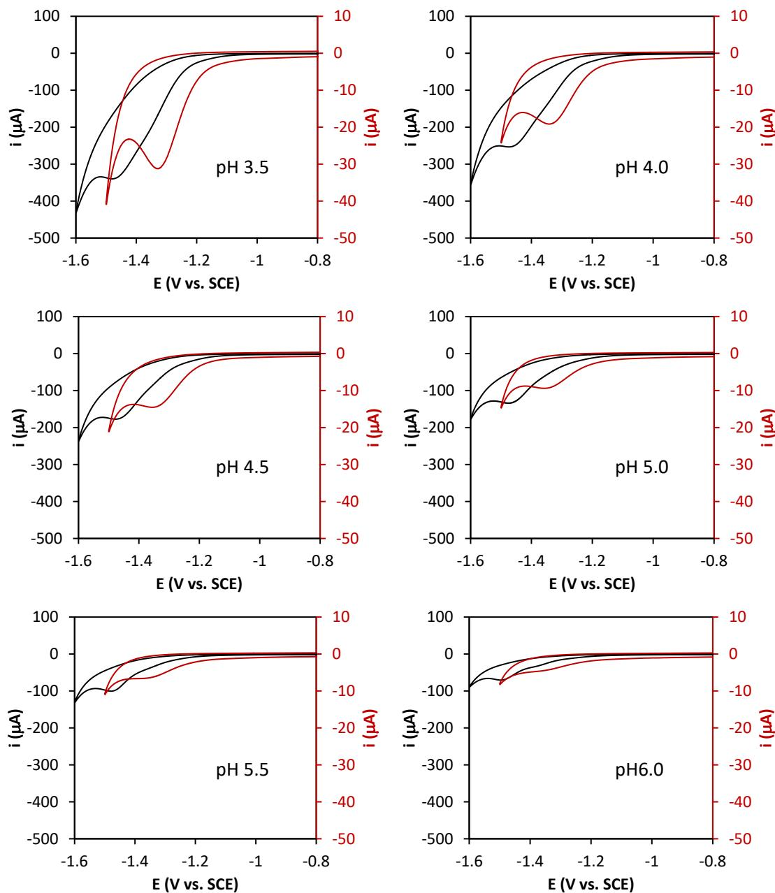
**Figure S45.** Cyclic voltammograms of **2<sup>Bio</sup>** (black trace) **2<sup>Bio</sup>C SA** (red trace). CVs measured in 100 mM citrate buffer, 100 mM NaCl, at different pH values. Scan rate of 100 mV·s<sup>-1</sup> using a 0.28 cm<sup>2</sup> glassy carbon working electrode. Potentials are quoted versus SCE.
