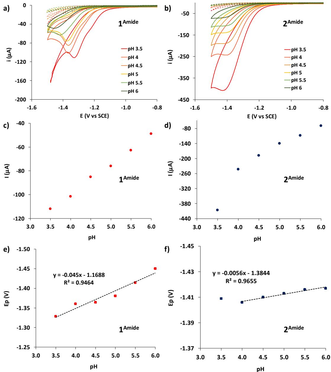
**Figure S55.** Cyclic voltammograms (CV) of a) **1**<sup>Amide</sup> (1 mM) and b) **2**<sup>Amide</sup> (1 mM) in buffer (citrate 100 mM, NaCl 100 mM) in the pH 3.5 - 6.0 range. Scan rate: 100 mV·s<sup>-1</sup>. Working electrode glassy carbon (0.28 cm<sup>2</sup>). Maximum peak intensity values versus pH for c) **1**<sup>Amide</sup> and d) **2**<sup>Amide</sup>. Plot of the peak potential (Ep) as a function of pH of e) **1**<sup>Amide</sup> and f) **2**<sup>Amide</sup>.
