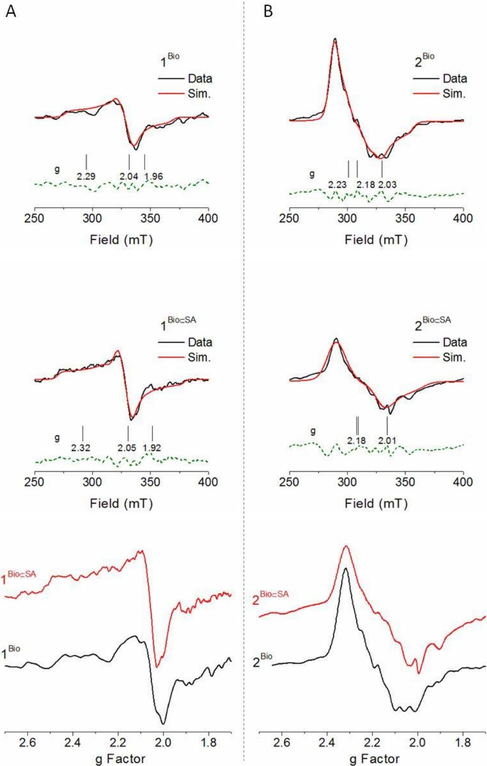
**Figure S27.** (A) EPR spectra and simulation of **1<sup>Bio</sup>** ( $A_z$ ,  $A_x$ ,  $A_y$ = 152.0, 5.6, 163.4, MHz), and **1<sup>Bio</sup> C SA** ( $A_z$ ,  $A_x$ ,  $A_y$ = 174.6, 2.8, 182.0, MHz). (B) EPR spectra and simulation of **2<sup>Bio</sup>** ( $A_z$ ,  $A_x$ ,  $A_y$ = 161.9, 105.1, 190.7 MHz), and **2<sup>Bio</sup> C SA** ( $A_z$ ,  $A_x$ ,  $A_y$ = 150.2, 169.1, 221.9, MHz) measured at 77K.
