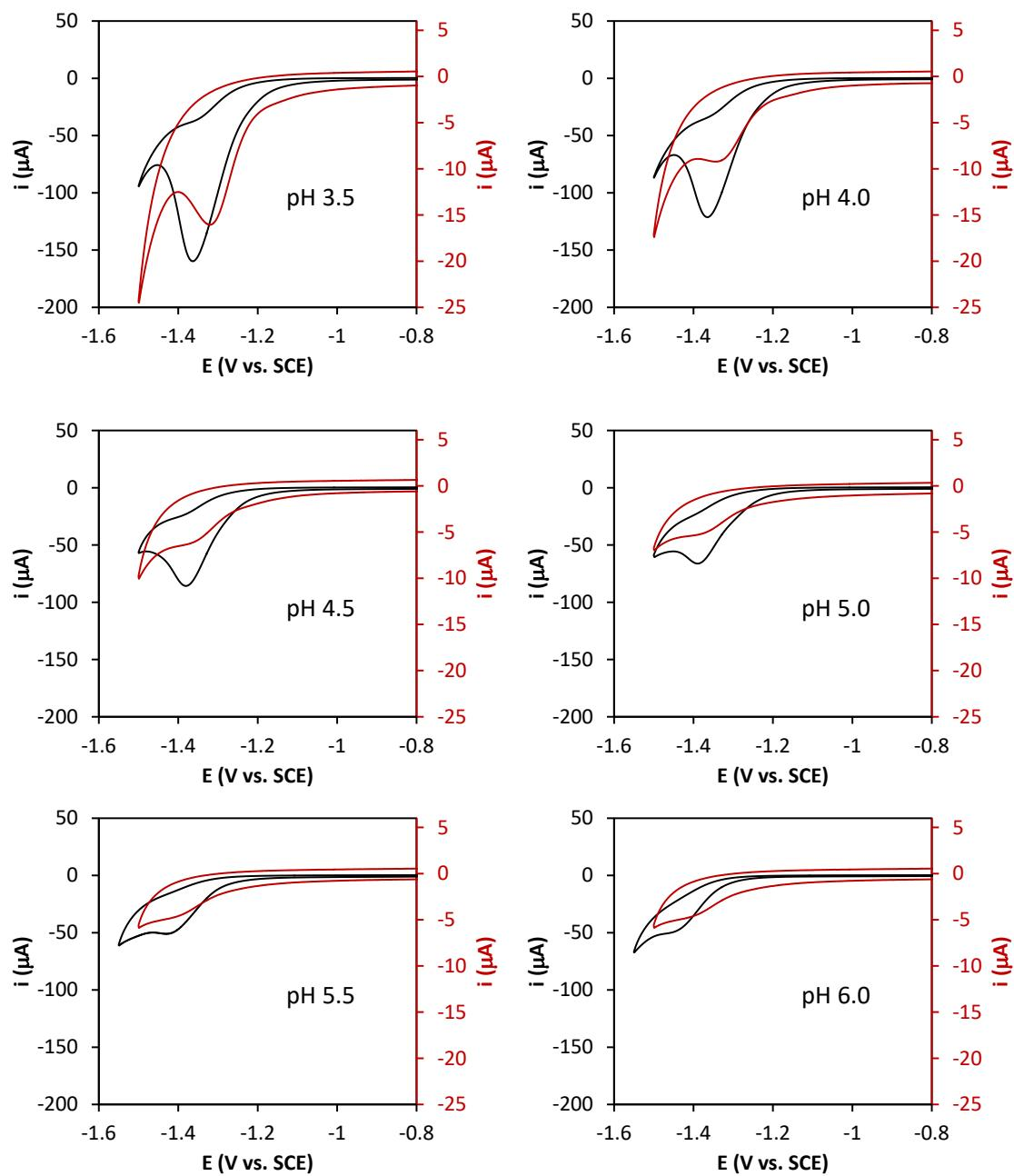
**Figure S44.** Cyclic voltammograms of **1<sup>Bio</sup>** (black trace) **1<sup>Bio</sup>-SA** (red trace). CVs measured in 100 mM citrate buffer, 100 mM NaCl, at different pH values, at scan rate of 100 mV·s<sup>-1</sup> using a 0.28 cm<sup>2</sup> glassy carbon working electrode. Potentials are quoted versus SCE.
