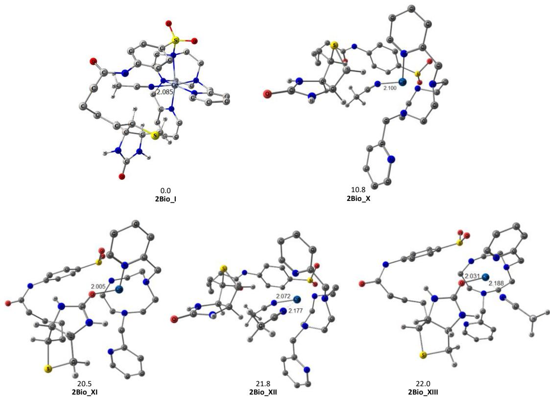
**Figure S85.** Optimized geometries of the lowest in energy possible isomers of **2Bio** complexes with a decoordination pyridine and with and without the biotin bonded to the metal center. Selected hydrogen atoms are omitted for clarity. Relevant bond distances are in Å. Free energy values in kcal·mol<sup>-1</sup> and referenced to **2Bio\_I**.
