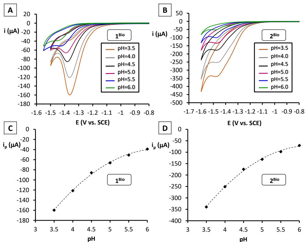
**Figure S35.** Cyclic voltammograms (CV) of **A**  $\mathbf{1}^{\text{Bio}}$  (1 mM) and **B**  $\mathbf{2}^{\text{Bio}}$  (1 mM) in buffer (citrate 100 mM, NaCl 100 mM) in the pH 3.5 - 6.0 range. Scan rate: 100 mV·s<sup>-1</sup>. Working electrode glassy carbon (0.28 cm<sup>2</sup>). Maximum peak intensity values versus pH for **C**  $\mathbf{1}^{\text{Bio}}$  and **D**  $\mathbf{2}^{\text{Bio}}$ .
