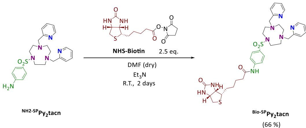
**Scheme S6.** Synthesis of <sup>Bio-SP</sup>**Py<sub>2</sub>tacn**.
