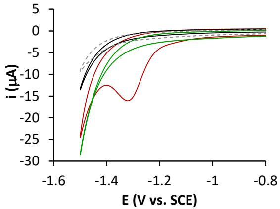
**Figure S38.** CV of a  $10 \mu\text{M}$   $\mathbf{1}^{\text{Bio}}$  C SA in solution (green trace) and as a thin film (red trace), bare electrode (dashed grey trace) and the CV of a thin film of SA (black trace). Conditions:  $100 \text{ mM}$  citrate buffer,  $100 \text{ mM}$  NaCl, at pH 3.5. Scan rate:  $100 \text{ mV}\cdot\text{s}^{-1}$ . Working electrode: glassy carbon ( $0.28 \text{ cm}^2$ ).
