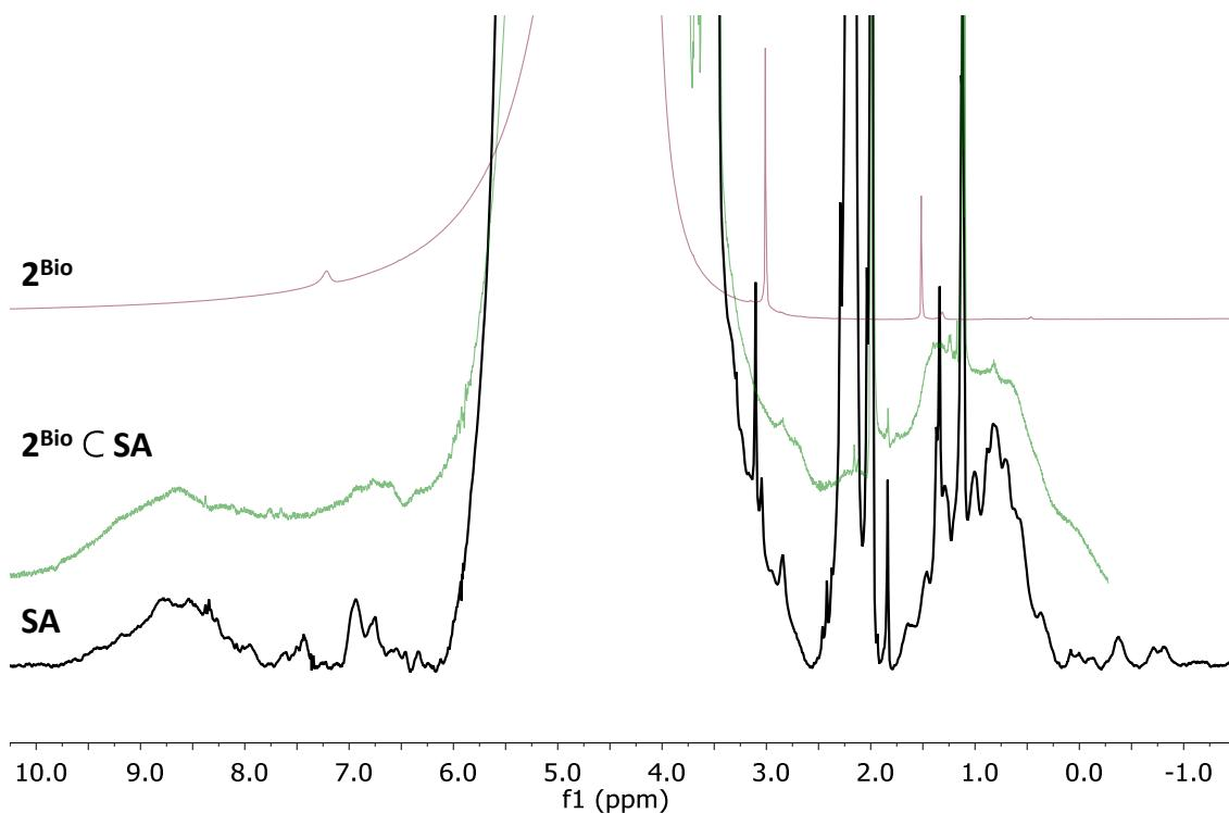
**Figure S24.** From *top* to *bottom*: Magnification of the diamagnetic region of the  $^1\text{H}$ -NMR spectra (500 MHz, Tris-HCl buffer pH 7.5: $\text{CD}_3\text{CN}$  (7:3) at 280 K) of **2<sup>Bio</sup>**, **2<sup>Bio</sup> C SA** and **SA**.
