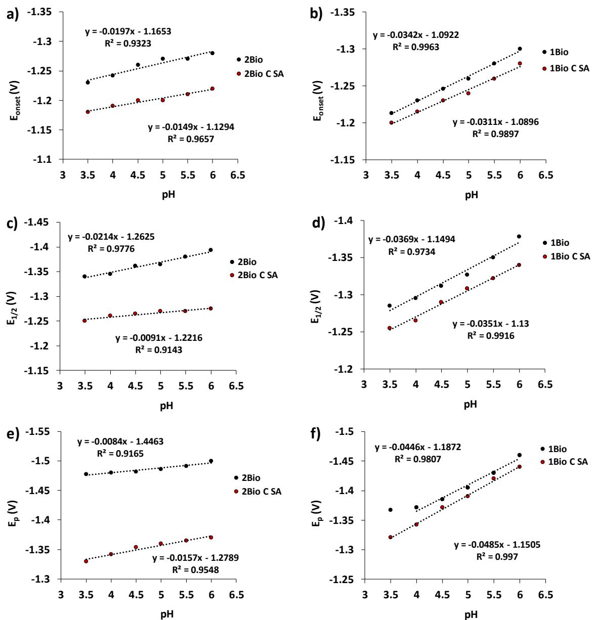
**Figure S46.** Plots of **a-b)** the onset potential ( $E_{\text{onset}}$ ), **c-d)** half peak potential ( $E_{1/2}$ ), and **e-f)** peak potential ( $E_p$ ) as a function of pH of **1<sup>Bio</sup>** (1 mM) and **1<sup>Bio</sup> C SA** (thin film) and **2<sup>Bio</sup>** (1 mM) and **2<sup>Bio</sup> C SA** (thin film) in buffer (citrate 100 mM, NaCl 100 mM) in the pH 3.0 - 6.0 range. Scan rate: 100 mV·s<sup>-1</sup>. Working electrode glassy carbon (0.28 cm<sup>2</sup>).
