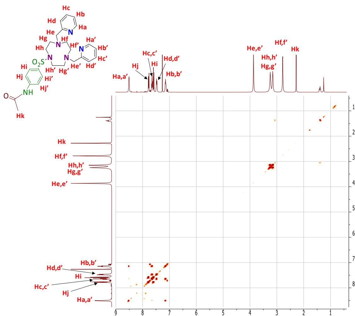
**Figure S104.**  $^1\text{H}$ - $^1\text{H}$  COSY ( $\text{CDCl}_3$ , 400 MHz, 300 K) spectrum of  $^{\text{Amide-SP}}\text{Py}_2\text{tacn}$ .
