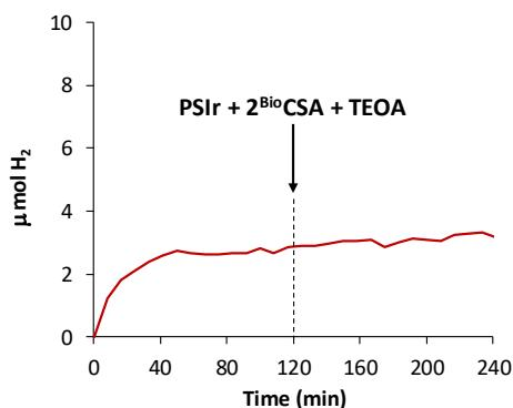
**Figure S64.** Time traces of the photoinduced H<sub>2</sub> production and recovery using **2<sup>Bio</sup> C SA** (5  $\mu$ M), **PSIr** (250  $\mu$ M), TEOA (0.4 M) in 4.2 mL of CH<sub>3</sub>CN:phosphate buffer (3:7 v/v) (100 mM) at pH 10.5 after 4 h irradiation (1100 W·m<sup>-2</sup>,  $\lambda > 400$  nm) and after further addition of **PSIr + 2<sup>Bio</sup> + TEOA** after reaching the plateau after 2 h of irradiation.
