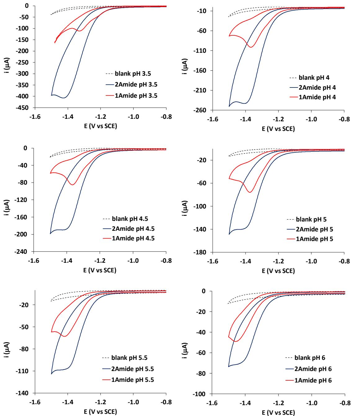
**Figure S56.** Cyclic voltammograms of **1**<sup>Amide</sup> and **2**<sup>Amide</sup> in buffer (citrate 100 mM, NaCl 100 mM) in the pH 3.5 - 6.0 range. Scan rate of 100 mV·s<sup>-1</sup> using a 0.28 cm<sup>2</sup> glassy carbon working electrode. Potentials are quoted versus SCE.
