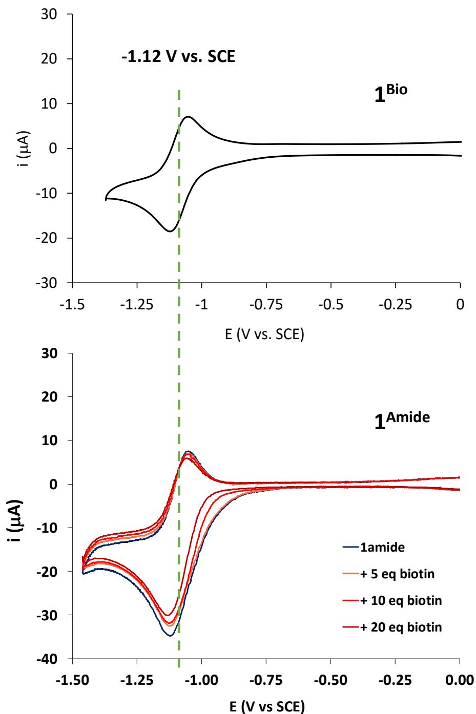
**Figure S53.** CVs of *Top*) **1<sup>Bio</sup>** (1 mM) in dry MeCN and *Bottom*) CV of **1<sup>Amide</sup>** (1 mM) in dry MeCN and CVs of the subsequent addition of biotin ethyl ester (from 5 to 20 eq). Experimental conditions: Bu<sub>4</sub>NPF<sub>6</sub> (0.1 M) as supporting electrolyte in acetonitrile, using a 0.28 cm<sup>2</sup> glassy carbonas working and Ag pseudoreference and the Fc/Fc<sup>+</sup> couple as reference electrodes. Scan rate of 100 mV·s<sup>-1</sup>.
