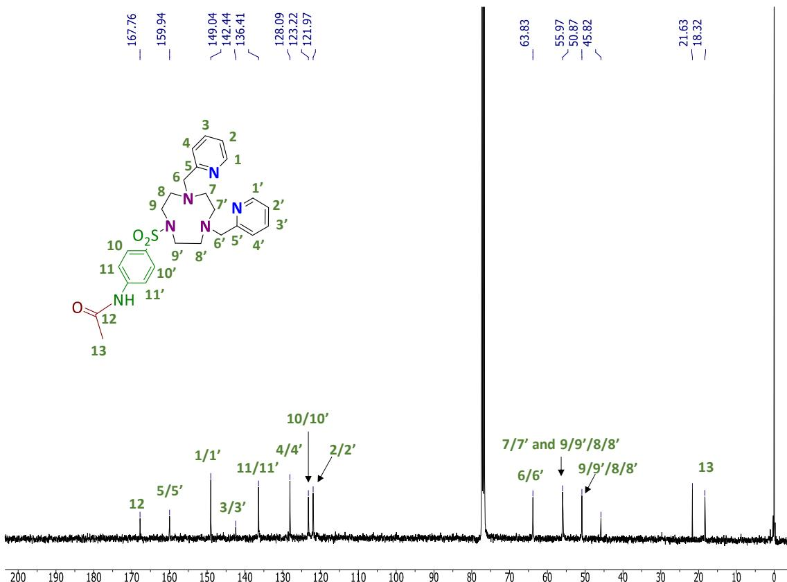
**Figure S103.**  $^{13}\text{C}$  NMR ( $\text{CDCl}_3$ , 101 MHz, 300 K) spectrum of Amide-SP Py<sub>2</sub>tacn.
