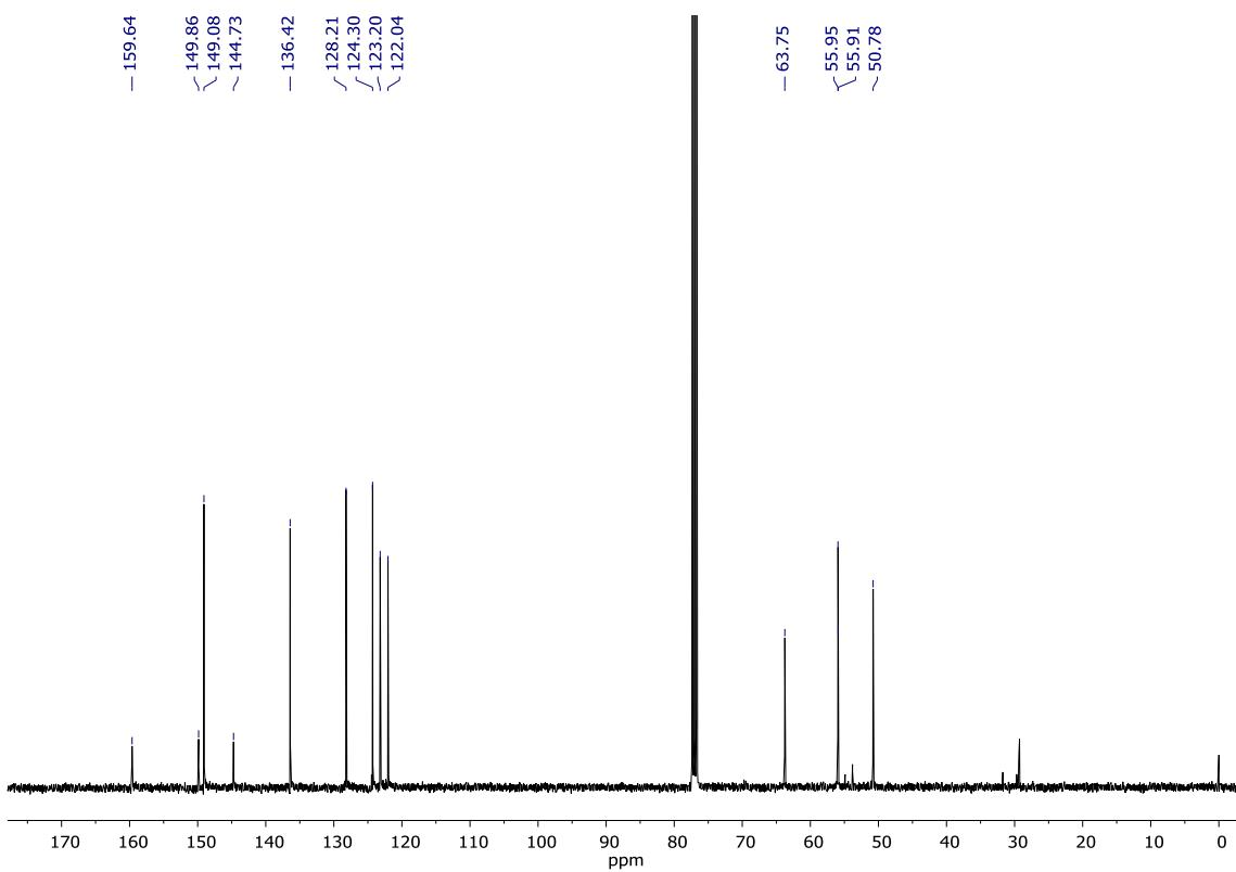
**Figure S93.**  $^{13}\text{C}$  NMR ( $\text{CDCl}_3$ , 101 MHz, 300 K) spectrum  $^{\text{NO}_2}\text{Py}_2\text{tacn}$ .
