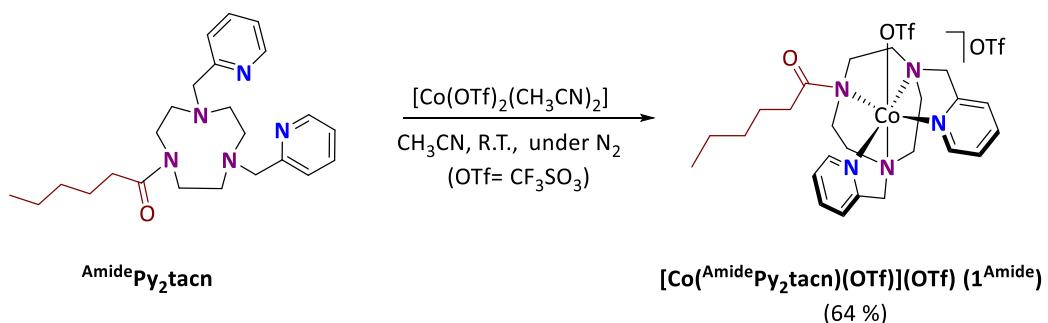
**Scheme S11.** Synthesis of  $[\text{Co}(\text{Amide Py}_2\text{tacn})(\text{MeCN})](\text{OTf})_2 (1^{\text{Amide}})$ .
