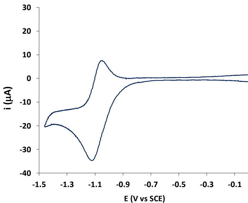
**Figure S12.** CV of **1<sup>Amide</sup>** (1 mM) in dry MeCN. Experimental conditions: Bu<sub>4</sub>NPF<sub>6</sub> (0.1 M) as supporting electrolyte in acetonitrile, using a 0.28 cm<sup>2</sup> glassy carbon as working and Ag pseudoreference and the Fc/Fc<sup>+</sup> couple as reference electrodes. Scan rate of 100 mV·s<sup>-1</sup>.
