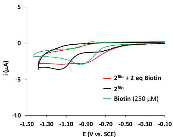
**Figure S16.** CVs of **biotin** (0.25 mM),  $\mathbf{2}^{\text{Bio}}$  (0.25 mM) and  $\mathbf{2}^{\text{Bio}}$  after the addition of 2 eq of biotin in dry MeCN. Experimental conditions:  $\text{Bu}_4\text{NPF}_6$  (0.1 M) as supporting electrolyte in acetonitrile, using a  $0.28 \text{ cm}^2$  glassy carbon as working and SCE as reference electrodes. Scan rate of  $100 \text{ mV}\cdot\text{s}^{-1}$ .
