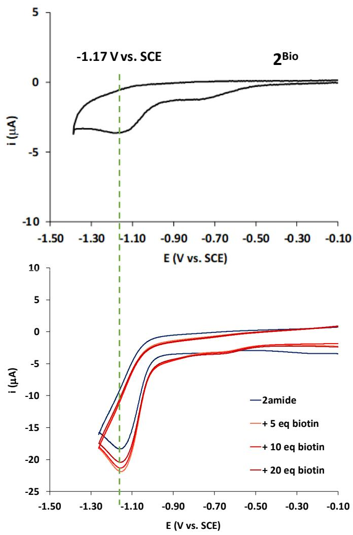
**Figure S54.** CVs of *Top*) **2<sup>Bio</sup>** (0.25 mM) in dry MeCN and *Bottom*) **2<sup>Amide</sup>** (1 mM) in dry MeCN and CVs of the subsequent addition of biotin ethyl ester (from 5 to 20 eq). Experimental conditions: Bu<sub>4</sub>NPF<sub>6</sub> (0.1 M) as supporting electrolyte in acetonitrile, using a 0.28 cm<sup>2</sup> glassy carbon as working and Ag pseudoreference and the Fc/Fc<sup>+</sup> couple as reference electrodes. Scan rate of 100 mV·s<sup>-1</sup>.
