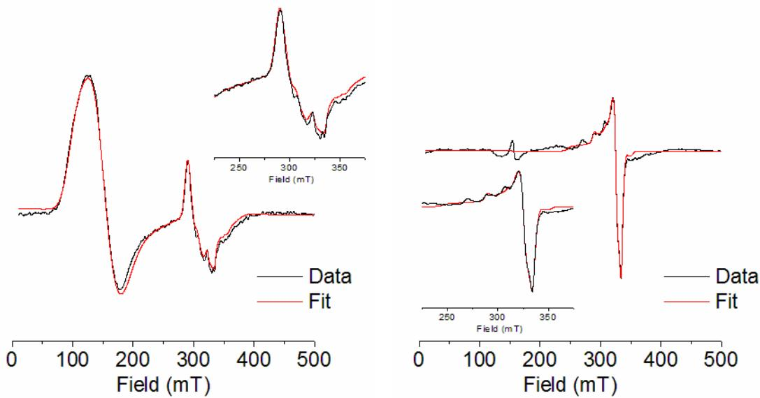
**Figure S34.** EPR spectra (black line) and simulation (red line) of  $\mathbf{1}^{\text{Bio}}$  (left) and  $\mathbf{1}^{\text{Bio}} \text{ C SA}$  (right) (0.35 mM) in  $\text{H}_2\text{O}:\text{MeCN}$  (7:3, 0.1 M Tris.HCl buffer pH 7.5) at 25 dB power and 15 K.
