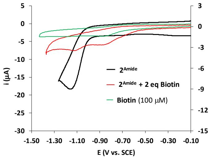
**Figure S17.** CVs of **biotin** (0.1 mM), **2<sup>Amide</sup>** (1 mM) and **2<sup>Amide</sup>** (0.25 mM) after the addition of 2 eq of biotin in dry MeCN. Experimental conditions: Bu<sub>4</sub>NPF<sub>6</sub> (0.1 M) as supporting electrolyte in acetonitrile, using a 0.28 cm<sup>2</sup> glassy carbon as working and SCE as reference electrodes. Scan rate of 100 mV·s<sup>-1</sup>.
