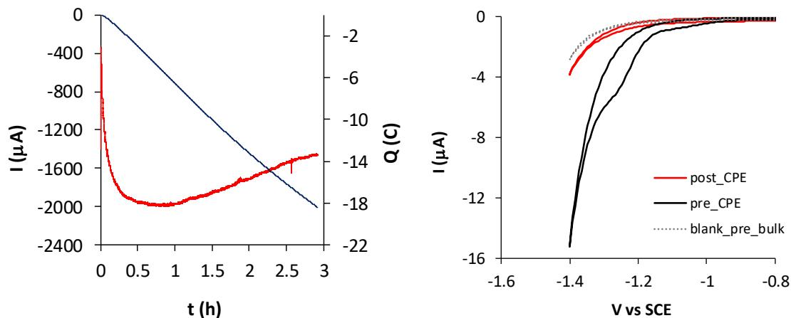
**Figure S51.** *Left)* Bulk electrolysis of  $\mathbf{2}^{\text{Bio}}$  ( $73 \mu\text{M}$ ) in  $100 \text{ mM}$  citrate buffer  $100 \text{ mM}$  NaCl pH 3.5 under  $\text{N}_2$  atmosphere at  $E_{\text{appl}} = -1.4 \text{ V}$  vs SCE using a carbon mesh as working electrode, Pt wire as counter electrode and SCE as reference electrode. Represented are the current (red) and charge (blue) passed over 3 h. *Right)* CV before (blank) and after (red) the CPE.
