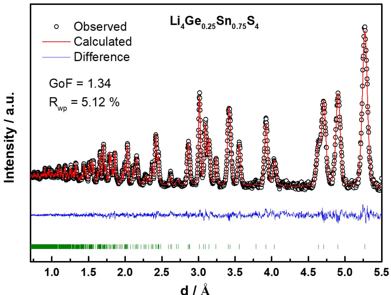
Figure S4: Neutron powder diffraction data for  $\text{Li}_4\text{Ge}_{0.25}\text{Sn}_{0.75}\text{S}_4$  and corresponding Rietveld refinement. Experimental data are shown in black and the red line denotes the calculated pattern, while the difference profile is shown in blue. Calculated positions of the Bragg reflections are shown as green vertical ticks.
