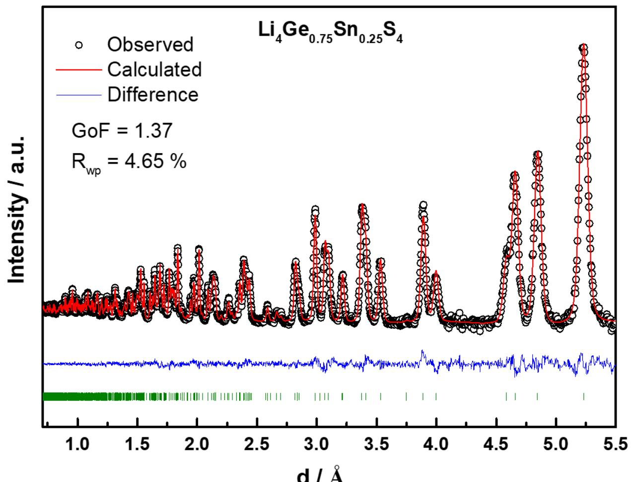
Figure S2: Neutron powder diffraction data for  $\text{Li}_4\text{Ge}_{0.75}\text{Sn}_{0.25}\text{S}_4$  and corresponding Rietveld refinement. Experimental data are shown in black and the red line denotes the calculated pattern, while the difference profile is shown in blue. Calculated positions of the Bragg reflections are shown as green vertical ticks.
