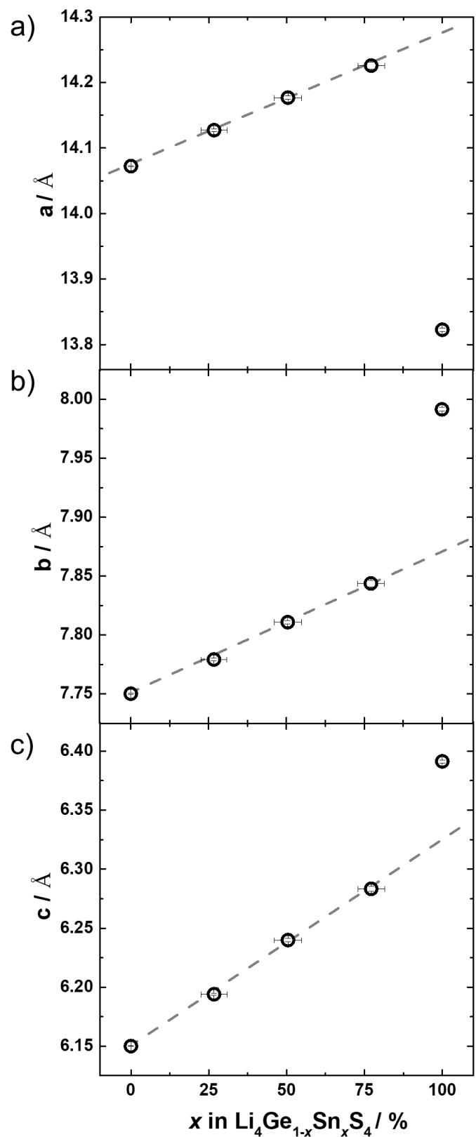
Figure S5: Lattice parameters of  $\text{Li}_4\text{Ge}_{1-x}\text{Sn}_x\text{S}_4$  against the refined Sn occupancy extracted from Rietveld refinements against neutron diffraction data.
