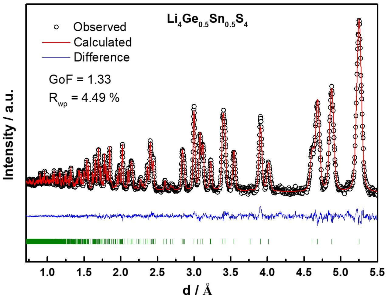
Figure S3: Neutron powder diffraction data for  $\text{Li}_4\text{Ge}_{0.5}\text{Sn}_{0.5}\text{S}_4$  and corresponding Rietveld refinement. Experimental data are shown in black and the red line denotes the calculated pattern, while the difference profile is shown in blue. Calculated positions of the Bragg reflections are shown as green vertical ticks.
