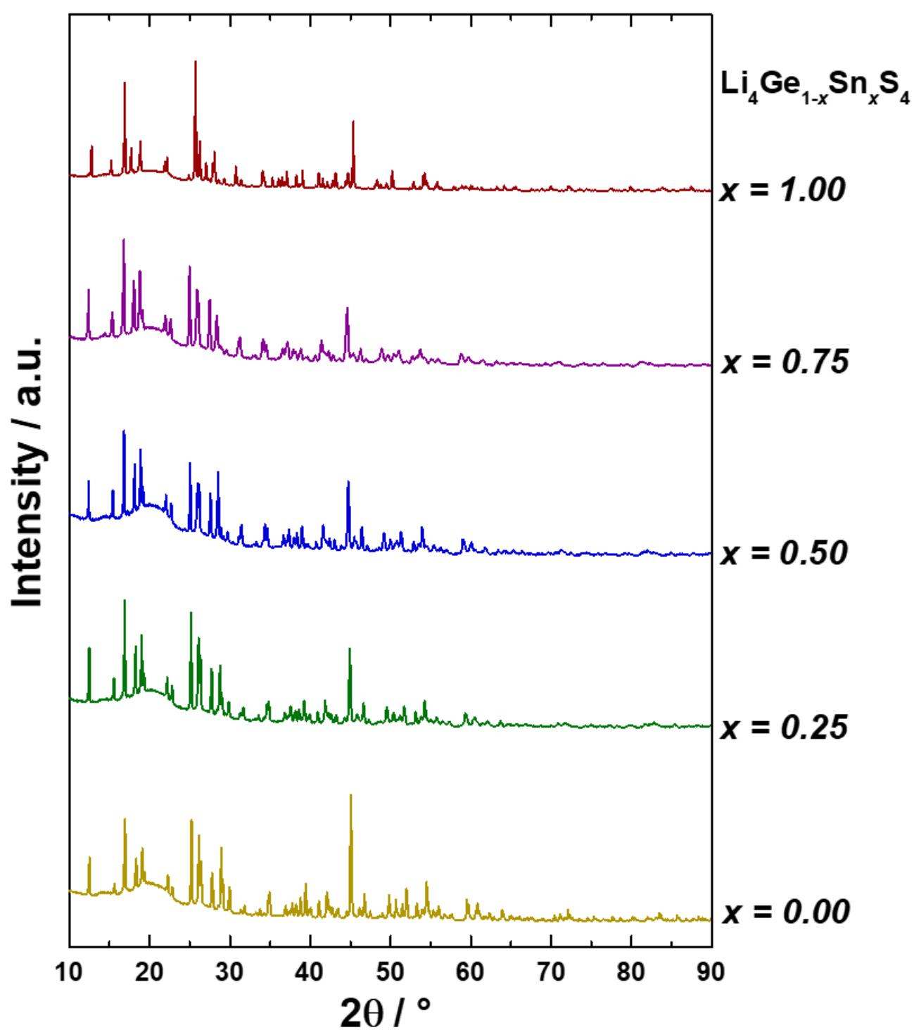
Figure S1: Laboratory X-ray powder diffractograms of  $\text{Li}_4\text{Ge}_{1-x}\text{Sn}_x\text{S}_4$ .
