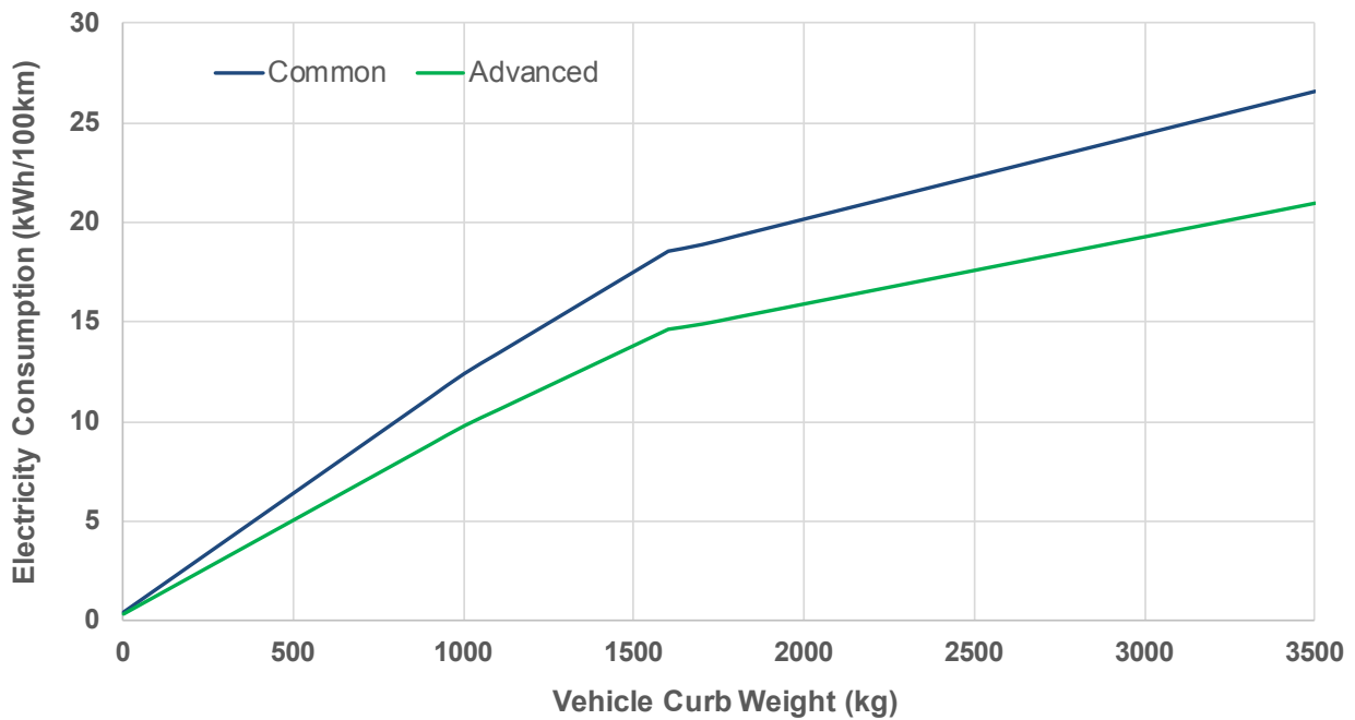
Figure S4. Vehicle electricity consumption requirement for BEVs in NEV credit policy
