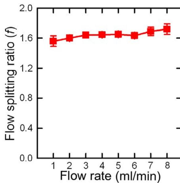
**Figure S8.** Flow splitting ratios ( $f=v_{\text{blank}}/v_{\text{target}}$ ) of our MPIM device at different flow rates of 1~8 ml/min. The  $v_{\text{blank}}$  and  $v_{\text{target}}$  are respectively the volumes of the particle-free blank fluids and the volumes of target concentrated samples.
