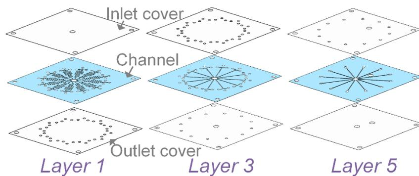
**Figure S1.** Three-sheet structure of channel layers (#1, #3, and #5) which is fabricated by enclosing the cut-through channels on the polymer film with the inlet and outlet covers.
