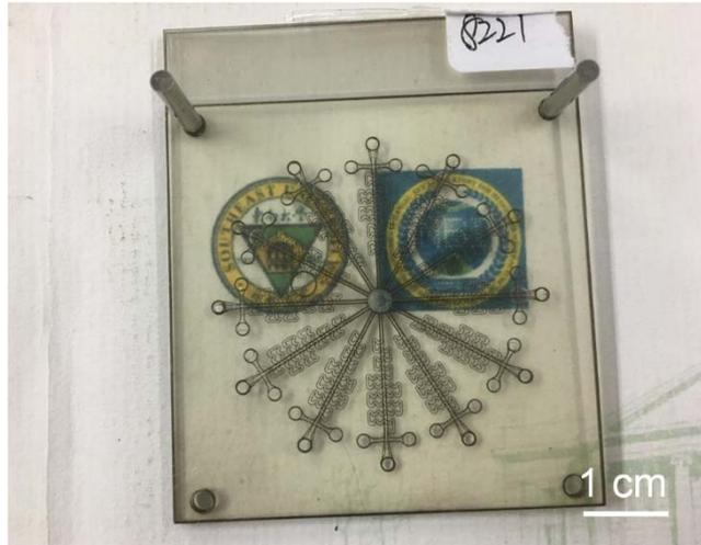
**Figure S6.** Photograph of our MPIM device showing a good optical transparency although 13 layers have been stacked in vertical direction.
