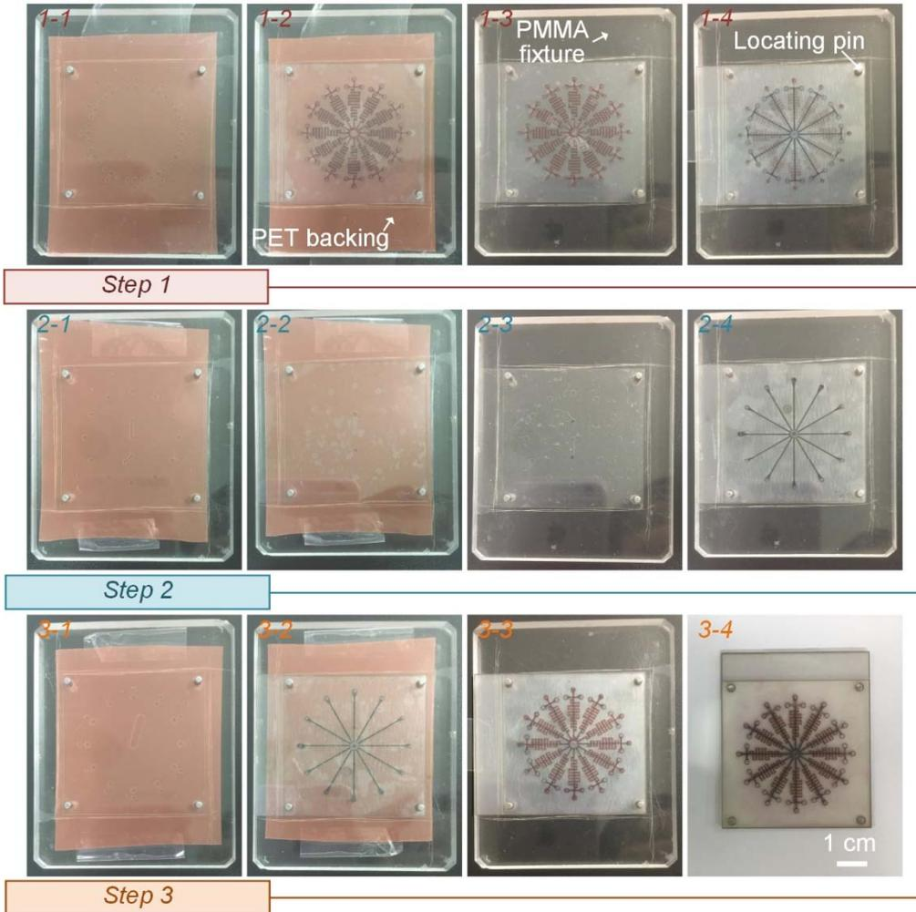
**Figure S4.** Assembly process of our MPIM device after fabricating each layer. The whole assembly process can be completed within three main steps.
