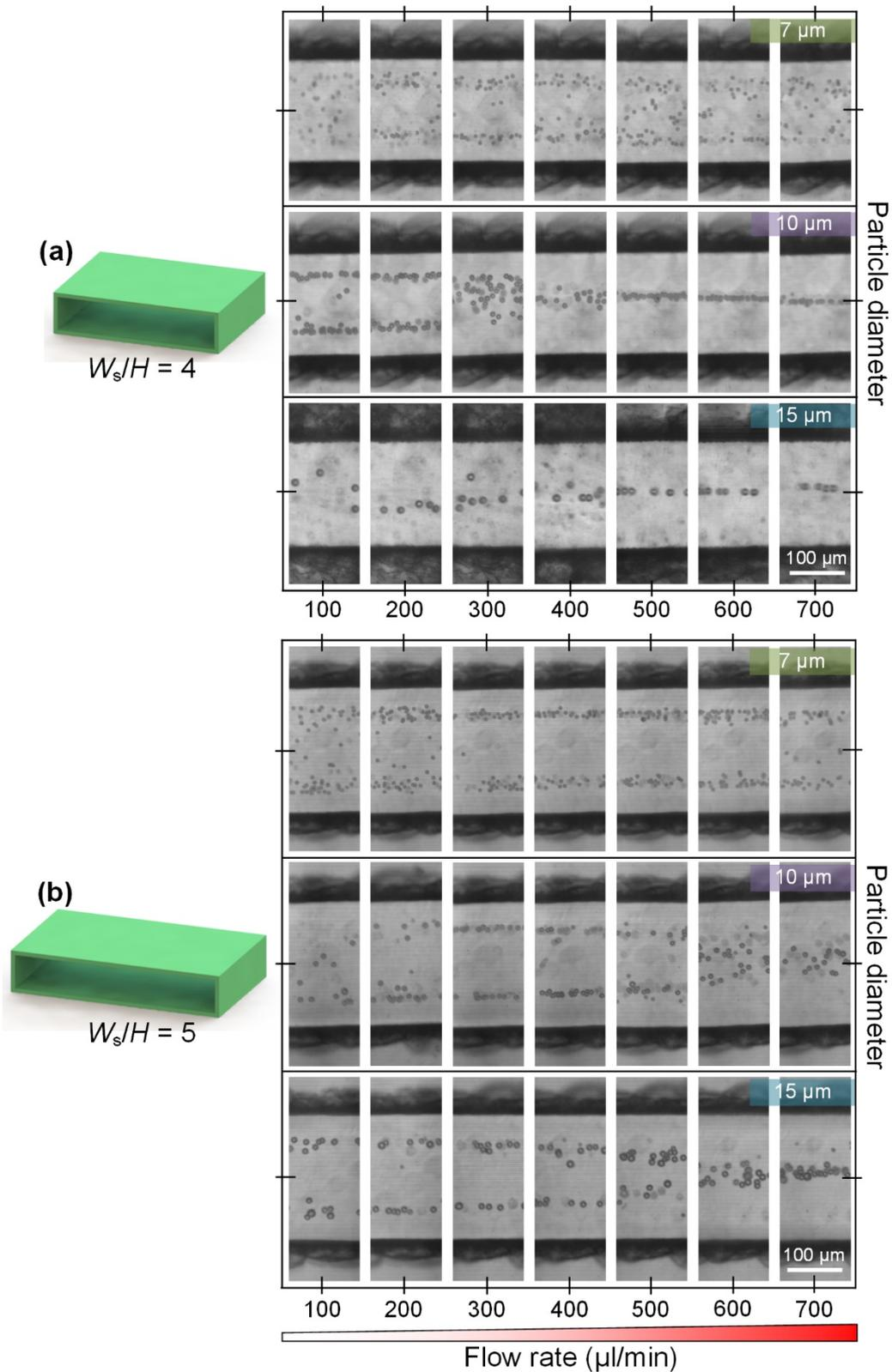
**Figure S7.** Focusing maps of 7  $\mu\text{m}$ , 10  $\mu\text{m}$  and 15  $\mu\text{m}$  particles in serpentine channels with  $W_s/H$  of 4 (a) and 5 (b) at different flow rates ranging from 100  $\mu\text{l}/\text{min}$  to 700  $\mu\text{l}/\text{min}$  (with an interval of 100  $\mu\text{l}/\text{min}$ ). The particle focusing dynamics were captured near the cross-shaped outlet.
