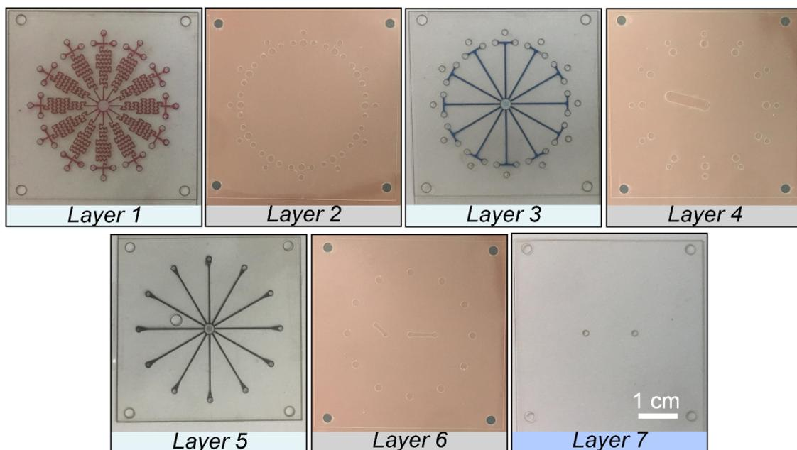
**Figure S3.** Photographs of the finished each layer. The channels were filled with ink for clear visualization. Before assembly, one side of the tape remained protected by the plastic backing (the brown film). It is worth noting that observation windows (cut-through holes) were designed on the adhesive layers at the positions before the cross-shaped outlet systems for better visualizing the cell migration in serpentine channels.
