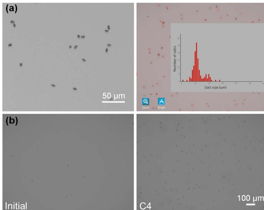
**Figure S9.** (a) Photograph and the measured size distribution of the green microalgae (GY-H1 *Platymonas helgolandica tsingtaoensis*). The average circularity of the green microalgae was measured to be  $\sim 0.5$ . (b) The microscopic images of the initial sample and the target sample collected after the C4 concentration step.
