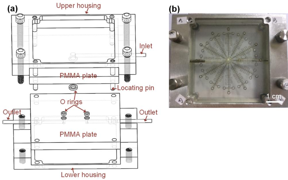
**Figure S5.** (a) Schematic diagram illustrating the structure of the housing for the chip-to-world interface. (b) Photograph of the custom housing equipped with our MPIM device.
