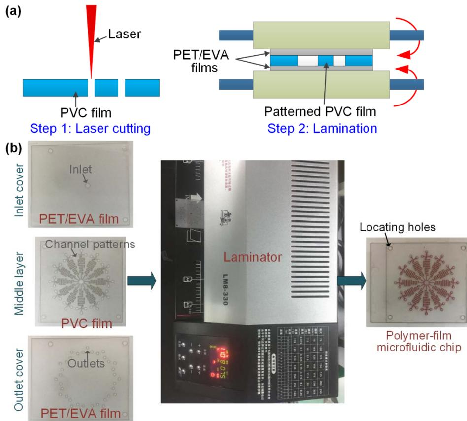
**Figure S2.** (a) Methods for fabricating the channel layers in our MPIM device. (b) Fabrication process for sealing the through channels on a polyvinyl chloride (PVC) film between two sheets of polyethylene terephthalate films with thermal sensitive ethylene-vinyl acetate copolymer (PET/EVA film) using the roll-to-roll lamination.
