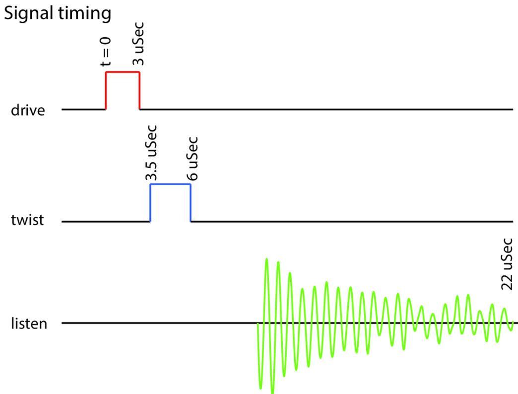
Figure S1: Timing diagram for the drive, twist, and listen pulses.
