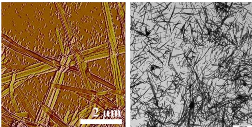
**Fig. S3.** AFM (left) and TEM (right) images of **2-S-HFIP**.
