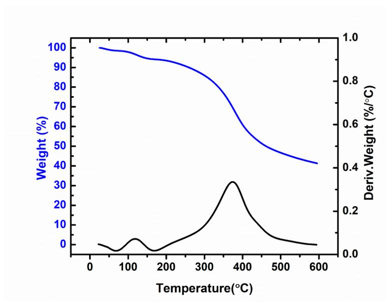
**Figure S2. TGA graph of as spun lignin fiber mat**
