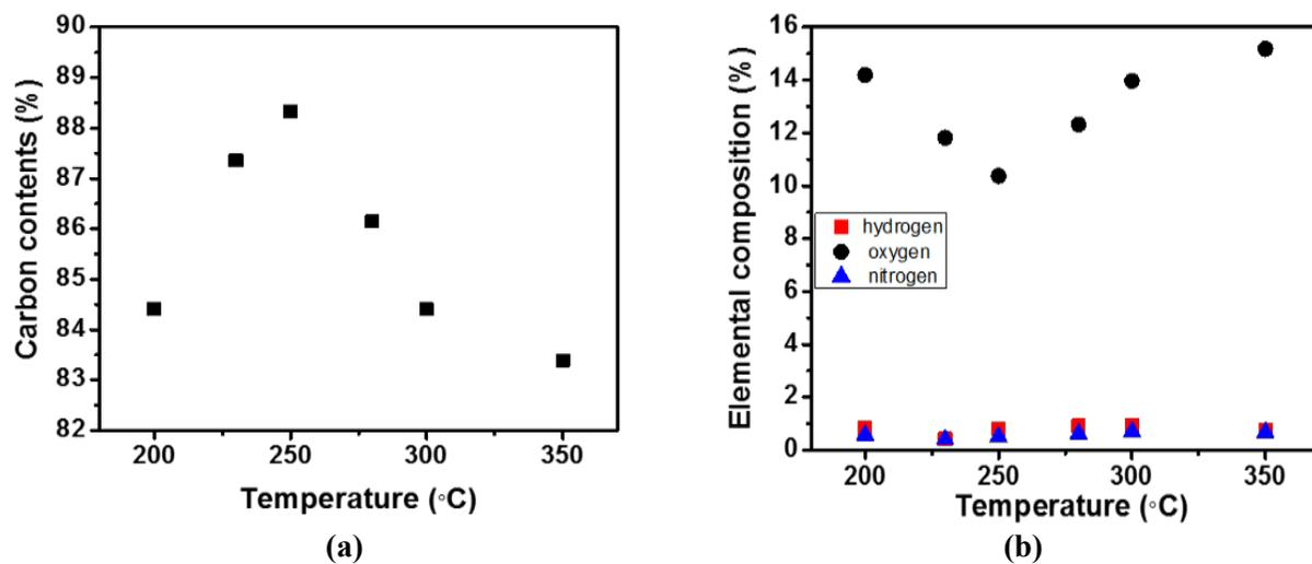
Figure S3. Elemental analysis of carbonized lignin fiber mats with different final temperatures (a) carbon content and (b) contents of hydrogen, oxygen and nitrogen.
