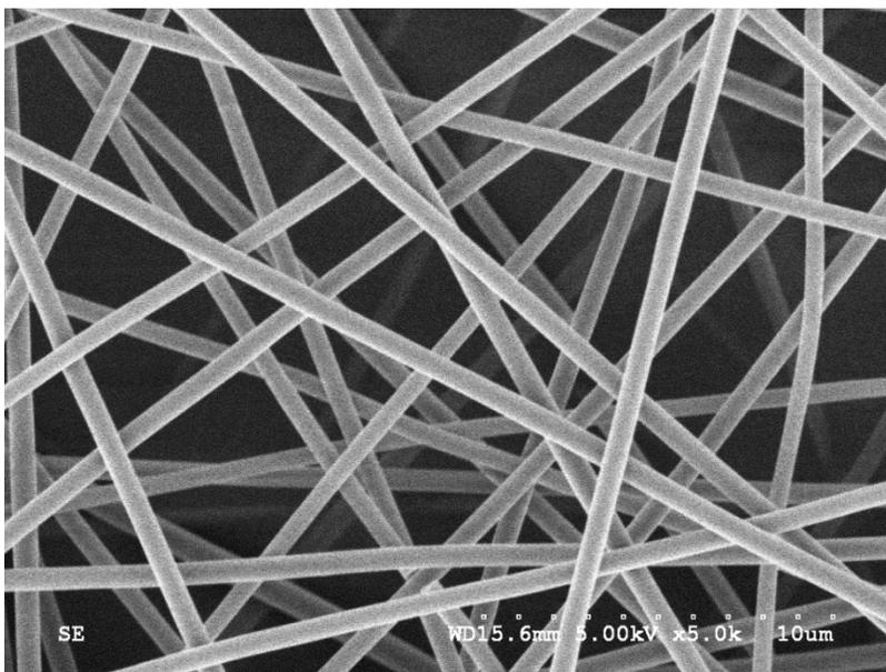
**Figure S1. SEM of electrospun lignin based nanofibers**
