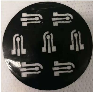
**Figure S1.** Specially designed mask for the fabrication of v-Au NWs arrays based stretchable electrode.
