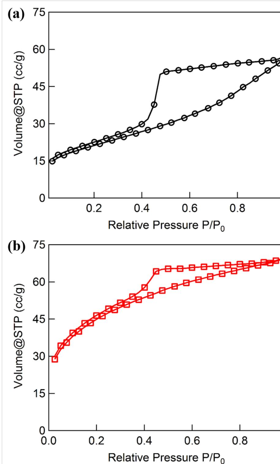
**Fig. S2.** Nitrogen adsorption-desorption isotherms of  $\text{Ni}(\text{OH})_2$  (a) and  $\text{Ni}_{0.78}\text{Fe}_{0.22}(\text{OH})_2$  (b).
