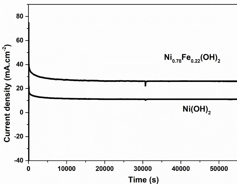
**Fig. S9.** Chronoamperometric curves of  $\text{Ni}_{0.78}\text{Fe}_{0.22}(\text{OH})_2$  and  $\text{Ni}(\text{OH})_2$  at 1.54 V (vs. RHE).
