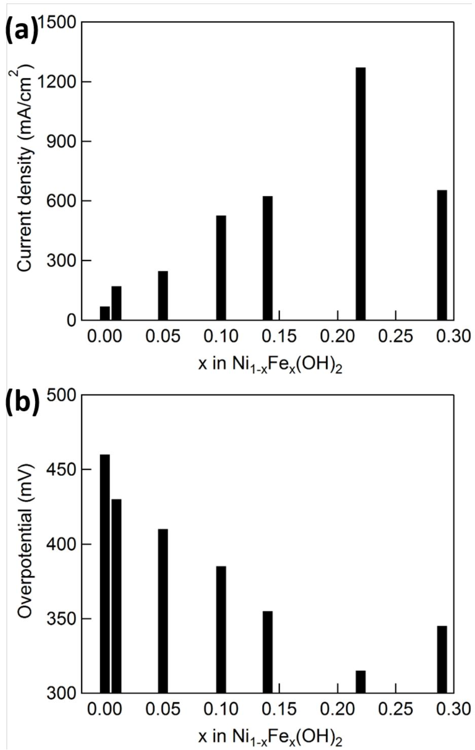
**Fig. S7.** (a) Current density at 1.8 V vs. RHE. (b) Overpotential at  $J = 10 \text{ mA}/\text{cm}^2$  of  $\text{Ni}_{1-x}\text{Fe}_x(\text{OH})_2$  ( $x = 0, 0.01, 0.05, 0.11, 0.14, 0.22, 0.29$ ) loaded on RDE (2000 rpm) in 1.0 M purified KOH, scan rate = 5 mV/s.
