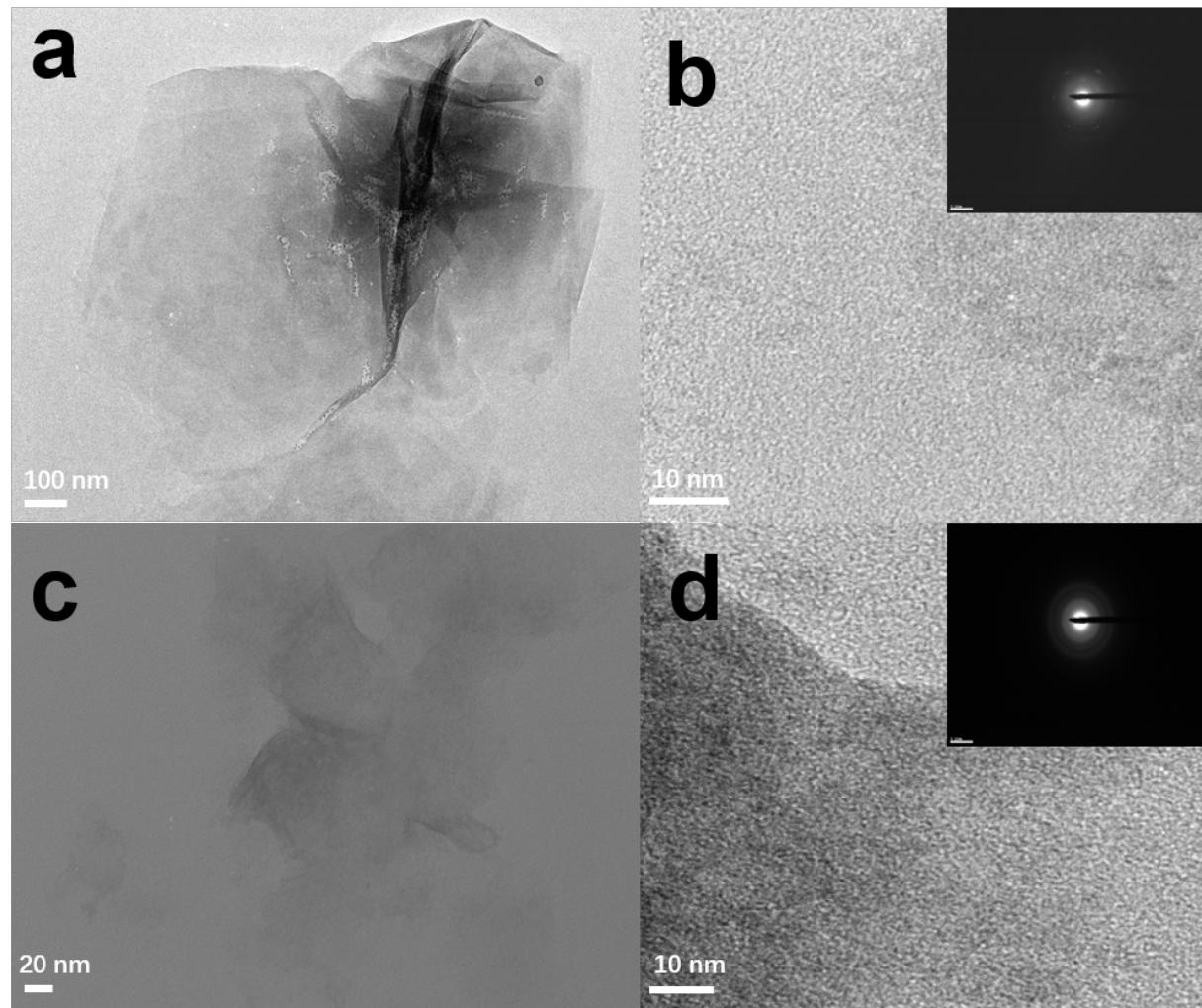
**Fig. S4.** TEM images of (a-b)  $\text{Ni}(\text{OH})_2$  (inset is the SAED pattern), (c-d)  $\text{Ni}_{0.78}\text{Fe}_{0.22}(\text{OH})_2$  (inset is the SAED pattern).
