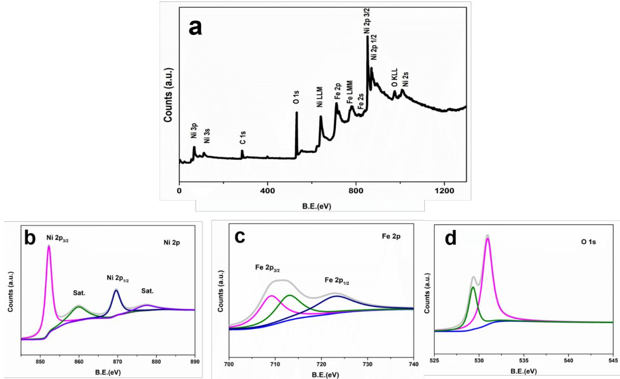
**Fig. S6.** XPS spectra of  $\text{Ni}_{0.78}\text{Fe}_{0.22}(\text{OH})_2$ : survey (a) and the spectral regions of Ni 2p (b), Fe 2p (c) and O 1s (d).
