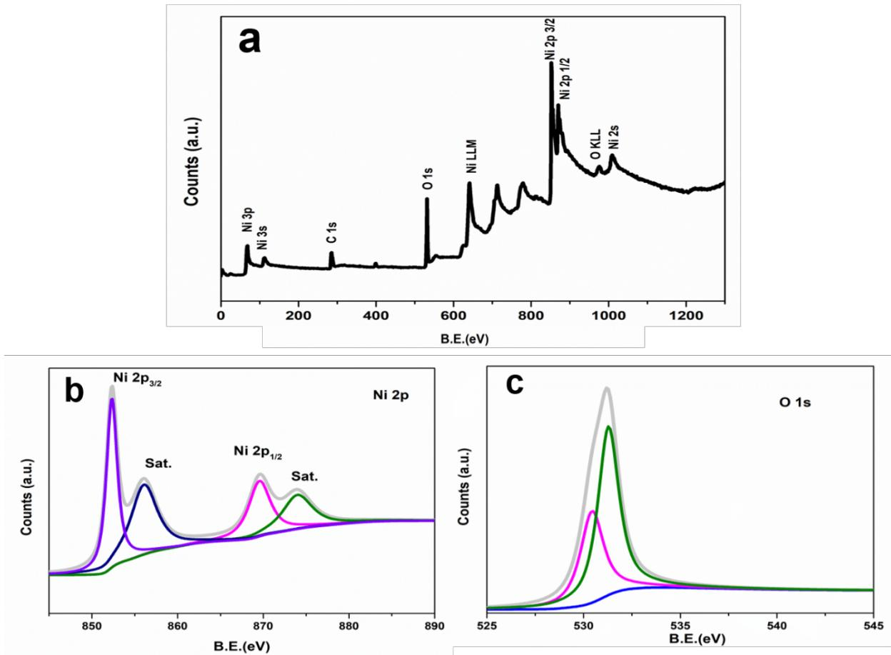
**Fig. S5.** XPS spectra of  $\text{Ni}(\text{OH})_2$ : survey (a) and the spectral regions of Ni 2p (b) and O 1s (c).
