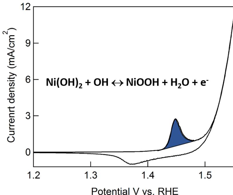
**Fig. S8.** Cyclic voltammetry of  $\text{Ni}_{0.78}\text{Fe}_{0.22}(\text{OH})_2$  in 1.0 M KOH with scan rate 10 mV/s.
