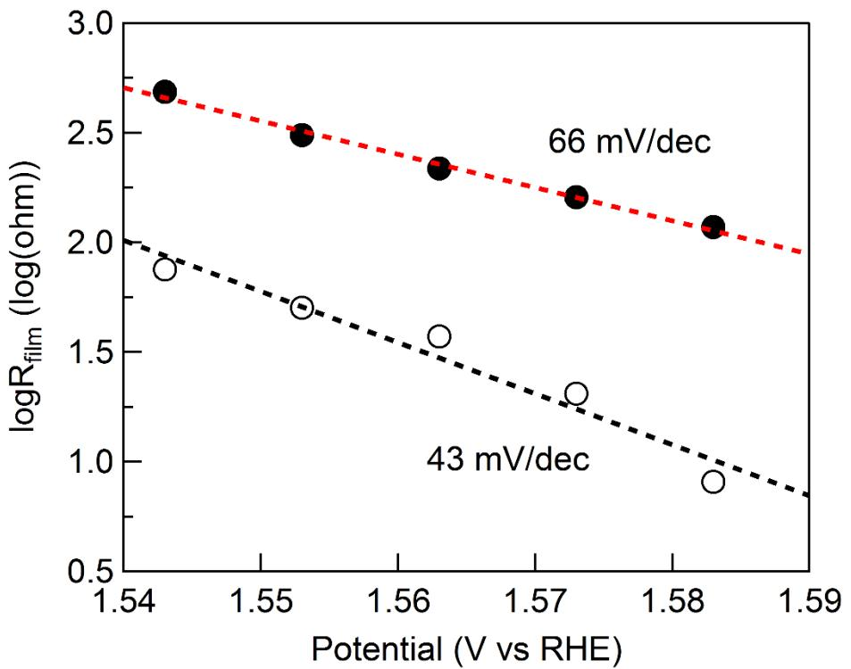
**Fig. S11.** Catalyst film resistance ( $R_{\text{film}}$ )-based Tafel plots derived from the EIS fitting results of  $\text{Ni(OH)}_2$  (black) and  $\text{Ni}_{0.78}\text{Fe}_{0.22}(\text{OH})_2$  (white).
