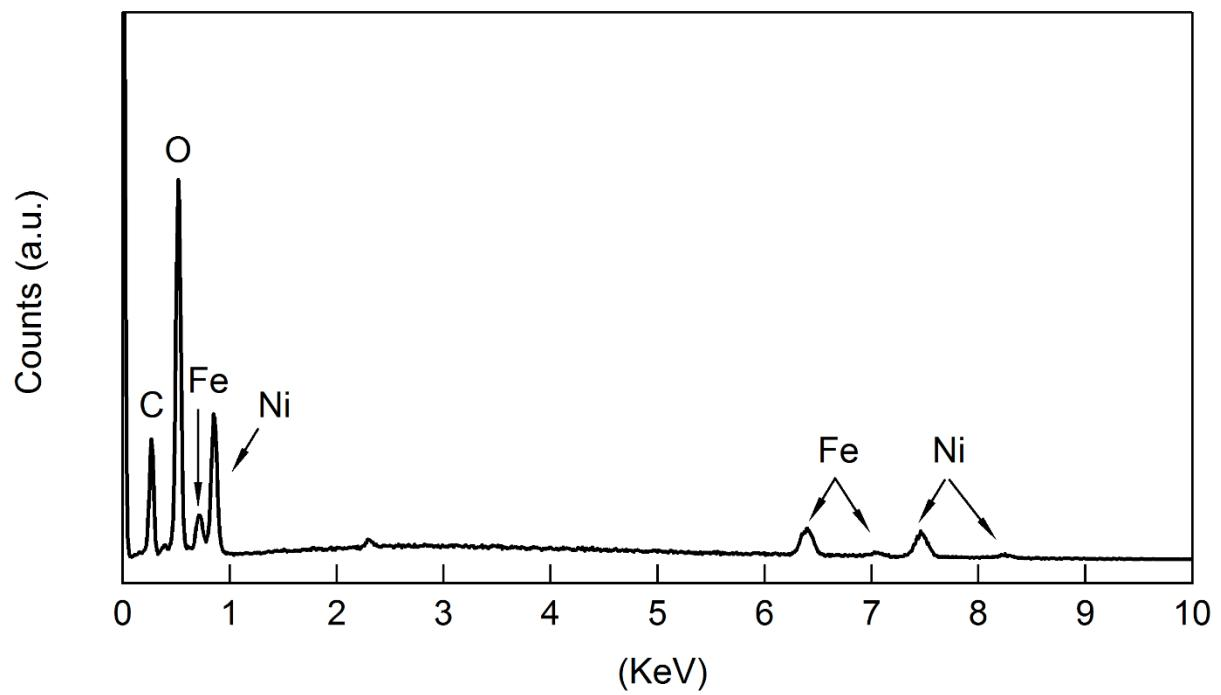
**Fig. S3.** Energy-dispersive X-ray spectrum of  $\text{Ni}_{0.78}\text{Fe}_{0.22}(\text{OH})_2$ .
