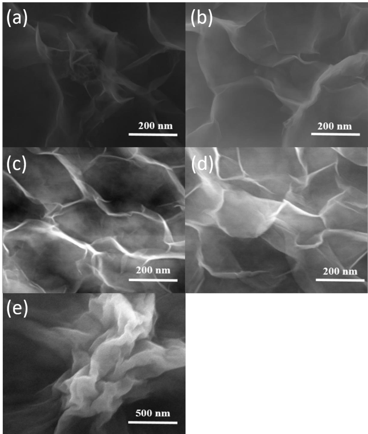
**Fig. S1.** SEM images of (a)  $\text{Ni}_{0.99}\text{Fe}_{0.01}(\text{OH})_2$ , (b)  $\text{Ni}_{0.95}\text{Fe}_{0.05}(\text{OH})_2$ , (c)  $\text{Ni}_{0.89}\text{Fe}_{0.11}(\text{OH})_2$ , (d)  $\text{Ni}_{0.84}\text{Fe}_{0.14}(\text{OH})_2$ , (e)  $\text{Ni}_{0.71}\text{Fe}_{0.29}(\text{OH})_2$ .
