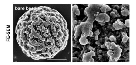
Figure S3. FE-SEM image of bare beads. Streptavidin coated beads have nano-grooves. Scale bar:
