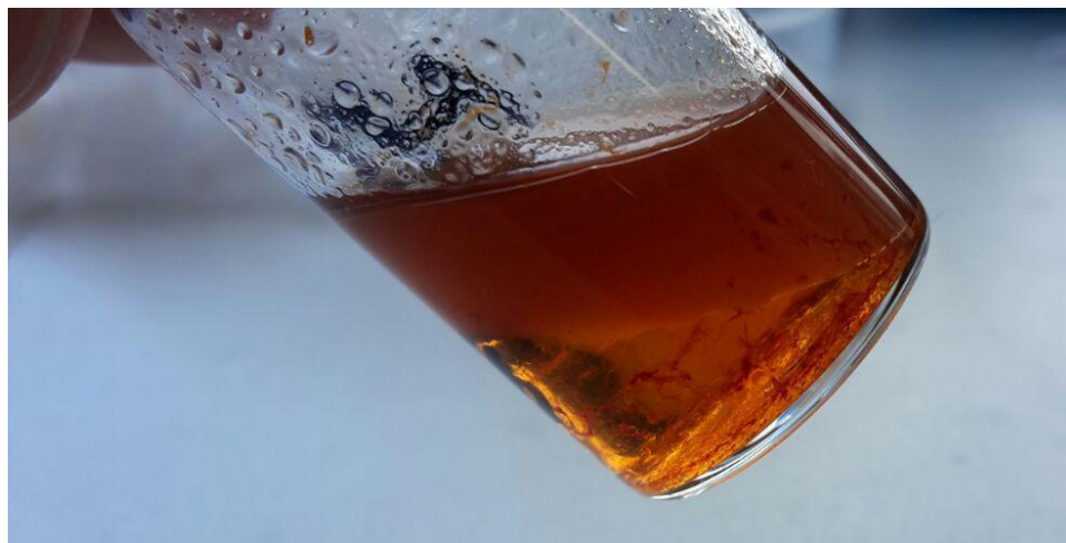
Figure S23. Positive Angeli-Rimini 2 chemical test of aldehyde functional PEG. The red-colored hydroxamic acid complexes could be partly transferred to the bottom dichloromethane layer.
