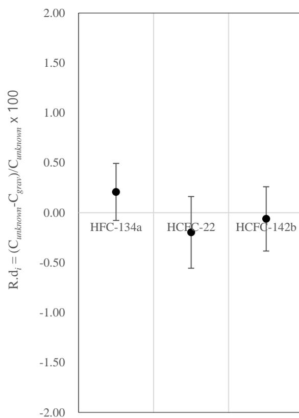
**Figure S9.** Difference between the calibrated concentration ( $C_{unknown}$ ) and the gravimetrically assigned concentration ( $C_{grav}$ ).  $C_{unknown}$  is calculated as 66.81, 218.65 and 21.90 pmol/mol for HFC-134a, HCFC-22 and HCFC-142b, respectively. New result shows better verification uncertainty compared to that of CCQM-K84 of which part were conducted by KRISS.
