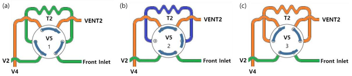
**Figure S1.** Gas flow pathways of V5. The position coordinates (1 or 2 or 3) given underneath of the symbol V5 correspond to (a), (b), and (c), respectively. For eye guide, connected lines are identically colored.
