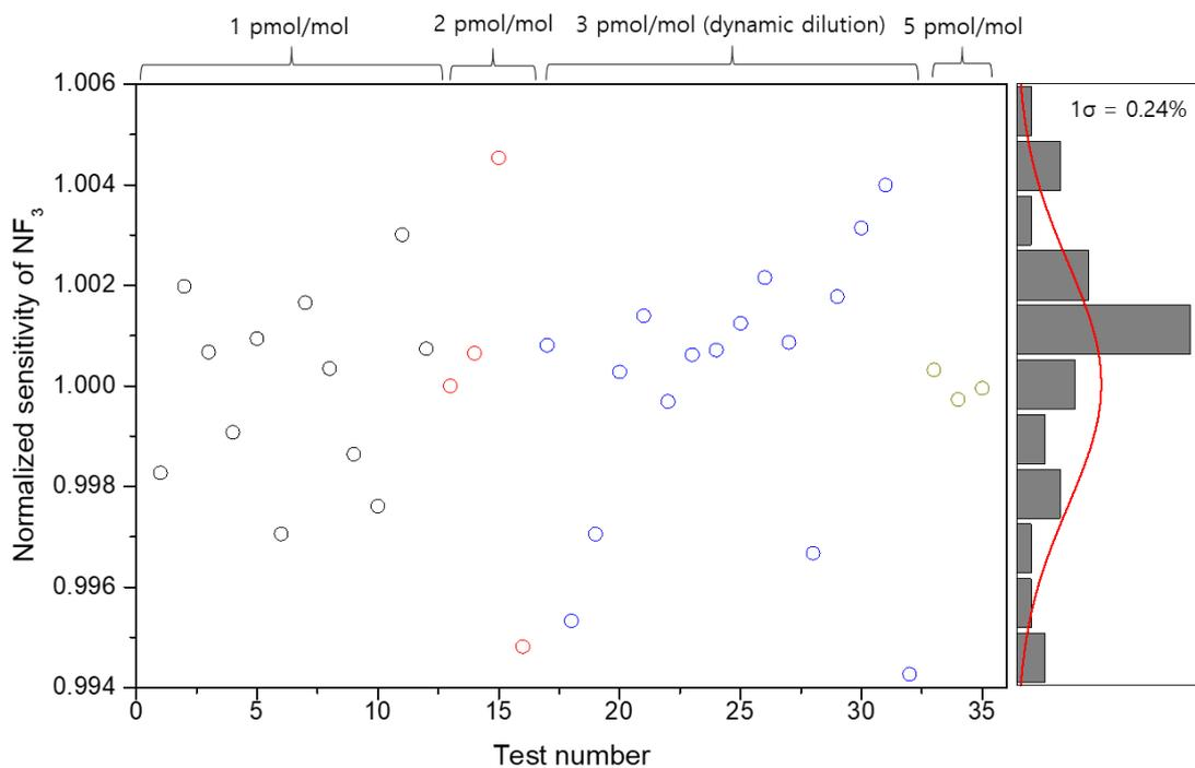
**Figure S6.** Precision test of  $\text{NF}_3$  measurement. Gravimetric gas mixtures of 1 pmol/mol, 2 pmol/mol, and 5 pmol/mol  $\text{NF}_3$  in synthetic air were measured. Results at 3 pmol/mol were given by dynamic dilution of 5 pmol/mol  $\text{NF}_3$ /air gas mixture by high purity  $\text{N}_2$  (> 99.999%) by adjusting ratio of flow rates, implying that measurement uncertainty includes uncertainty of flow rates. Overall precision was evaluated to be less than 0.35% ( $1\sigma$ )
