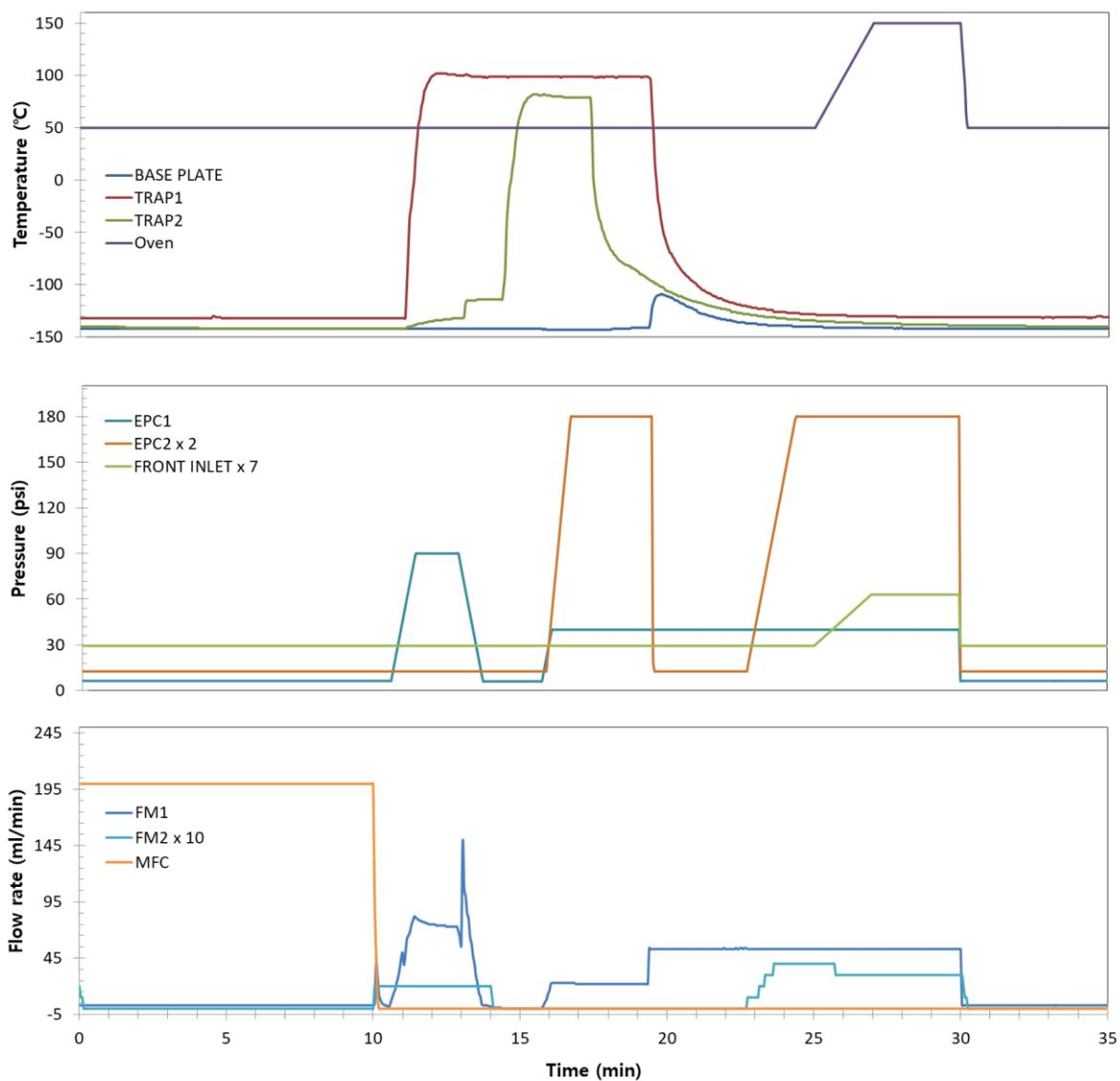
**Figure S4.** Strip chart of  $\text{NF}_3$  in  $\text{CO}_2$  free synthetic air measurement procedure. When the balance gas is pure nitrogen, it is not necessary to consider  $\text{CO}_2$ , so the temperature is raised to  $100^\circ\text{C}$  when transferring from T1 to T2. Applying this condition reduces the transfer time, and the time to cool down to a temperature where it is again possible to concentrate is shortened, allowing measurement in a shorter time per cycle.
