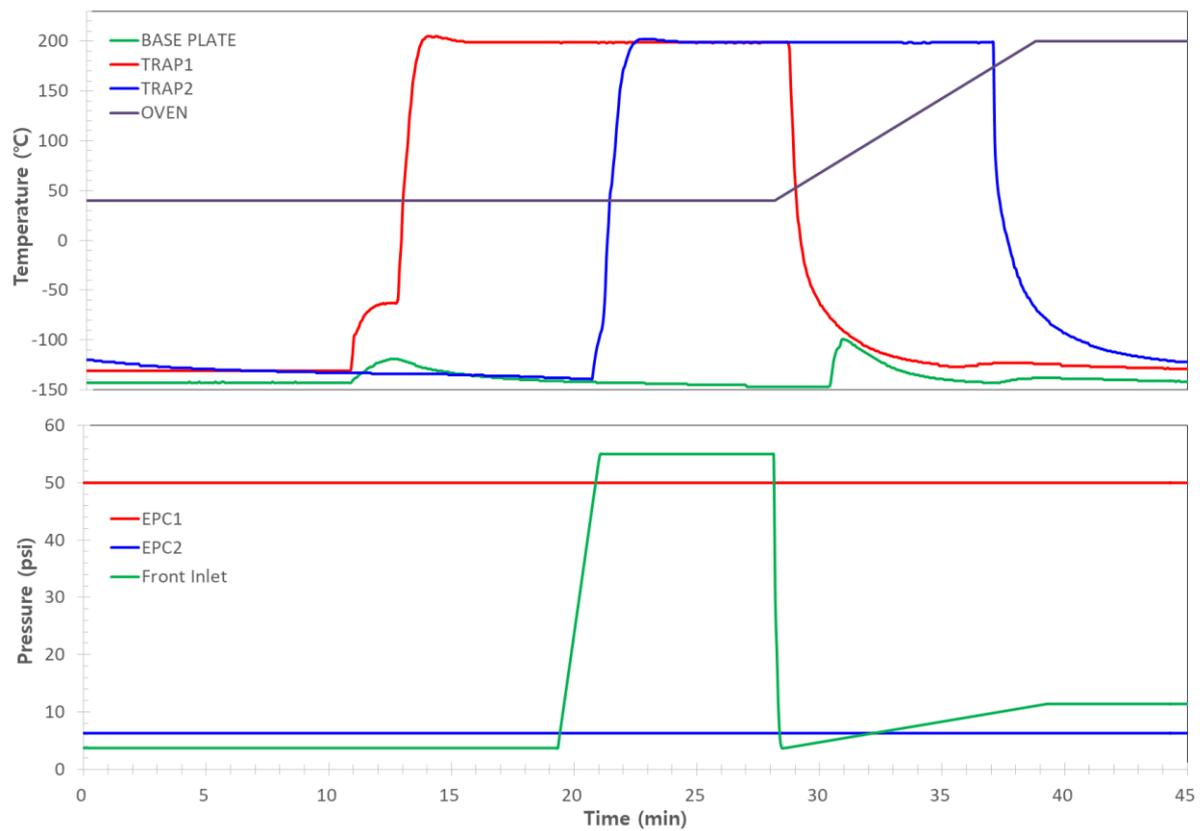
**Figure S3.** Strip chart of HFCs measurement procedure. Compared with  $\text{NF}_3$  analysis, the retaining time in Step 8, which is the preparation step for injection, is longer.
