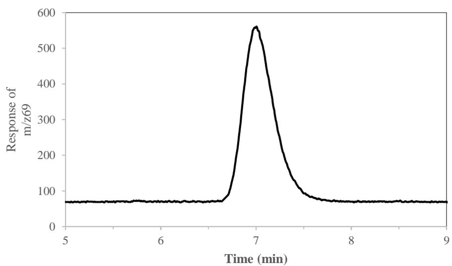
**Figure S10.** Chromatogram of  $\text{CF}_4$ . The retention time and peak shape are different from those under the conditions described in the main section due to non-identical analytical condition described in the main text. Only separation condition was changed.
