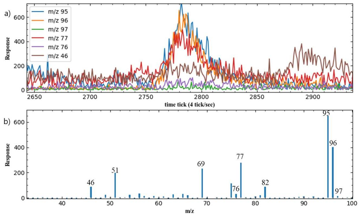
**Figure S13.** a) Combined chromatogram of HFO-1234zf at various m/z levels denoted in the legend, b) mass spectrum obtained at the peak around 2600 time ticks, which shows over 90% Q factor with the NIST mass spectroscopy library.
