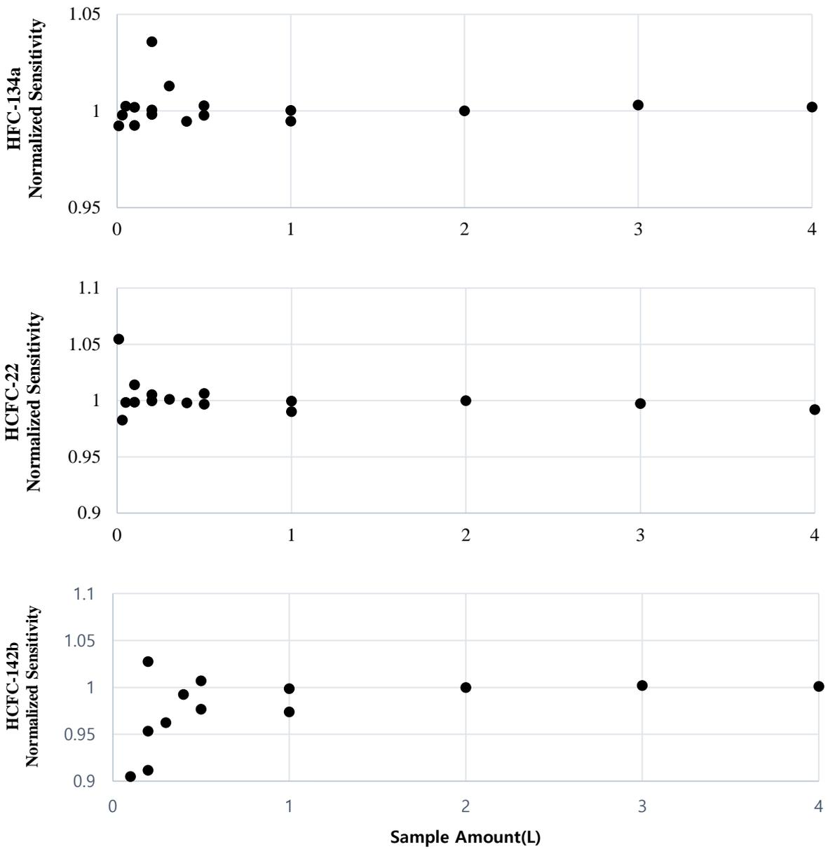
**Figure S7.** Response linearities of HFCs. The result obtained by dividing the value obtained from the response by the sample volume is sensitivity, and each value was divided based on the sensitivity of 2L and normalized. Sampling time was adjusted with sampling flow of 200ml/min when measuring 0.5L or more, while sampling time was adjusted with sampling flow of 60ml/min when measuring less than 0.5L.
