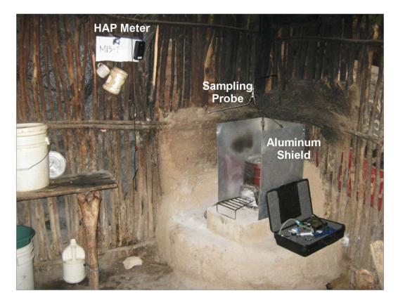
Figure S1. Stove emissions sampling configuration.
