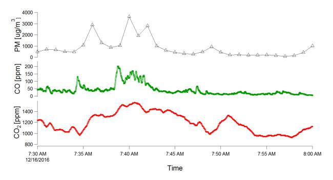
**Figure S2.** Resolution of HAP data. PM concentration was recorded once per minute while CO and CO<sub>2</sub> concentrations were recorded once per second.
