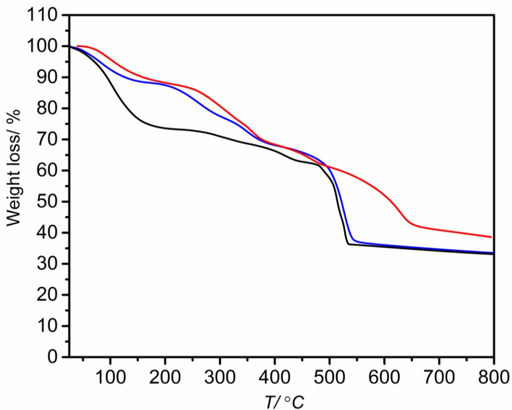
Figure S4. TGA data of **1**\_EG (red line), **2**\_EG (blue line) and **3**\_EG (black line)
