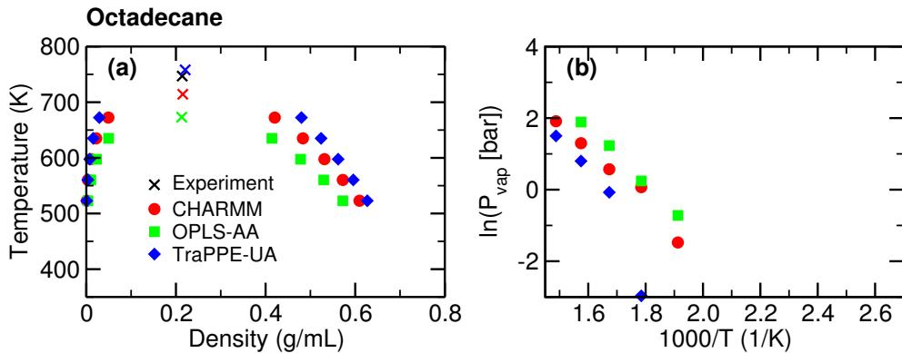
Figure S4: Vapor-liquid coexistence curves (a) and vapor pressures (b) for *n*-octadecane obtained using CHARMM, OPLS-AA, and TraPPE-UA. Experimental data obtained from the NIST webbook.<sup>1</sup>
