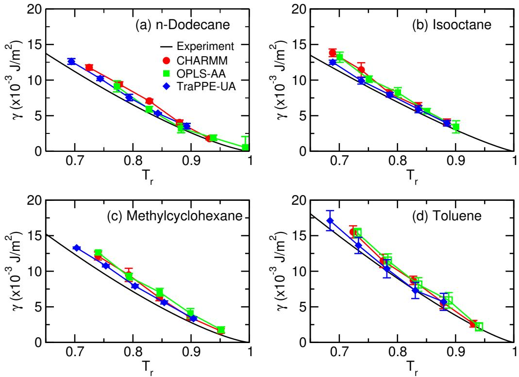
Figure S14: Surface tension,  $\gamma$ , of *n*-dodecane (**a**), isoctane (**b**), methylcyclohexane (**c**), and toluene (**d**) as a function of reduced temperature,  $T_r$ .  $T_r$  is the temperature normalized by the corresponding  $T_c$ . Experimental data plotted using Eqn. 7 from the main text, with constants obtained from Ref. 2.
