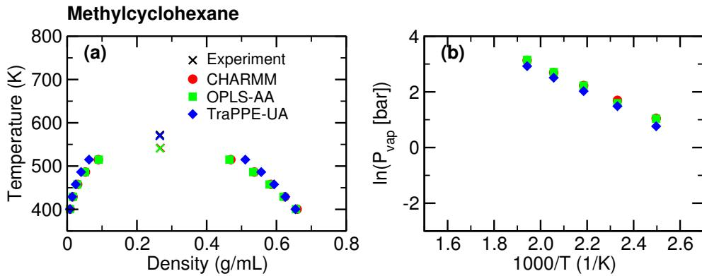
Figure S7: Vapor-liquid coexistence curves **(a)** and vapor pressures **(b)** for methylcyclohexane obtained using CHARMM, OPLS-AA, and TraPPE-UA. Experimental data obtained from the NIST webbook.<sup>1</sup>
