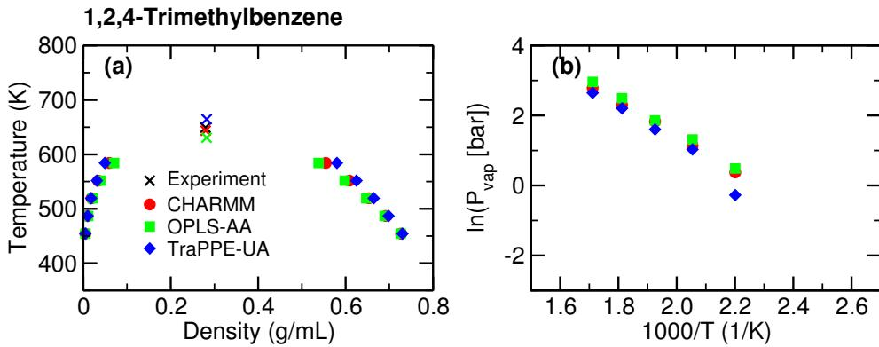
Figure S10: Vapor-liquid coexistence curves **(a)** and vapor pressures **(b)** for 1,2,4-trimethylbenzene obtained using CHARMM, OPLS-AA, and TraPPE-UA. Experimental data obtained from the NIST webbook.<sup>1</sup>
