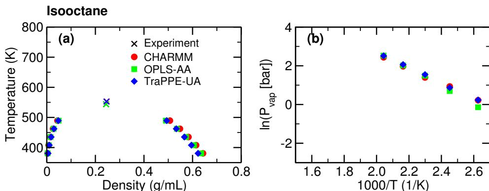
Figure S5: Vapor-liquid coexistence curves (a) and vapor pressures (b) for isoctane obtained using CHARMM, OPLS-AA, and TraPPE-UA. Experimental data obtained from the NIST webbook.<sup>1</sup>
