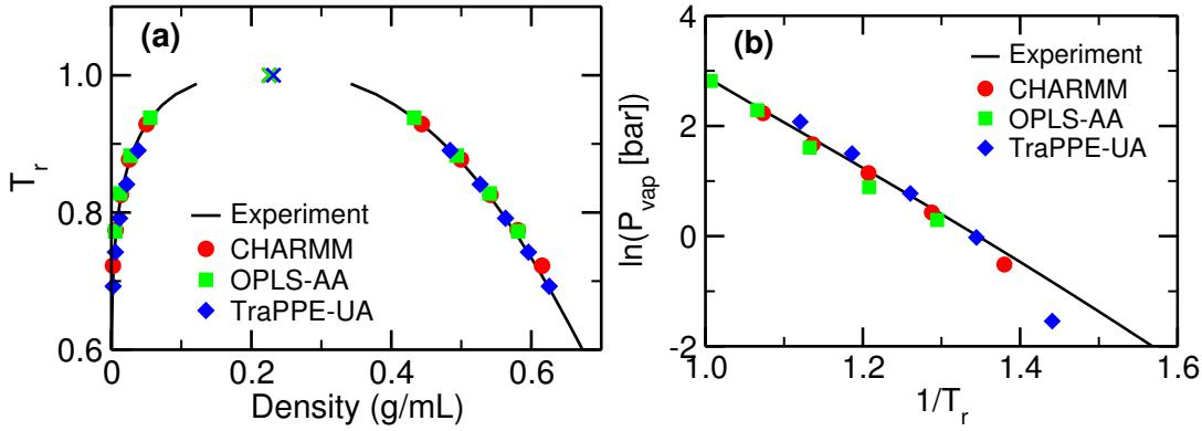
Figure S1: Vapor-liquid coexistence curves (a) and vapor pressures (b) for *n*-dodecane obtained using CHARMM, OPLS-AA, and TraPPE-UA. Experimental data obtained from the NIST webbook.<sup>1</sup>  $T_r$  is the temperature normalized by the corresponding  $T_c$ .
