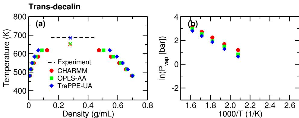
Figure S8: Vapor-liquid coexistence curves **(a)** and vapor pressures **(b)** for trans-decalin obtained using CHARMM, OPLS-AA, and TraPPE-UA. Experimental data obtained from the NIST webbook.<sup>1</sup>
