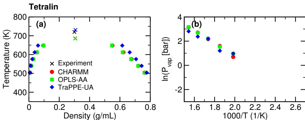
Figure S11: Vapor-liquid coexistence curves **(a)** and vapor pressures **(b)** for tetralin obtained using CHARMM, OPLS-AA, and TraPPE-UA. Experimental data obtained from the NIST webbook.<sup>1</sup>
