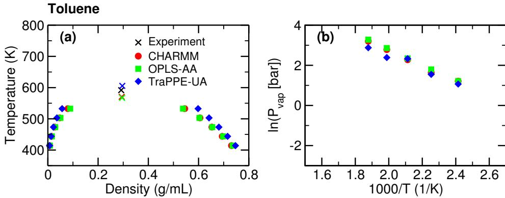
Figure S9: Vapor-liquid coexistence curves **(a)** and vapor pressures **(b)** for toluene obtained using CHARMM, OPLS-AA, and TraPPE-UA. Experimental data obtained from the NIST webbook.<sup>1</sup>
