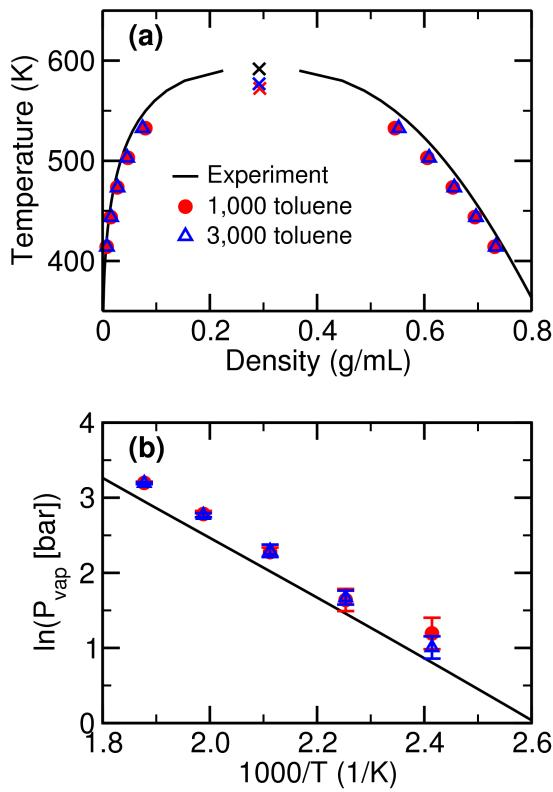
Figure S13: Vapor-liquid coexistence curves (a) and vapor pressures (b) for toluene simulated using CHARMM. The 3,000 molecule systems were generated by tripling both the thickness of the initial slab as well as the length of the  $z$ -axis.
