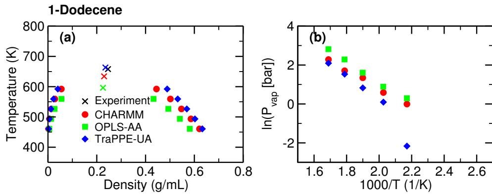
Figure S2: Vapor-liquid coexistence curves (a) and vapor pressures (b) for 1-dodecene obtained using CHARMM, OPLS-AA, and TraPPE-UA. Experimental data obtained from the NIST webbook.<sup>1</sup>
