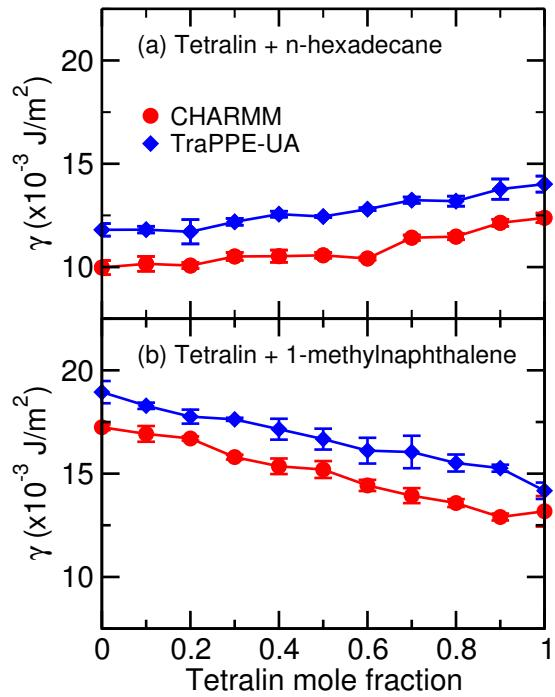
Figure S16: Surface tension  $\gamma$  as a function of composition for binary mixtures of tetralin with *n*-hexadecane (**a**) or 1-methylnaphthalene (**b**) at 523.15 K.
