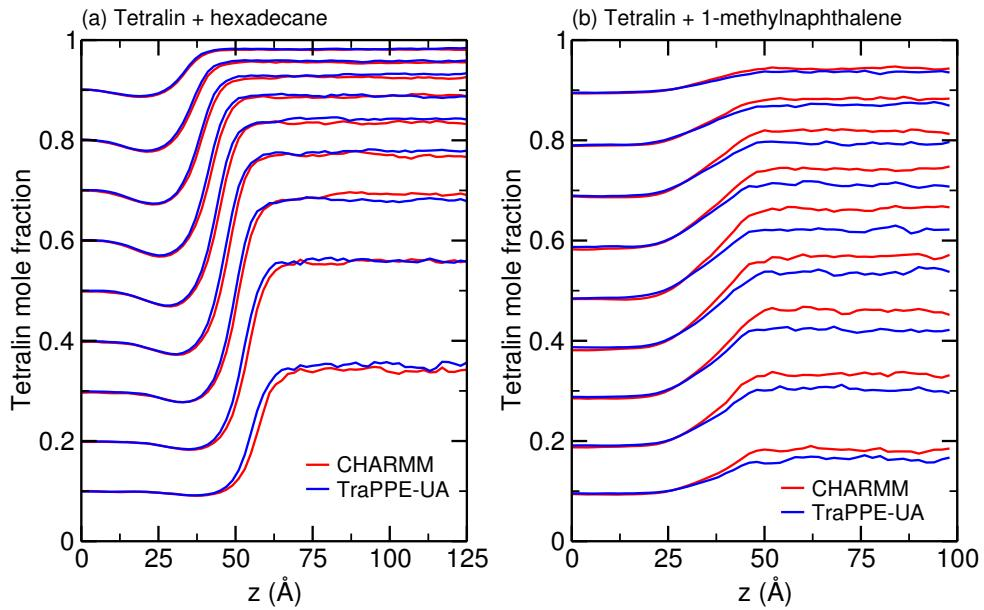
Figure S15: Tetralin mole fraction as a function of distance from liquid slab center of mass for binary mixtures of tetralin with *n*-hexadecane (**a**) or 1-methylnaphthalene (**b**) at 523.15 K. System compositions range from 0.1 to 0.9 mole fraction tetralin moving from bottom to top.
