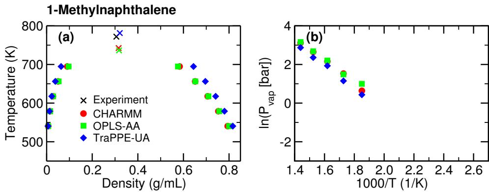
Figure S12: Vapor-liquid coexistence curves (a) and vapor pressures (b) for 1-methylnaphthalene obtained using CHARMM, OPLS-AA, and TraPPE-UA. Experimental data obtained from the NIST webbook.<sup>1</sup>
