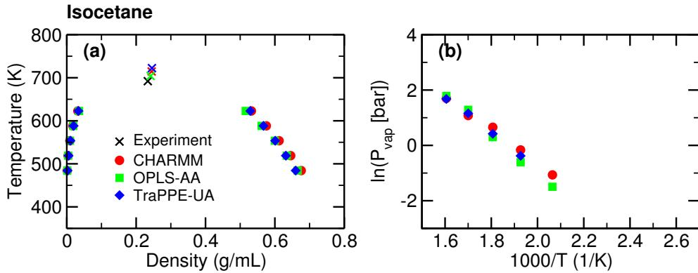
Figure S6: Vapor-liquid coexistence curves **(a)** and vapor pressures **(b)** for isocetane obtained using CHARMM, OPLS-AA, and TraPPE-UA. Experimental data obtained from the NIST webbook.<sup>1</sup>
