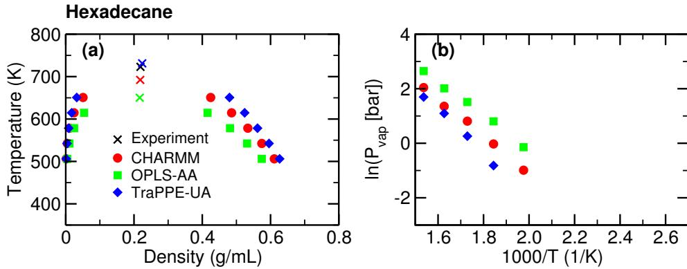
Figure S3: Vapor-liquid coexistence curves (a) and vapor pressures (b) for *n*-hexadecane obtained using CHARMM, OPLS-AA, and TraPPE-UA. Experimental data obtained from the NIST webbook.<sup>1</sup>
