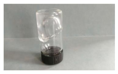
Fig. S1.Photo of the as-prepared quasi-solid-state gel electrolyte.
