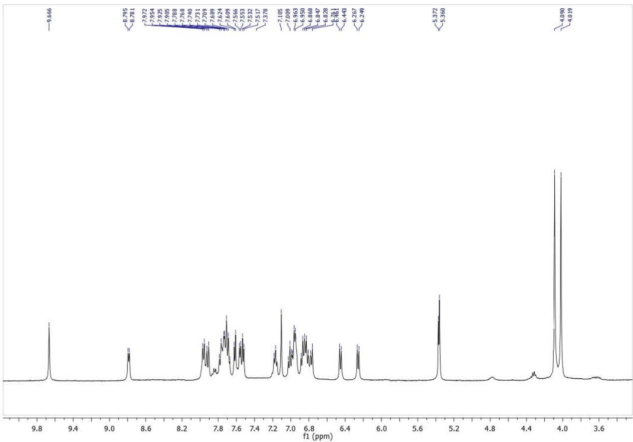
**Figure S3.**  $^1\text{H}$  NMR spectrum ( $\text{CD}_2\text{Cl}_2$ , expansion of the aromatic protons region) of a *cis*-**5** enriched fraction obtained from liquid chromatography of the reaction mixture for iridium(III) complex preparation.
