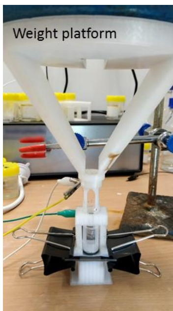
Figure S2. Small-scale electrochemical cell used to oxidize 40-750 mg flake graphite.
