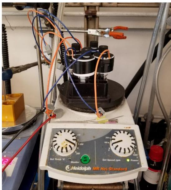
**Figure S1.** Picture of 4 electrochemical cells connected in series.
