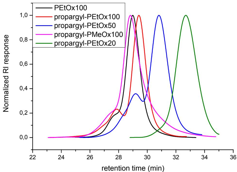
**Figure S10: SEC overlay for the different polymers. The double molar mass shoulders at lower retention times can be attributed to chain transfer followed by chain coupling as commonly observed for the polymerization of 2-oxazoline monomers at 140°C.**
