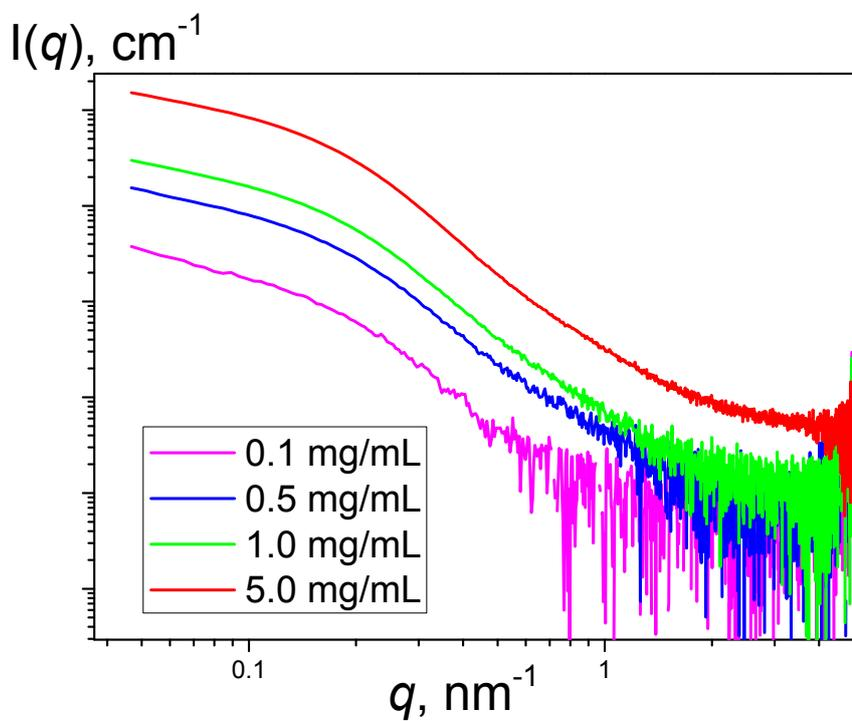
**Figure S9: SAXS data for different concentrations for molar C<sub>60</sub>:alkyne-PEtOx DP100 molar ratio 0.5:1 .**
