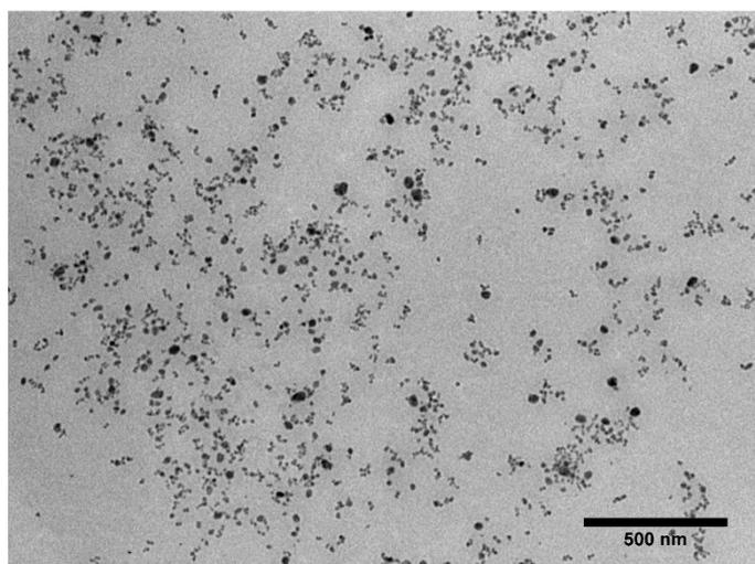
**Figure S13: TEM images of C<sub>60</sub> NPs with PEtOx DP 100 for 0.5:1 (top), 1:1 (middle) and 2:1 (bottom) molar ratio of (C<sub>60</sub>:PAOx).**
