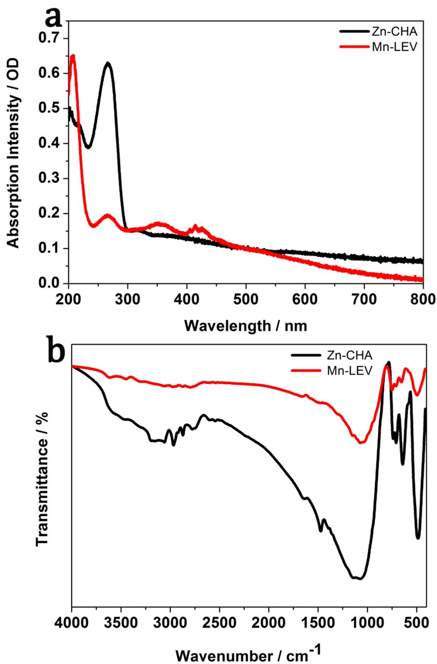
**Figure S7.** a) UV-vis absorption spectra and b) FTIR spectra of CDs@Mn-LEV and CDs@Zn-CHA composites.
