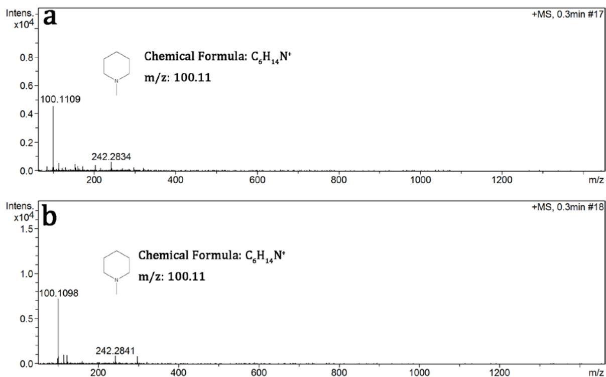
**Figure S2.** LC-HRMS of dissolved CDs@zeolite composites: a) CDs@Mn-LEV and b) CDS@Zn-CHA.
