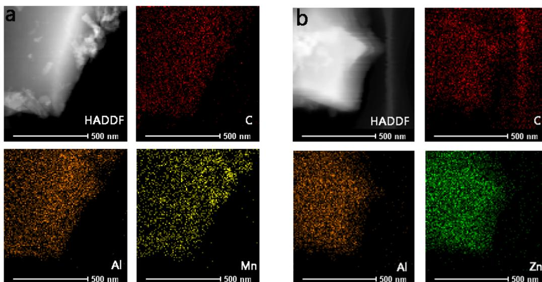
**Figure S3.** TEM mappings and HADDF STEM images of a) CDs@Mn-LEV and b) CDs@Zn-CHA.
