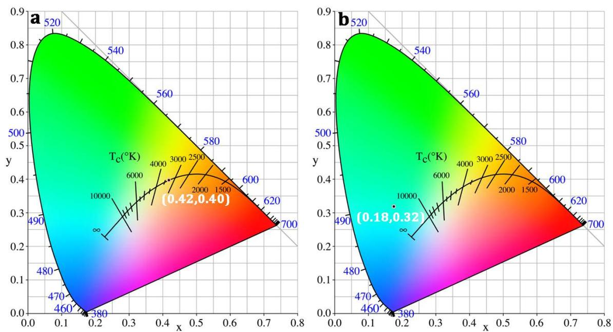
**Figure S5.** The CIE color coordinates of (a) CDs@Mn-LEV and (b) CDs@Zn-CHA composites.
