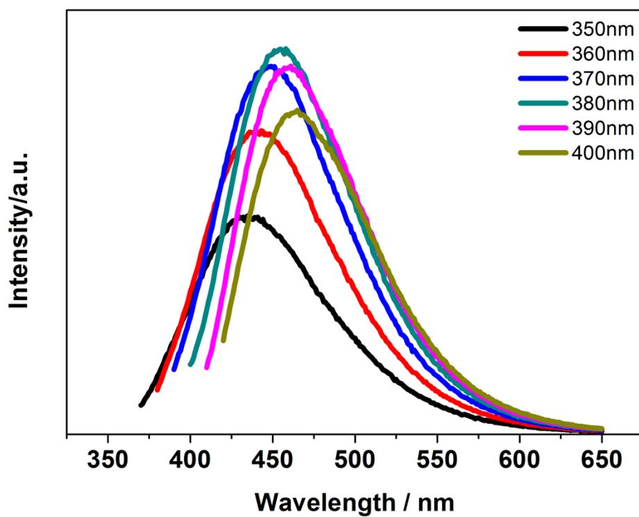
**Figure S9.** Fluorescence emission spectra of CDs@Zn-LEV mother solution under different excitation wavelength.
