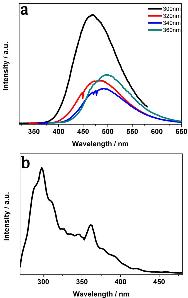
**Figure S10.** a) low temperature (77K) phosphorescence spectra of mother solution of CDs@Mn-LEV under different excitation; b) low temperature (77K) phosphorescence excitation spectrum of mother solution of CDs@Mn-LEV.
