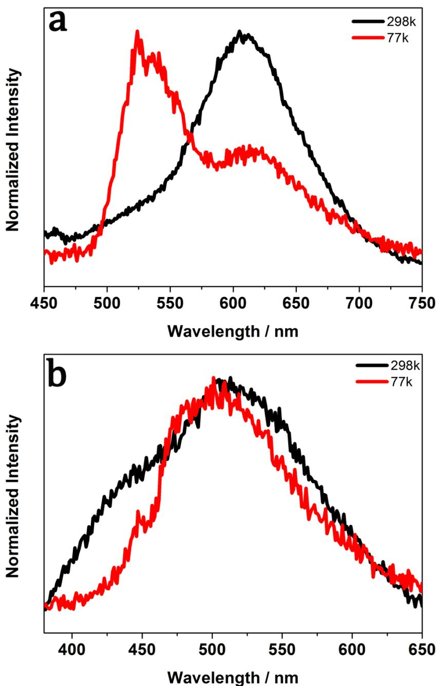
**Figure S13.** low temperature (77K) and room temperature (298K) phosphorescence spectra of a) CDs@Mn-LEV and b) CDs@Zn-CHA composites.
