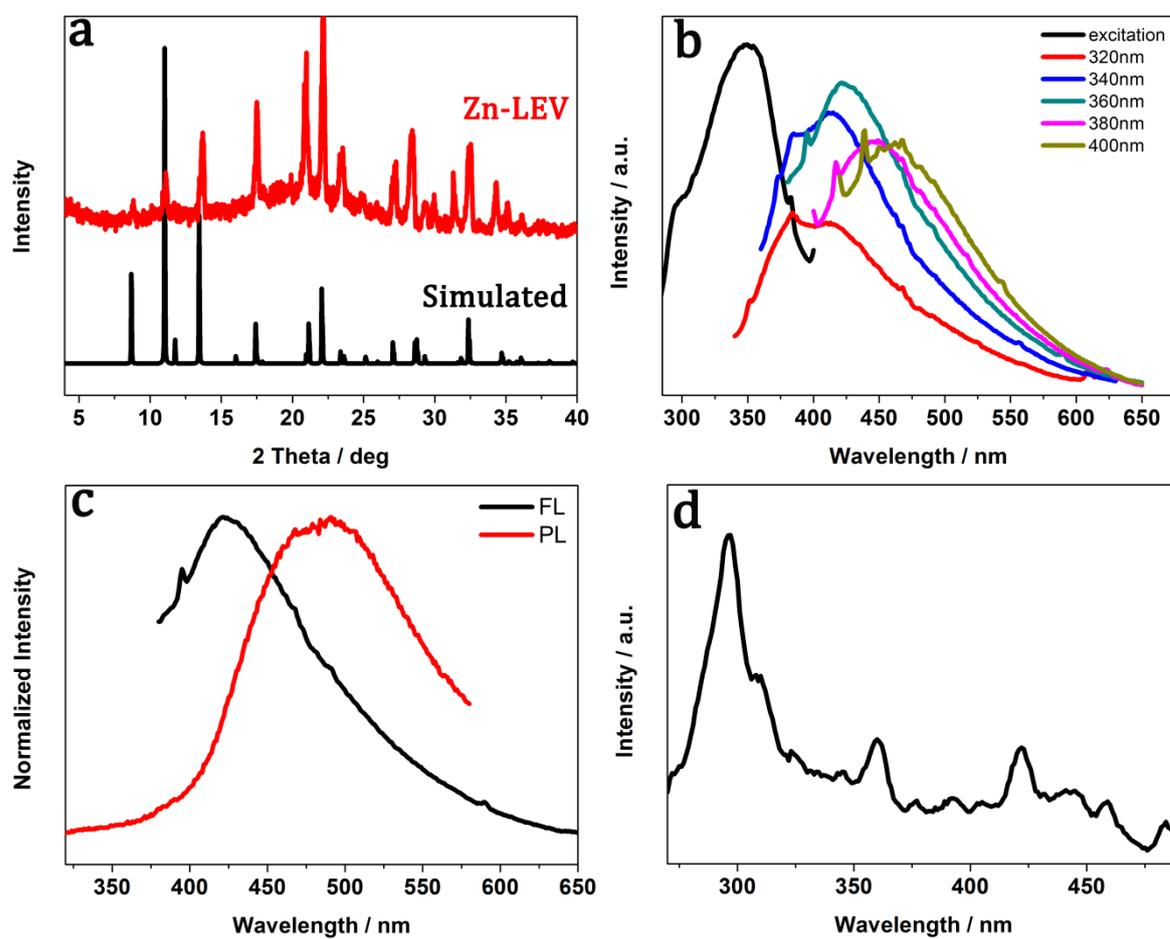
**Figure S8.** a) PXRD pattern of CDs@Zn-LEV; b) fluorescence excitation spectrum (black line) and emission spectra under different  $\lambda_{ex}$ ; c) normalized fluorescence (black line) and phosphorescence (red line) spectra of CDs@Zn-LEV; d) phosphorescent excitation spectrum of CDs@Zn-LEV.
