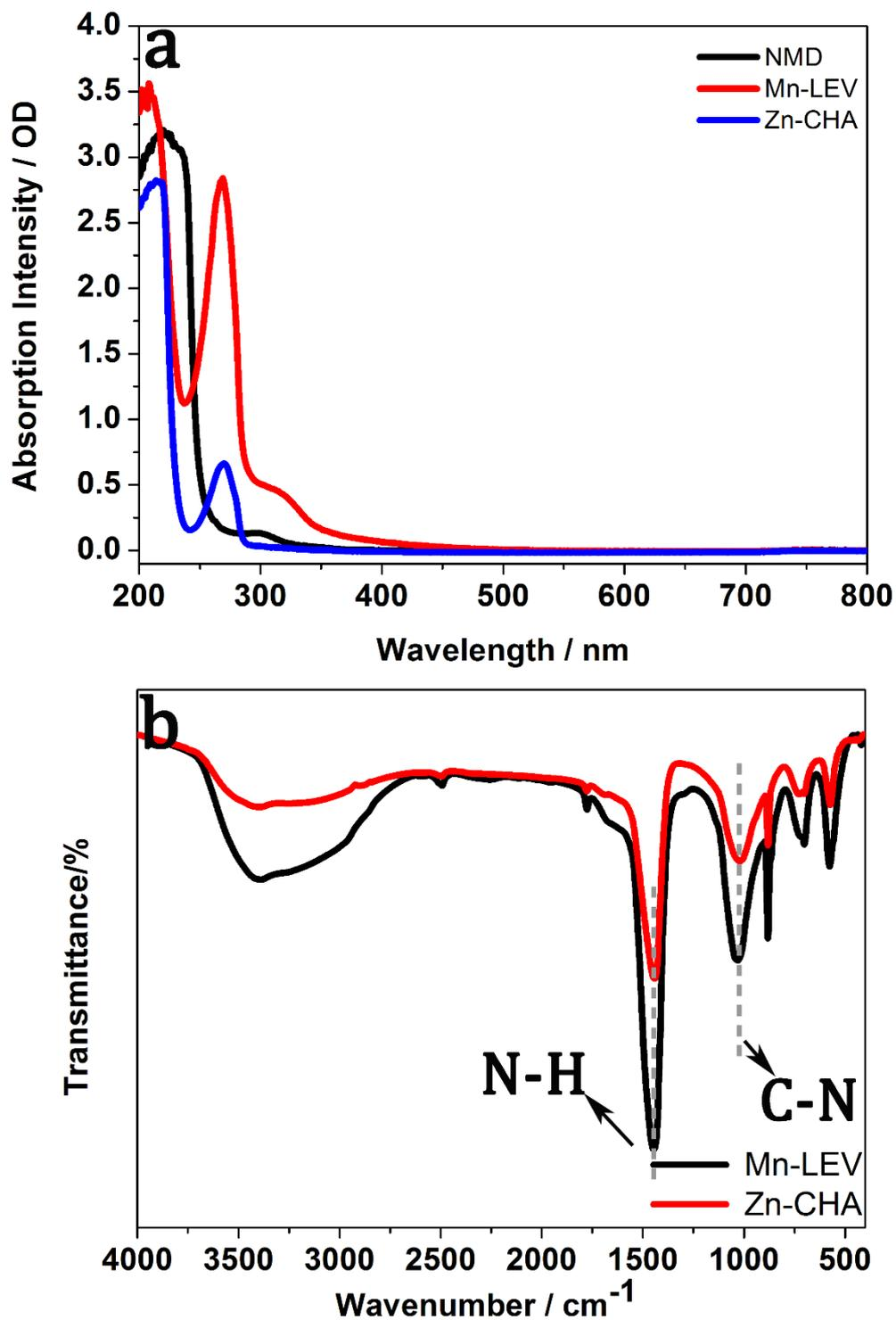
**Figure S6.** a) UV-vis absorption spectra and b) FTIR spectra of mother solutions obtained from the CDs@Mn-LEV and CDs@Zn-CHA.
