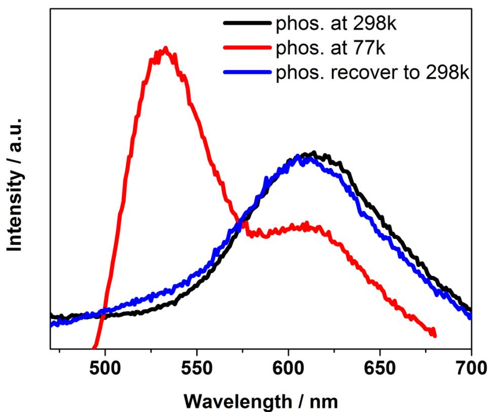
**Figure S15.** Recyclable thermal-responsive phosphorescence emission of CDs@Mn-LEV from green to red upon heating up from 77K to room temperature.
