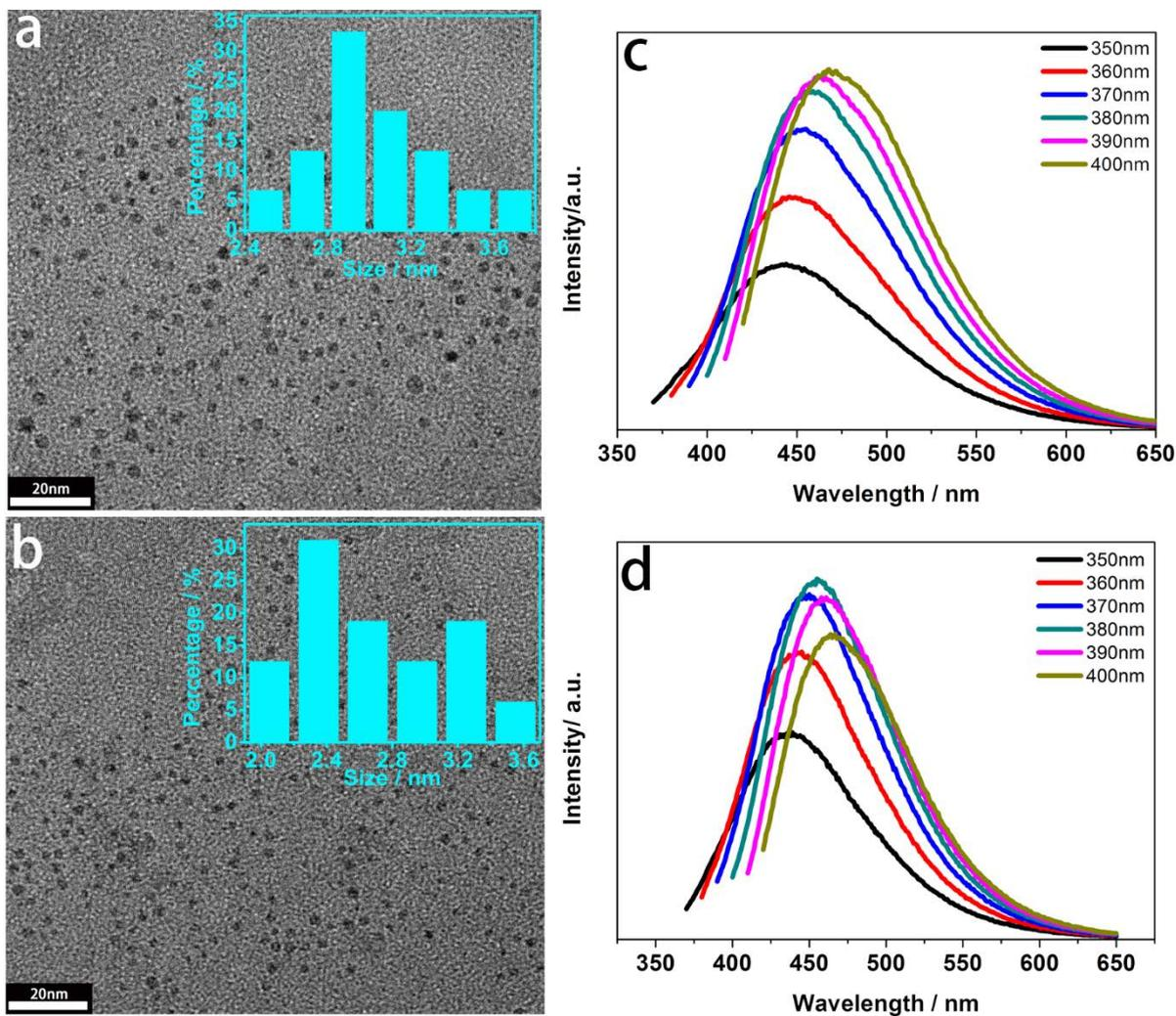
**Figure S4.** a, b) TEM images and particle diameter distributions of CDs in mother solutions of CDs@Mn-LEV and CDs@Zn-CHA; c, d) fluorescence emission spectra of mother solutions of CDs@Mn-LEV and CDs@Zn-CHA under different excitation.
