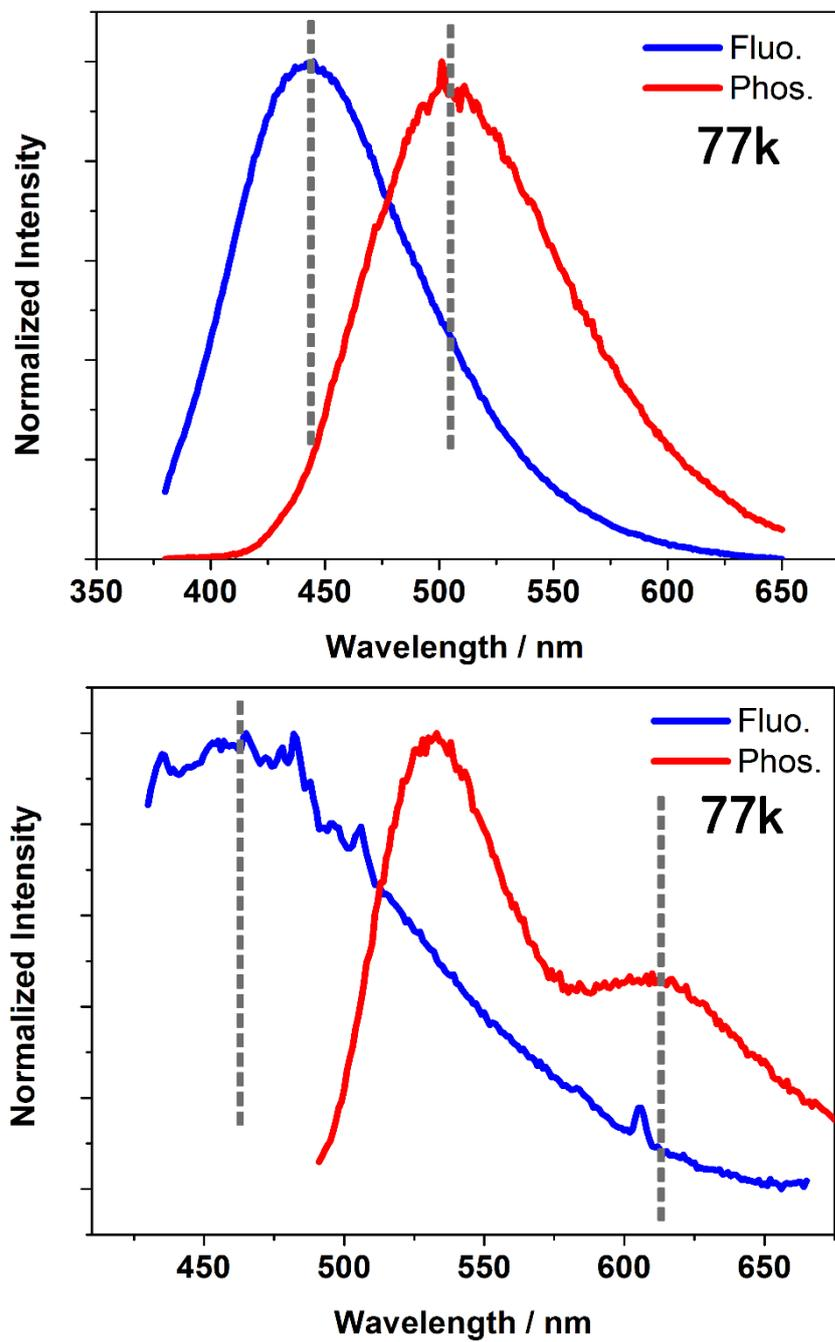
**Figure S11.** The fluorescence spectra (blue line) and phosphorescence spectra (red line) of mother solution (up) and CDs@Mn-LEV (down) excited under 360 nm at 77 K.
