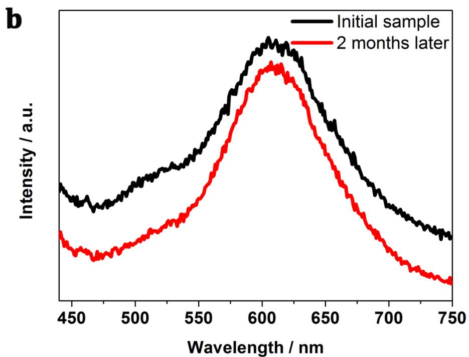
**Figure S14.** a) phosphorescence intensity ratios of CDs@Mn-LEV under UV lamp from 15 min to 180 min; b) phosphorescence emissions of CDs@Mn-LEV at the beginning and after 2 months.
