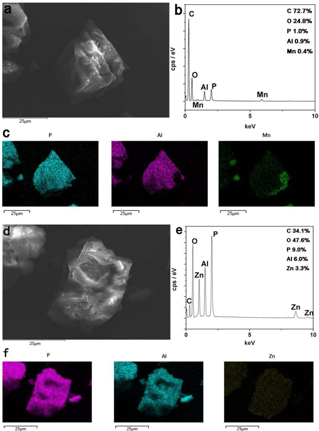
**Figure S1.** a, b, c) SEM mappings and EDS spectra of CDs@Mn-LEV; d, e, f) SEM mapping and EDS spectra of CDs@Zn-CHA.
