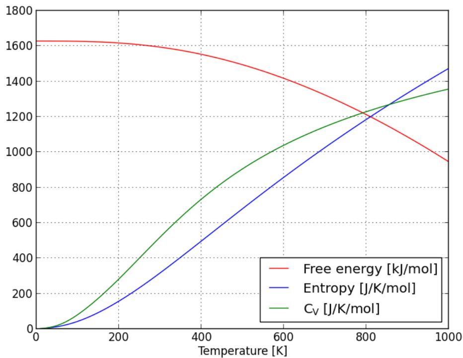
Figure S4: Thermodynamic properties for graphamine computed from the phonon density of states.
