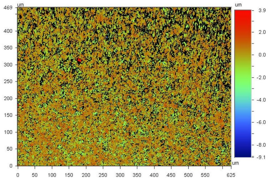
**Figure S1.** Optical profilometry of ceramic substrates. Surface profile of  $\text{Al}_2\text{O}_3$  (top) and  $\text{AlN}$  (bottom) ceramic substrates
