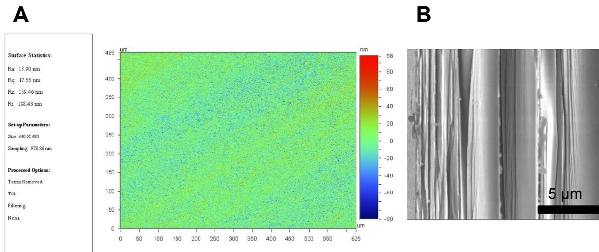
**Figure S3.** Graphitic networks on quartz. (A) Surface profile of quartz substrate. (B) SEM cross-section of graphitic networks on quartz
