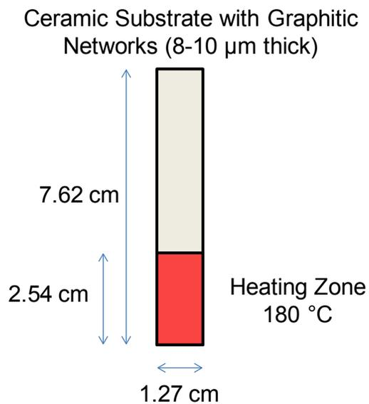
**Figure S2.** Heat transfer set-up for comparison of  $\text{Al}_2\text{O}_3/\text{AlN}$  coated with graphitic networks
