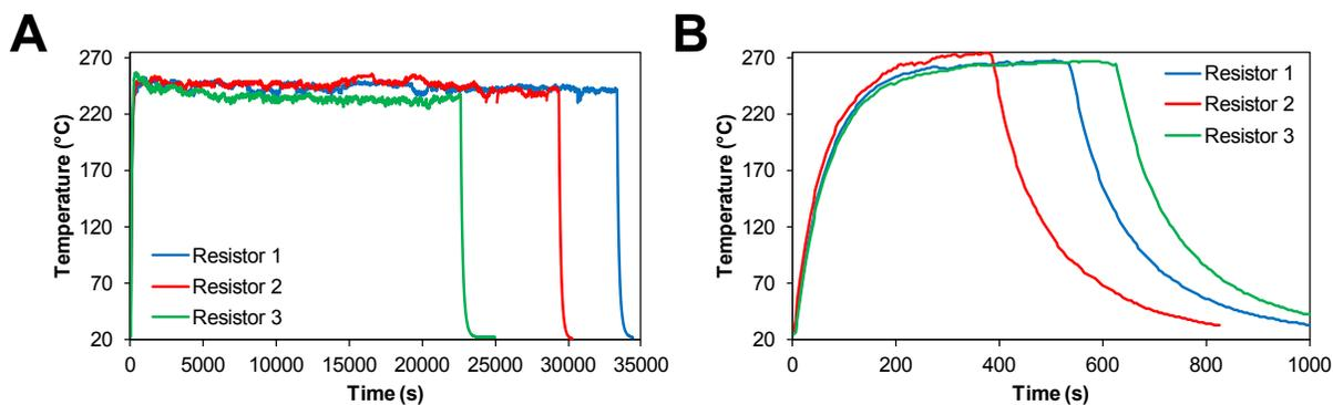
Figure S4. Resistor failure experiment front edge temperature profiles. Front edge temperature profiles of (A) coated Al<sub>2</sub>O<sub>3</sub> and (B) bare AlN DBC substrates
