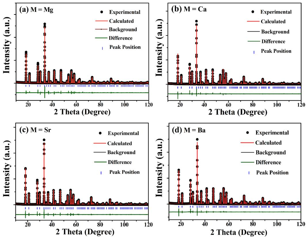
**Figure S1.** Rietveld refinement of XRD patterns of  $(\text{Lu}_2\text{M})(\text{Al}_4\text{Si})\text{O}_{12}\text{:Ce}^{3+}$  for  $\text{M}=\text{Mg}$  (a),  $\text{M}=\text{Ca}$  (b),  $\text{M}=\text{Sr}$  (c) and  $\text{M}=\text{Ba}$  (d).
