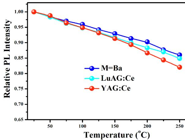
**Figure S6.** Thermal quenching properties of  $(\text{Lu}_2\text{M})(\text{Al}_4\text{Si})\text{O}_{12}:\text{Ce}^{3+}$  ( $\text{M}=\text{Ba}$ ), LuAG:Ce and YAG:Ce.
