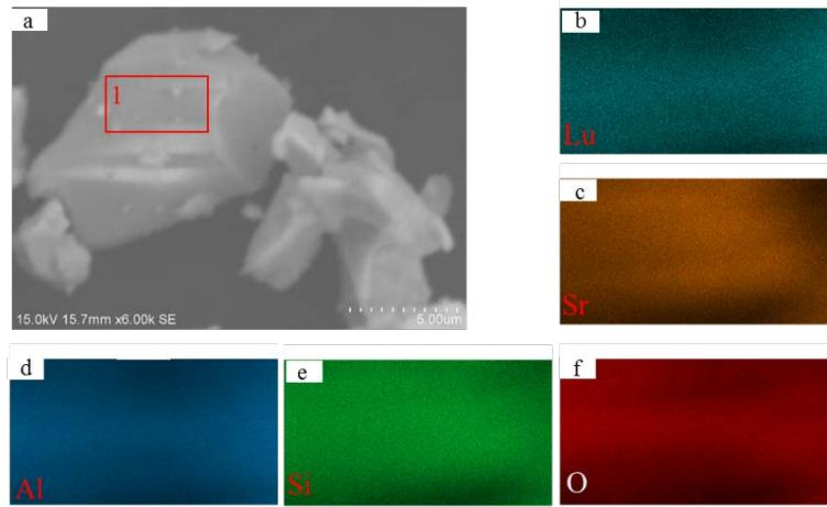
**Figure S5.** SEM image of  $(\text{Lu}_2\text{M})(\text{Al}_4\text{Si})\text{O}_{12}:\text{Ce}^{3+}$  ( $\text{M} = \text{Sr}$ ) microcrystal particles (a). And EDS elemental mapping images of Lu (b), Sr (c), Al (d), Si (e) and O (f) for the selected  $(\text{Lu}_2\text{M})(\text{Al}_4\text{Si})\text{O}_{12}:\text{Ce}^{3+}$  ( $\text{M} = \text{Sr}$ ).
