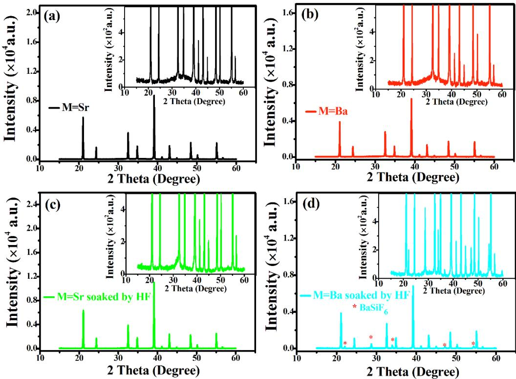
**Figure S3.** XRD patterns of  $(\text{Lu}_2\text{M})(\text{Al}_4\text{Si})\text{O}_{12}:\text{Ce}^{3+}$  before and after soakage by HF solution for  $\text{M}=\text{Sr}$  (a&c) and  $\text{Ba}$  (b&d) (the insets are the intensified ones).
