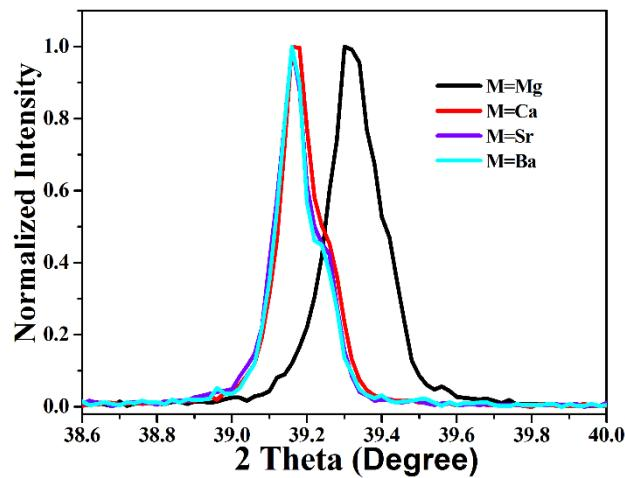
**Figure S2.** Normalized magnified XRD patterns of  $(\text{Lu}_2\text{M})(\text{Al}_4\text{Si})\text{O}_{12}\text{:Ce}^{3+}$  around  $39^\circ$ .
