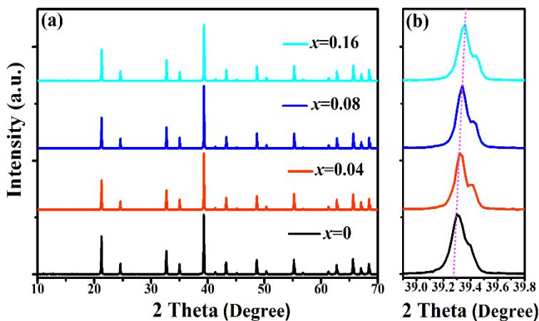
**Figure S4.** XRD patterns (a) and magnified XRD patterns around  $39^\circ$  (b) of  $\text{Lu}_3\text{Al}_5-\text{xSi}_\text{x}\text{O}_{12}:\text{Ce}^{3+}$  ( $\text{x}=0, 0.04, 0.08$  and  $0.16$ ).
