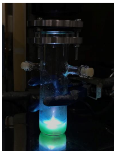
Figure S9. A photograph of the photoreactor of the dye sensitized photocatalyst Pt/TiO 2 /1 in phosphate buffer solution containing ascorbic acid (0.5 M) as the sacrificial electron donor. A 300 W Xenon lamp with a light guide was used to irradiate the photocatalyst from the top side of the photoreactor.
