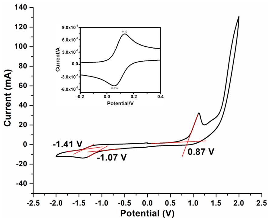
**Figure S11:** Cyclic voltammogram of PFBT-A film recorded on glassy carbon electrode with a scan rate of  $50 \text{ mV s}^{-1}$ . The inset corresponds to the cyclic voltammogram of ferrocene.
