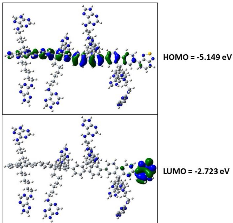
**Figure S10:** HOMO-LUMO hybrid structures of the polymer bioconjugate PFBT-A. Theoretical Band Gap =  $2.426 \text{ eV}$
