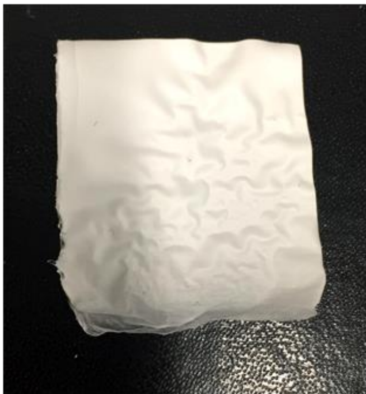
Figure S1: Electrospun nanofiber mesh that appear like tissue paper
