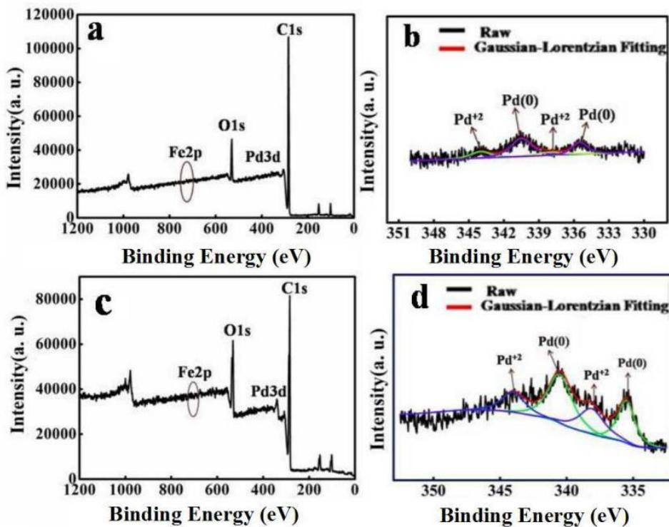
**Figure S8.** XPS spectra of (a,b)  $\text{Fe}_3\text{O}_4@\text{CFR}@ \text{PdNPs}$  and (c,d)  $\text{Fe}_3\text{O}_4@\text{CFR}@ \text{GO}@ \text{PdNPs}$  nanospheres (a,c: survey spectra, b,d: High-resolution Pd2p spectra).
