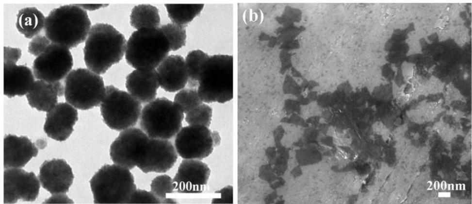
**Figure S1.** TEM images of (a) Fe<sub>3</sub>O<sub>4</sub> nanoparticles and (b) graphene oxide sheets.
