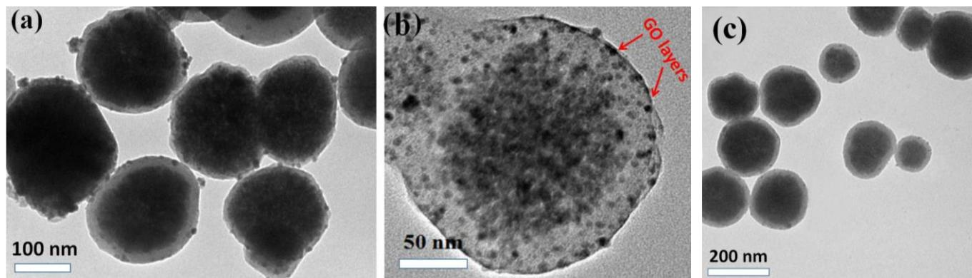
Figure S6. (a) Low-magnification and (b) High-magnification TEM images of  $\text{Fe}_3\text{O}_4@\text{CFR}@\text{GO}@ \text{PdNPs}$  nanospheres. (c). Low-magnification TEM image of  $\text{Fe}_3\text{O}_4@\text{CFR}@ \text{PdNPs}$  nanospheres.
