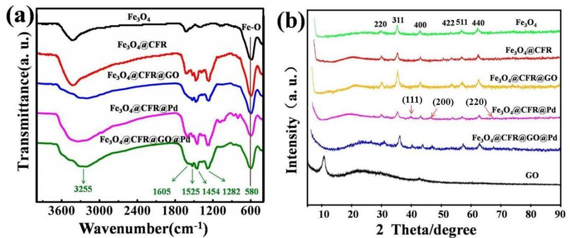
**Figure S9.** (a) FTIR and (b) XRD spectra of different samples.
