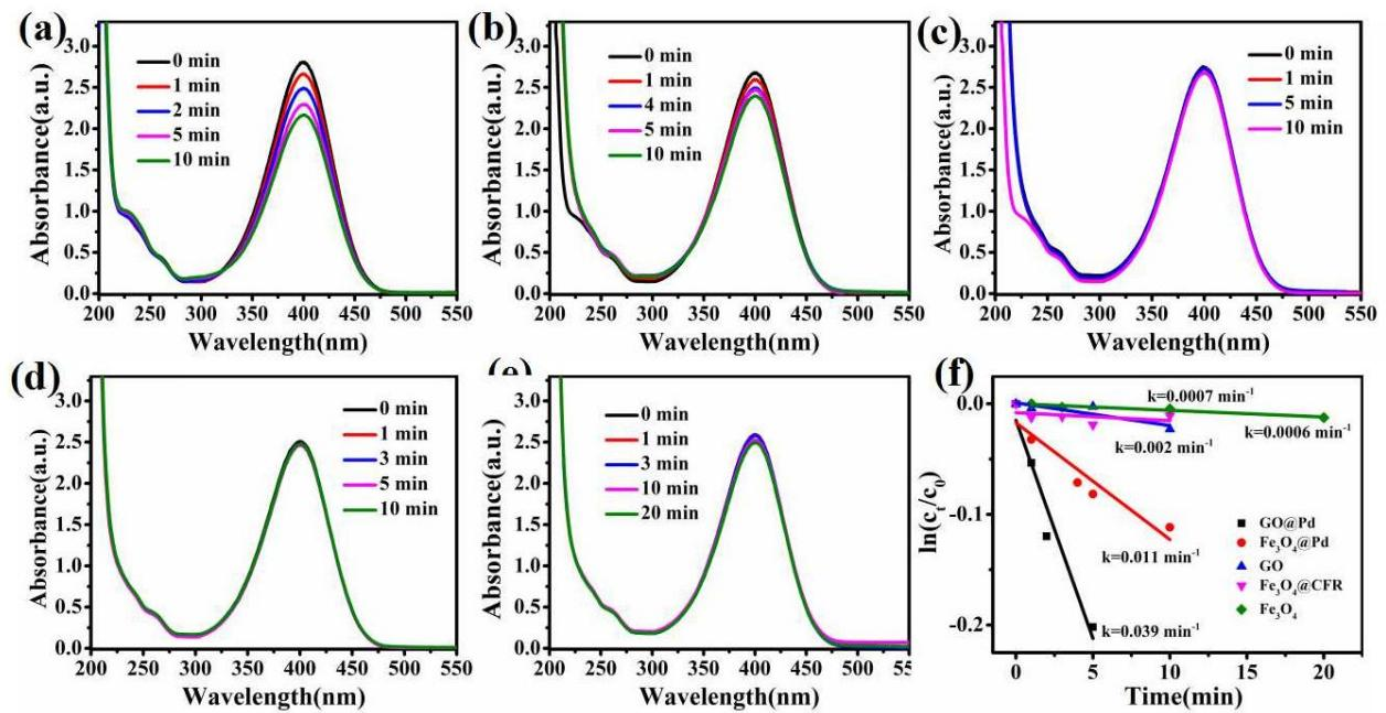
**Figure S11.** Successive reduction of *p*-NP using (a) GO@Pd, (b)  $\text{Fe}_3\text{O}_4@\text{Pd}$ , (c) GO, (d)  $\text{Fe}_3\text{O}_4@\text{CFR}$ , (e)  $\text{Fe}_3\text{O}_4$  and (f) Plots of  $\ln(c_t/c_0)$  vs. reaction time ( $t$ ) for different control catalysts (0.05 mg  $\text{mL}^{-1}$  catalyst, 2.0 mL of 0.16 mM *p*-NP and 1.0 mL of 0.2 M  $\text{NaBH}_4$  were used for the reduction of *p*-NP).
