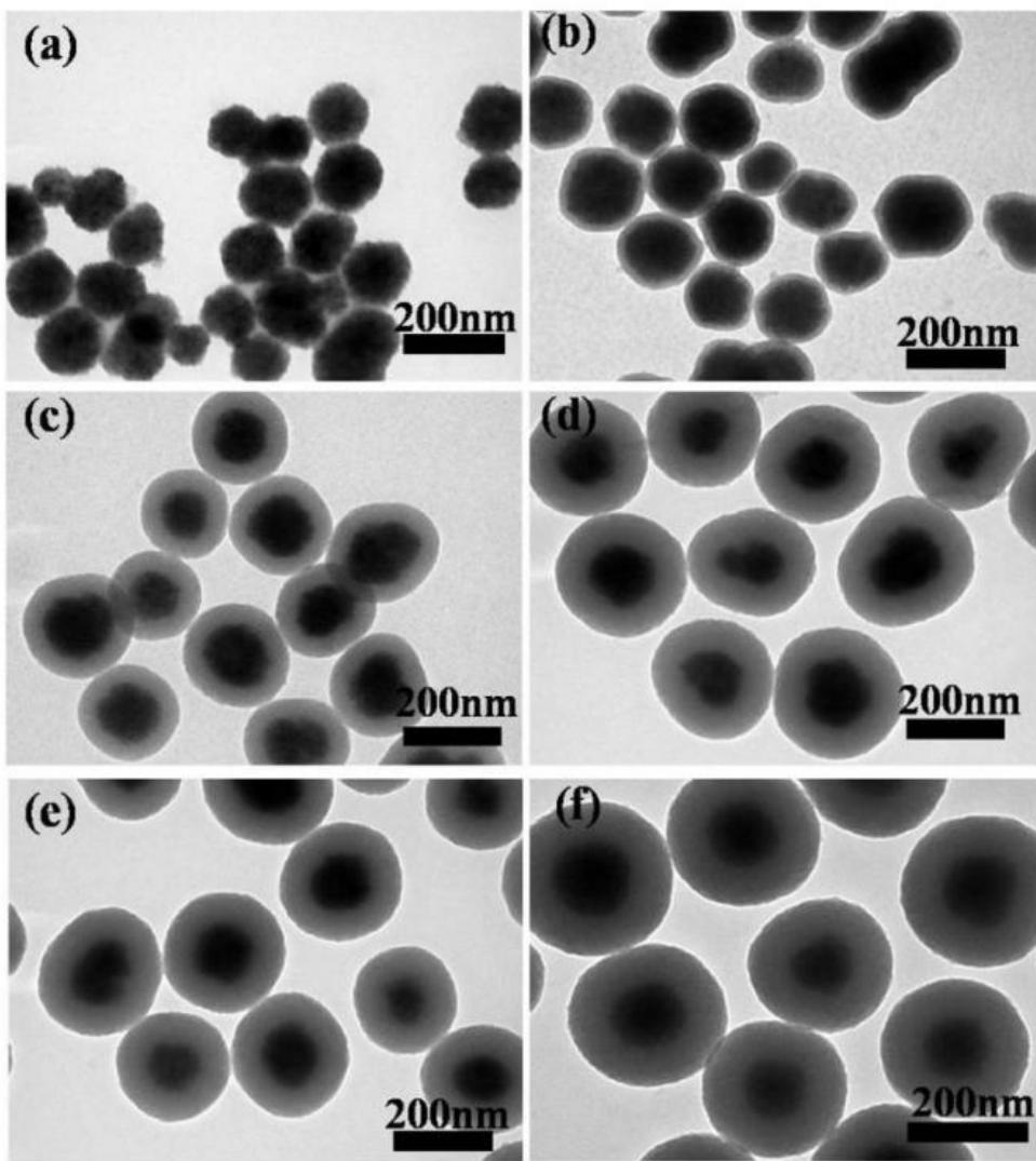
**Figure S4.** TEM images of  $\text{Fe}_3\text{O}_4@\text{CFR}$  core-shell nanospheres prepared with different reaction temperatures: (a) 80 °C, (b) 100 °C, (c) 120 °C, (d) 140 °C, (e) 160 °C, and (f) 180 °C. Reaction conditions: formaldehyde solution 0.14 mL, catechol 0.1 g,  $\text{Fe}_3\text{O}_4$  15.0 mg, water 20 mL, ammonia solution 0.075 mL, heating time 100 min.
