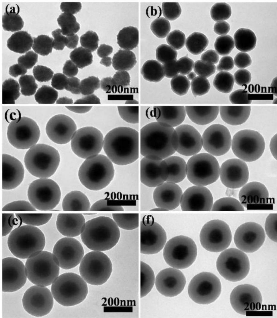
**Figure S5.** TEM images of the  $\text{Fe}_3\text{O}_4@\text{CFR}$  core-shell nanospheres prepared with different reaction times:
