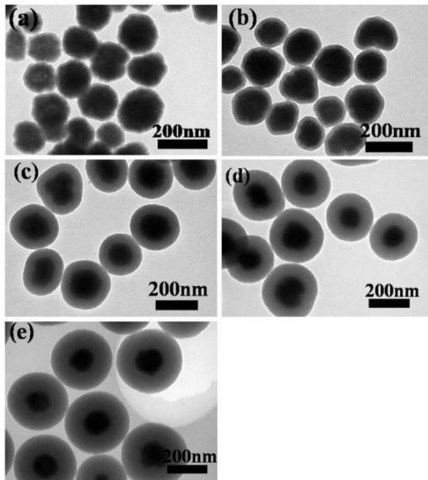
**Figure S3.** TEM images of  $\text{Fe}_3\text{O}_4@\text{CFR}$  core-shell nanospheres prepared with different amounts of formaldehyde solution: (a) 0.01 mL, (b) 0.035 mL, (c) 0.07 mL, (d) 0.105 mL, and (e) 0.14 mL. Reaction conditions: catechol 0.1 g,  $\text{Fe}_3\text{O}_4$  15.0 mg, water 20 mL, ammonia solution 0.075 mL, heating time 100 min, and reaction temperature 160 °C.
