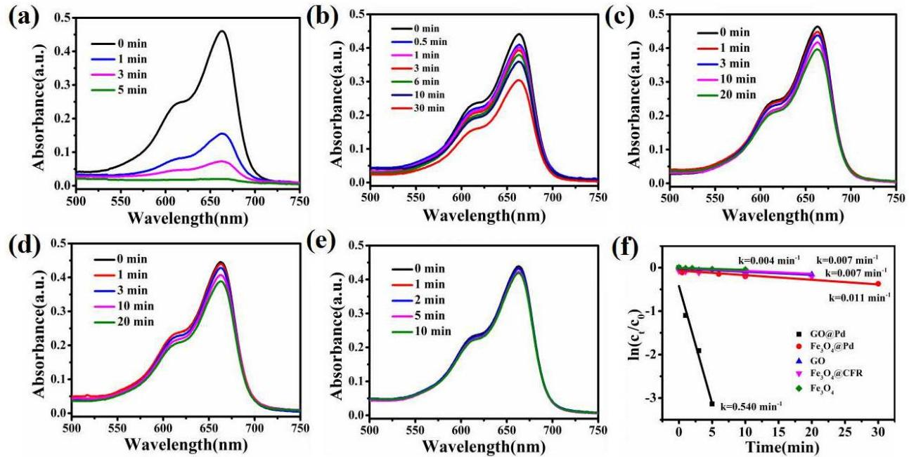
**Figure S10.** Successive reduction reaction of MB using catalysts (20  $\mu\text{L}$ ): (a) GO@Pd, (b)  $\text{Fe}_3\text{O}_4@\text{Pd}$ , (c) GO, (d)  $\text{Fe}_3\text{O}_4@\text{CFR}$ , (e)  $\text{Fe}_3\text{O}_4$  and (f) Plots of  $\ln(c_t/c_0)$  vs. reaction time ( $t$ ) for different control catalysts (0.05 mg  $\text{mL}^{-1}$  catalyst, 2.0 mL of 5 mg  $\text{L}^{-1}$  MB and 1.0 mL of 0.5 M  $\text{NaBH}_4$  were used for the reduction of MB).
