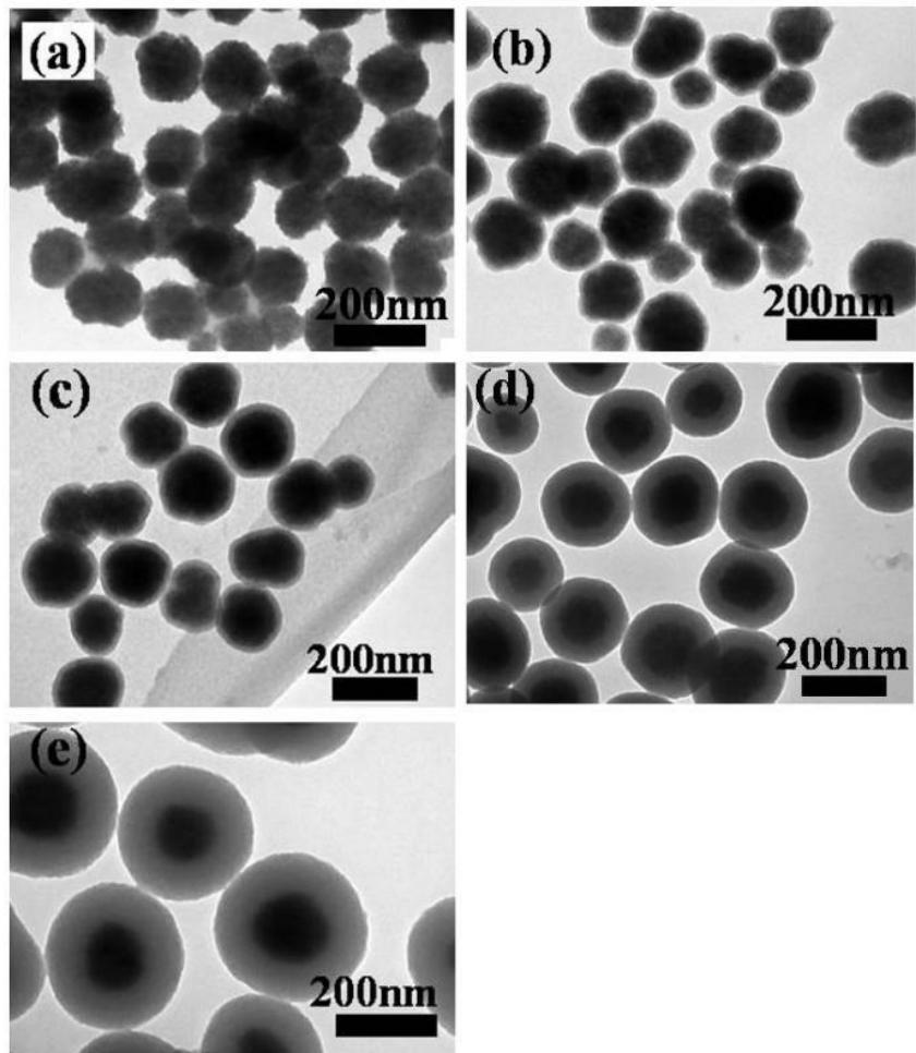
**Figure S2.** TEM images of  $\text{Fe}_3\text{O}_4@\text{CFR}$  core-shell nanospheres obtained from different amounts of catechol: (a) 0.01 g, (b) 0.02 g, (c) 0.04 g, (d) 0.08 g, (e) 0.16 g. Reaction conditions: formaldehyde solution 0.07 mL,  $\text{Fe}_3\text{O}_4$  15.0 mg, water 20 mL, ammonia solution 0.075 mL, heating time 100 min, and reaction temperature 160 °C.
