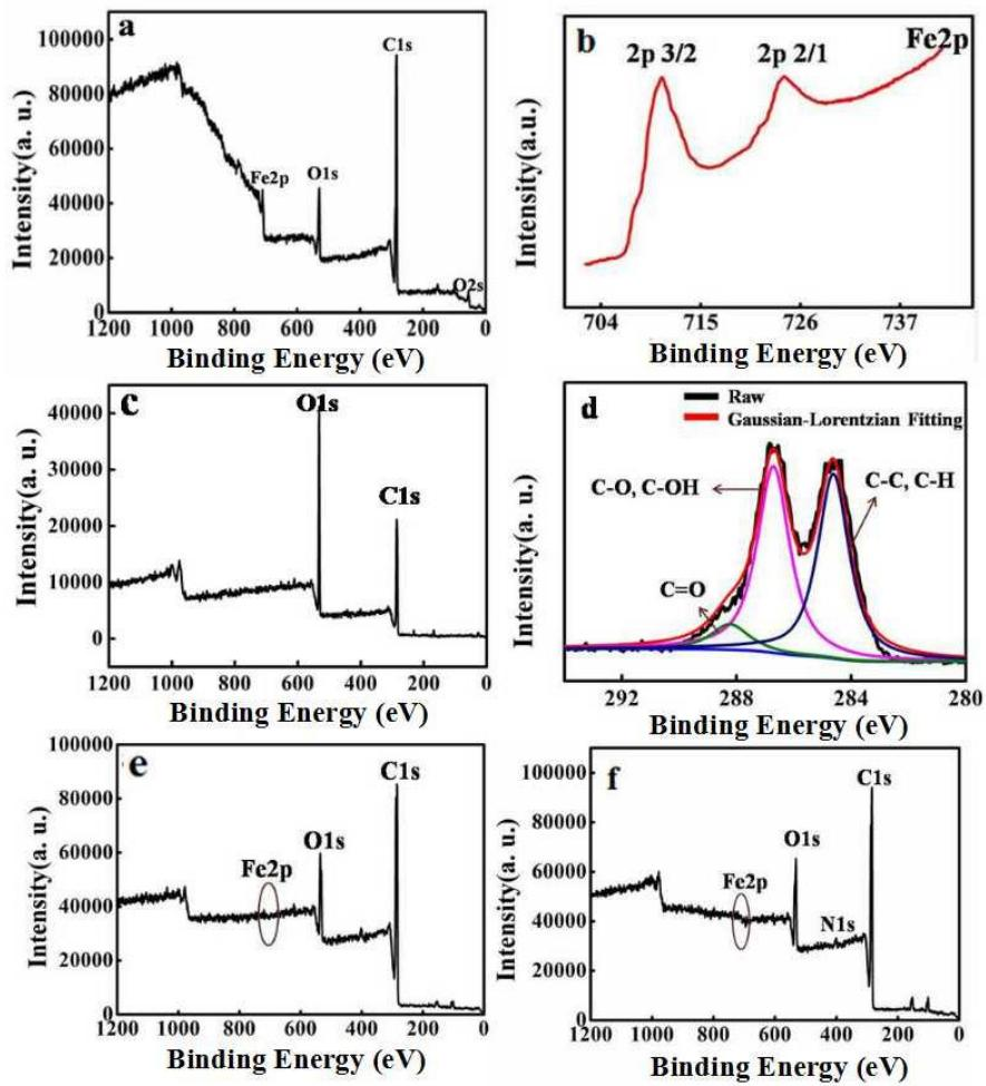
**Figure S7.** XPS survey spectra of (a)  $\text{Fe}_3\text{O}_4$  NPs, (c) GO, (e)  $\text{Fe}_3\text{O}_4@\text{CFR}$  and (f)  $\text{Fe}_3\text{O}_4@\text{CFR}@GO$
