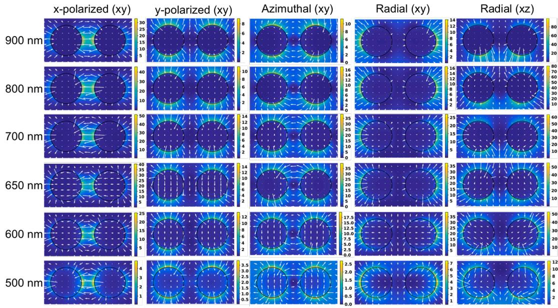
**Figure S4. Near field intensity distribution for x-polarized, y-polarized, azimuthally and radially polarized light.** The simulated AuNP diameter is 100 nm with 40 nm gap distance. The 1<sup>st</sup> to 4<sup>th</sup> columns are the xy plane (focal plane) and the 5<sup>th</sup> column is the xz plane. Six wavelengths of 900 nm, 800 nm, 700 nm, 650 nm, 600 nm, and 500 nm were selected for each polarization.
