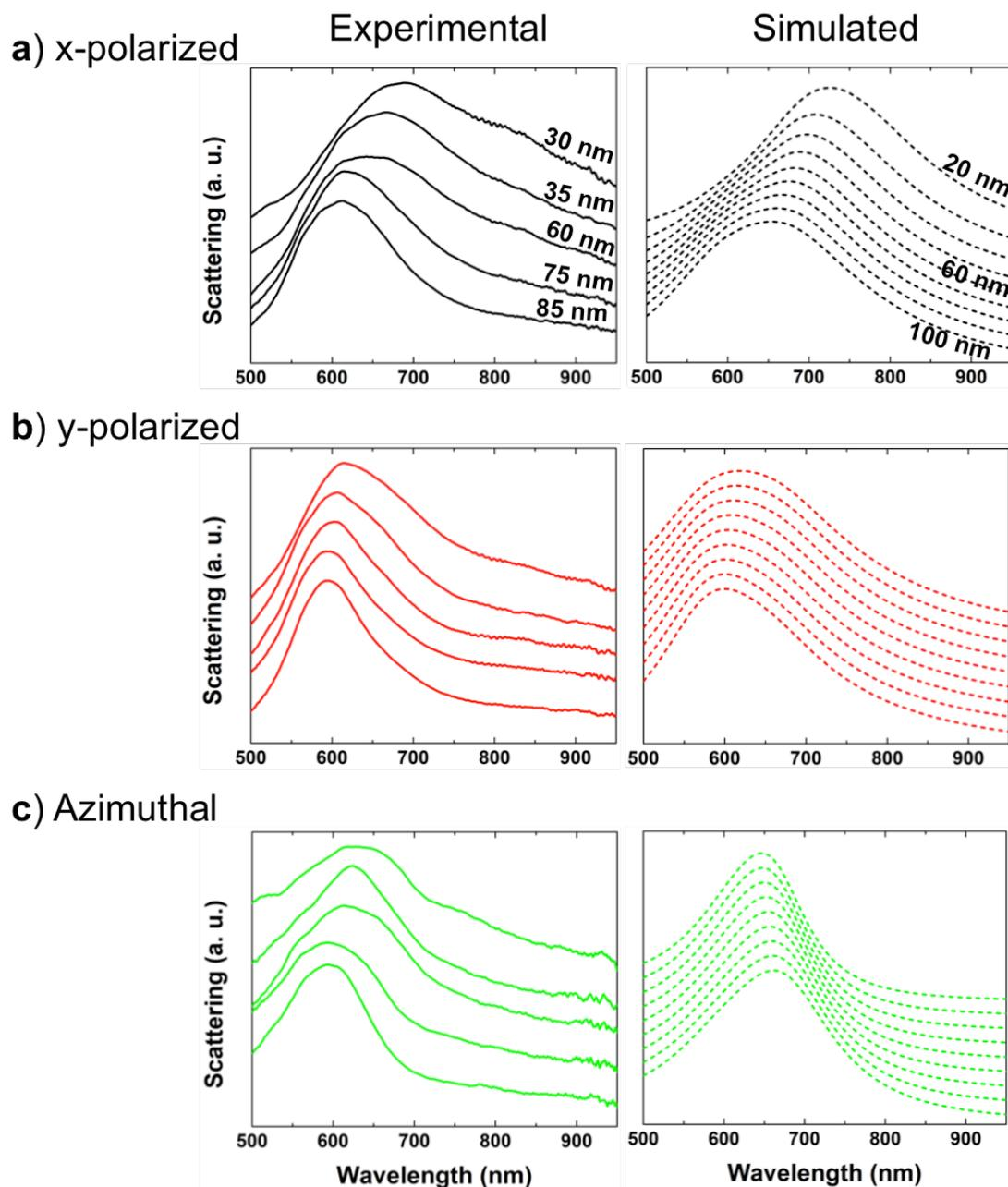
**Figure S7. Experimental and simulated spectra of AuNP dimers with different gaps excited by (a) x-polarized, (b) y-polarized, and (c) azimuthally polarized light.** From top to bottom, the gaps are 30 nm, 35 nm, 60 nm, 75 nm, and 85 nm in the experimental spectra, and are from 20 to 100 nm, with step size of 10 nm in the simulated spectra. The experimental and simulated spectra are in good agreement.
