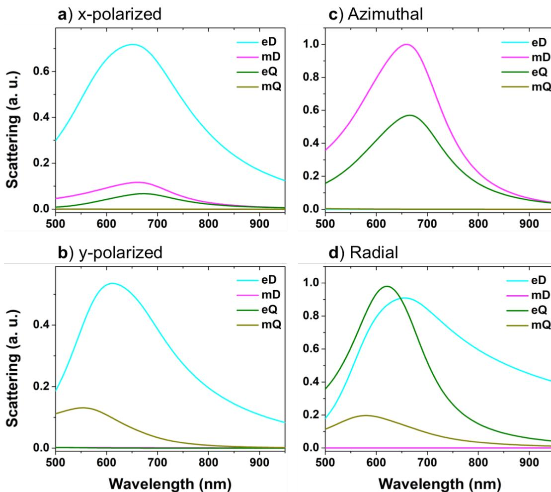
**Figure S8.** Expansion of the FDTD scattering amplitudes into electric and magnetic multipolar modes for a 100 nm gap AuNP dimer. The simulated results are for (a) x-polarized, (b) y-polarized, (c) azimuthally polarized, and (d) radially polarized beam excitation. Compared to the 40 nm gap AuNP dimer (Figure 3d), the scattering spectra associated with the eD and eQ modes are more overlapped for radial beam illumination, resulting in more symmetric spectra (Figure 7c, bottom spectra).
