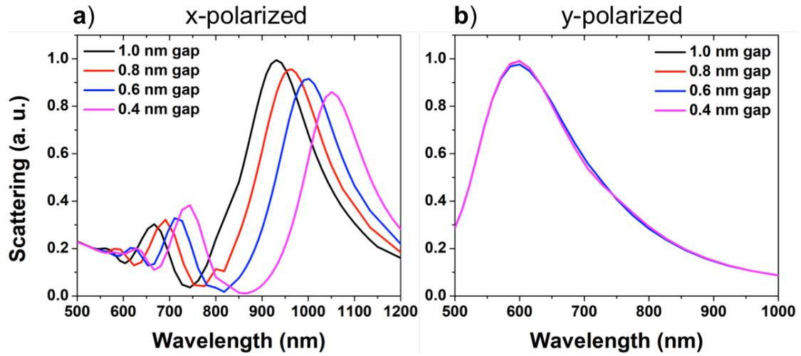
**Figure S2. Simulated scattering spectra excited by linearly polarized beams.** (a) The scattering spectra are obtained for polarization of the incident field parallel to the dimer axis (x-polarized), and (b) scattering spectra obtained for illuminating beams linearly polarized perpendicular to the dimer axis (y-polarized).
