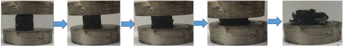
Figure S12. Digital photographs of KGA-3 compression test with a carbonization temperature of 800 °C.
