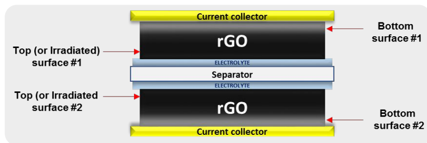
Figure S1. Structure of an rGO supercapacitor.
