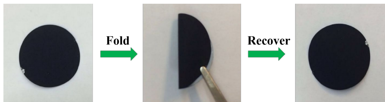
Figure S1. Optical image of Co(OH) 2 @CNF/KB-modified separator with the folding test.
