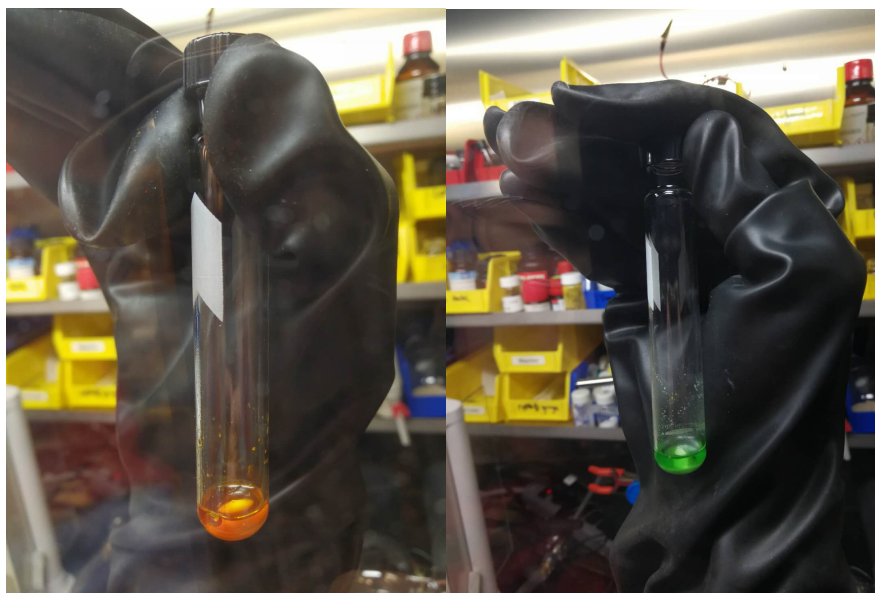
Figure S1. Pre-activation of the catalyst. Left: before pre-activation, showing red color from catalyst. Right: after pre-activation, showing green color of the Ti III active catalyst.
