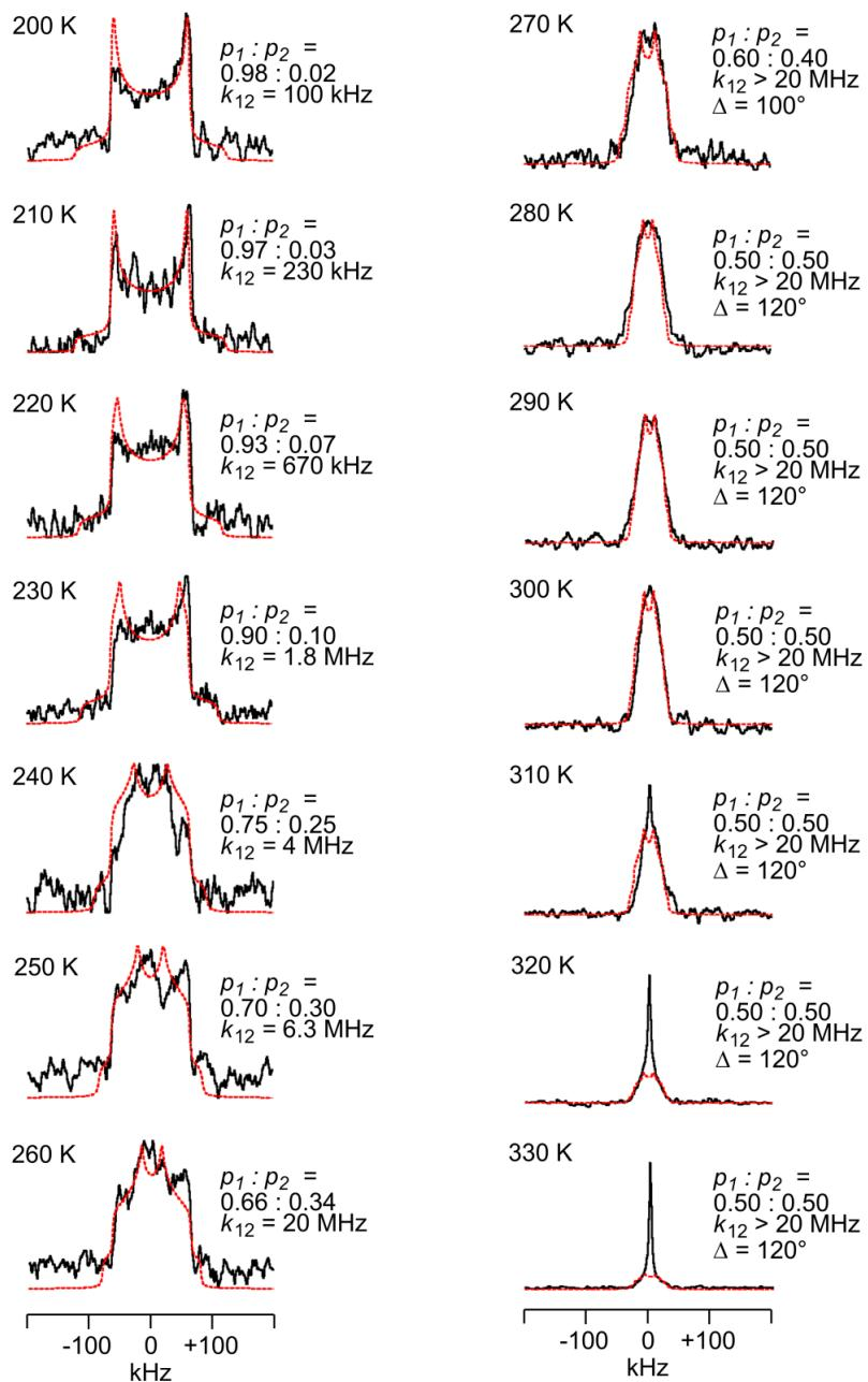
**Figure S39.** Temperature dependence of solid-state  $^2\text{H}$  NMR spectra of C16-d<sub>2</sub> [solid black line: observed spectra; dotted red line: spectra simulated by assuming  $180^\circ$  flipping with designated exchange rate constants,  $k$ , and population ratio between two sites,  $p_1:p_2$ , and degree of angular displacement ( $\Delta$ )].
