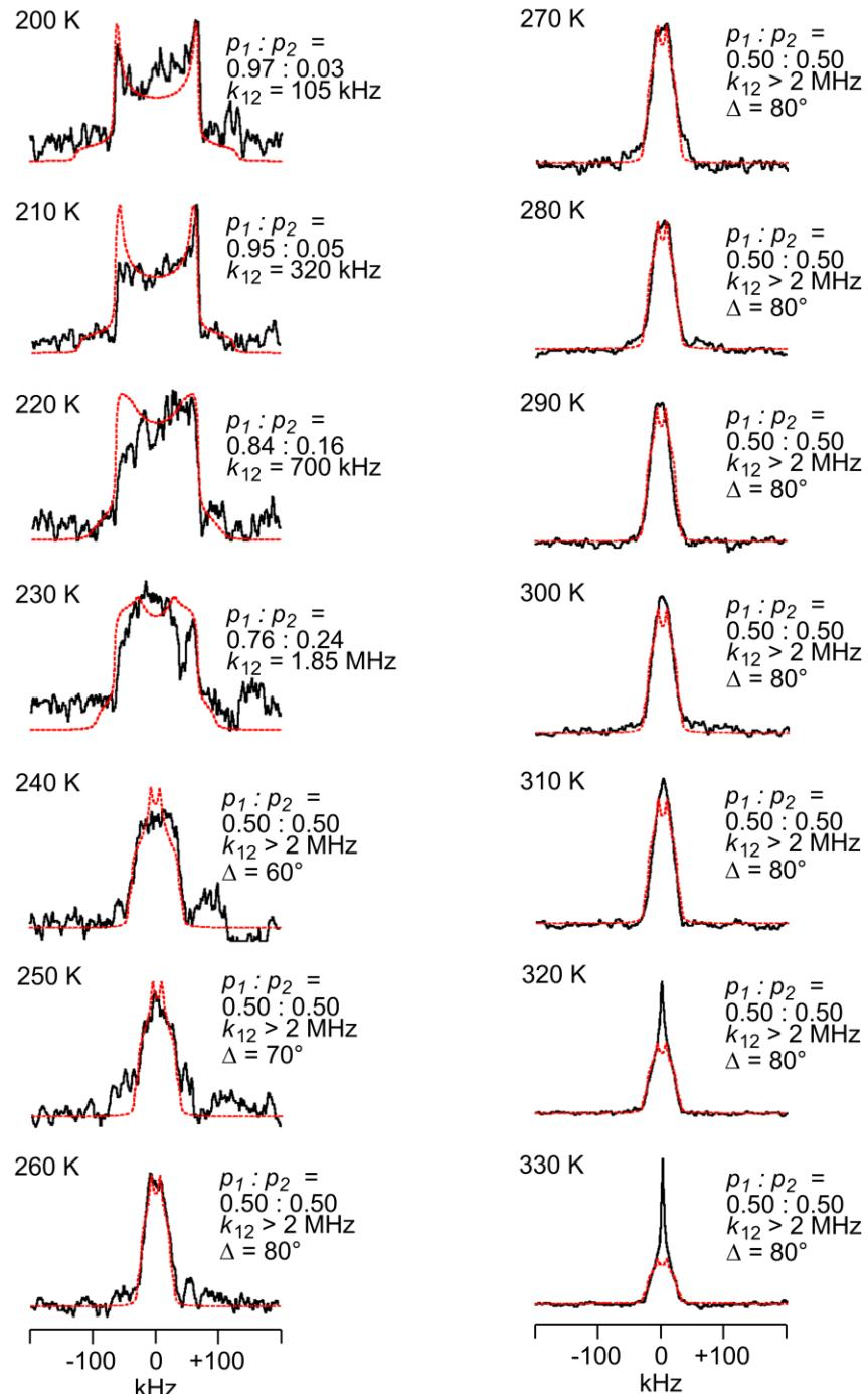
**Figure S40.** Temperature dependence of solid-state  $^2\text{H}$  NMR spectra of C17-d<sub>2</sub> [solid black line: observed spectra; dotted red line: spectra simulated by assuming 180° flipping with designated exchange rate constants,  $k$ , and population ratio between two sites,  $p_1:p_2$ , and degree of angular displacement ( $\Delta$ )].
