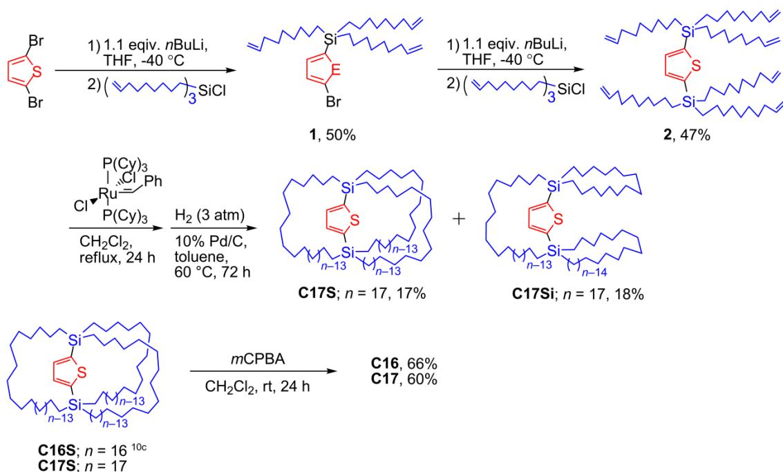
**Scheme S1.** Synthesis of molecular gyrotops **C16** and **C17**.
