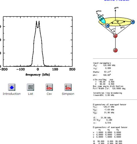
**Figure S41.** Representative displays of  $^2\text{H}$  NMR spectral simulation: (a) an example for 2-site exchange at certain rate (**C16-d<sub>2</sub>** at 200 K); (b) an example for 2-site exchange at fast rate limit (**C16-d<sub>2</sub>** at 280 K).
